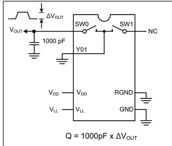
**FIGURE 3-11:** Charge Injection.
