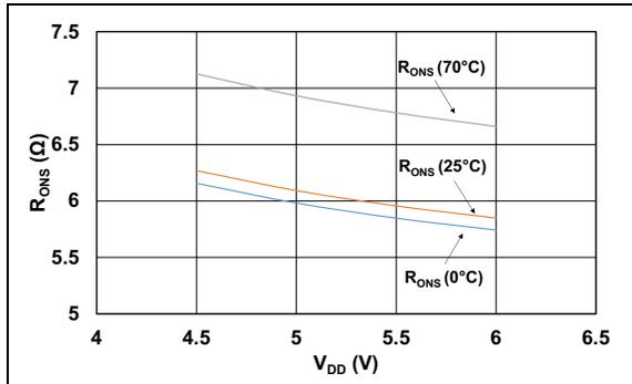
**FIGURE 4-1:**  $R_{ONS}$  at 5 mA vs.  $V_{DD}$ .
