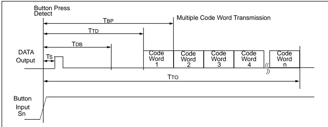
**TABLE 8-3: POWER-UP AND TRANSMIT TIMING<sup>(2)</sup>**
