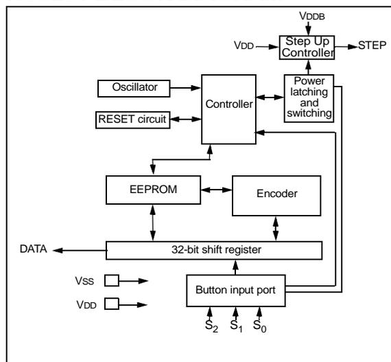
The HCS201 combines a 32-bit hopping code, generated by a nonlinear encryption algorithm, with a 28-bit serial number and 6 information bits to create a 66-bit code word. The code word length eliminates the threat of code scanning and the code hopping mechanism makes each transmission unique, thus rendering code capture and resend schemes useless.
