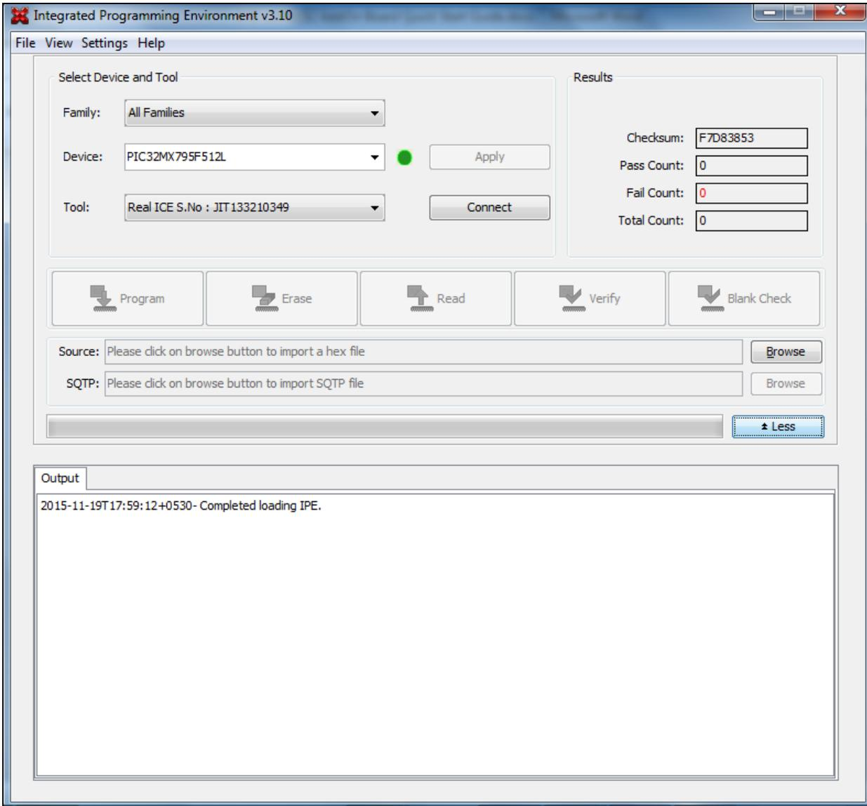
4. Select the corresponding device from the “Device” drop-down box and then click **Apply**.
