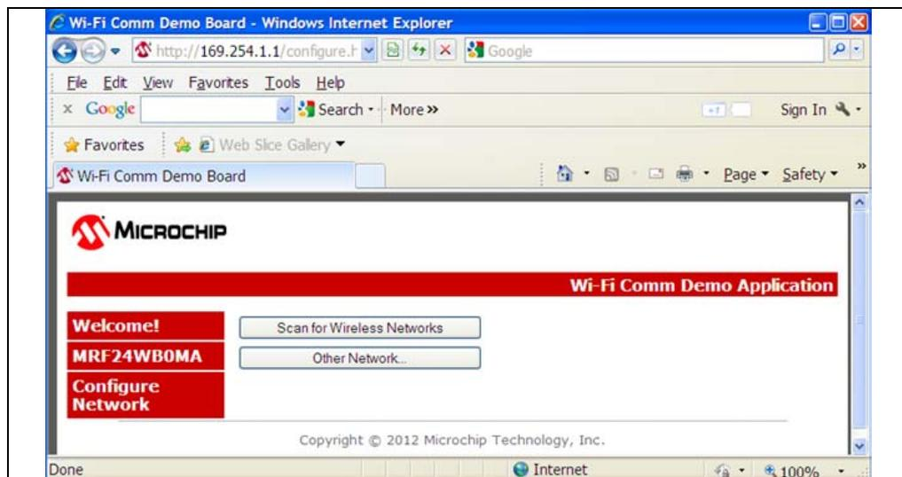
5. To connect the Wi-Fi Comm Demo board to an existing network: Click **Scan for Wireless Networks** on the `configure.htm` web page.
