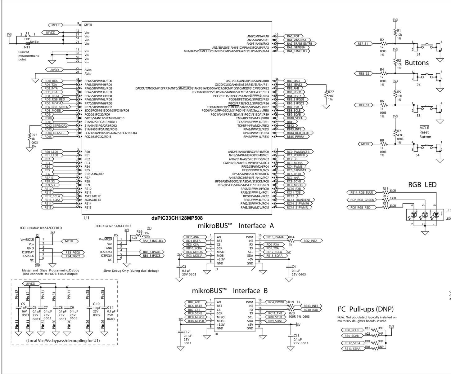
FIGURE A-3: dsPIC33CH CURIOSITY BOARD LAYOUT SCHEMATIC REV. 1.0 (SHEET THREE OF FOUR)
