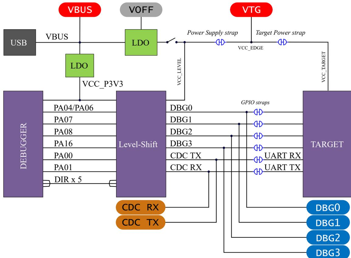
Figure 7-6. On-Board Debugger Connection Cut Straps
