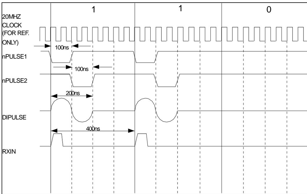
Figure 5.9 - Dipulse Waveform for Data of 1-1-0
