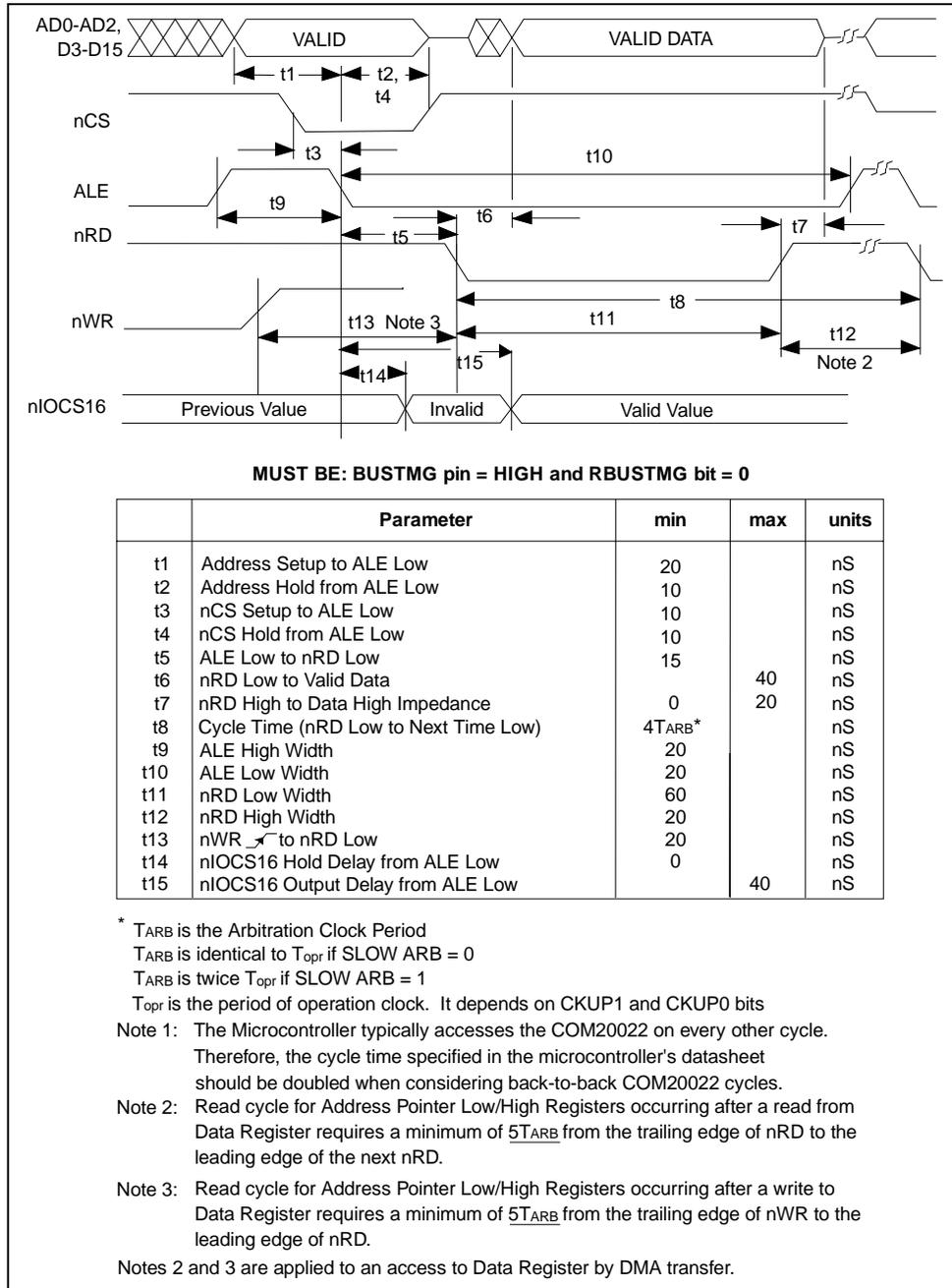
**Figure 8.2 - Multiplexed Bus, 80XX-Like Control Signals; Read Cycle**
