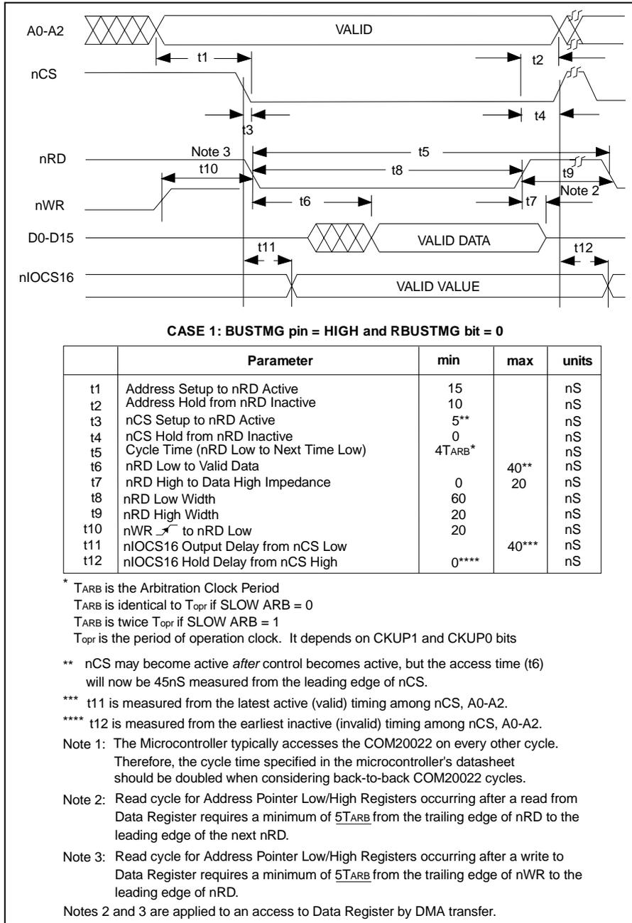
Figure 8.5 - Non-Multiplexed Bus, 80XX-Like Control Signals; Read Cycle
