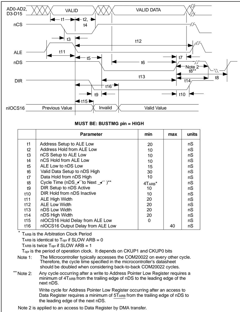
**Figure 8.3 - Multiplexed Bus, 68XX-Like Control Signals Write Cycle**
