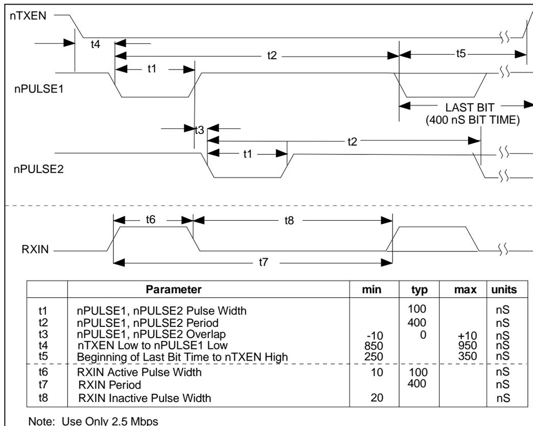
**Figure 8.13 - Normal Mode Transmit or Receive Timing**
