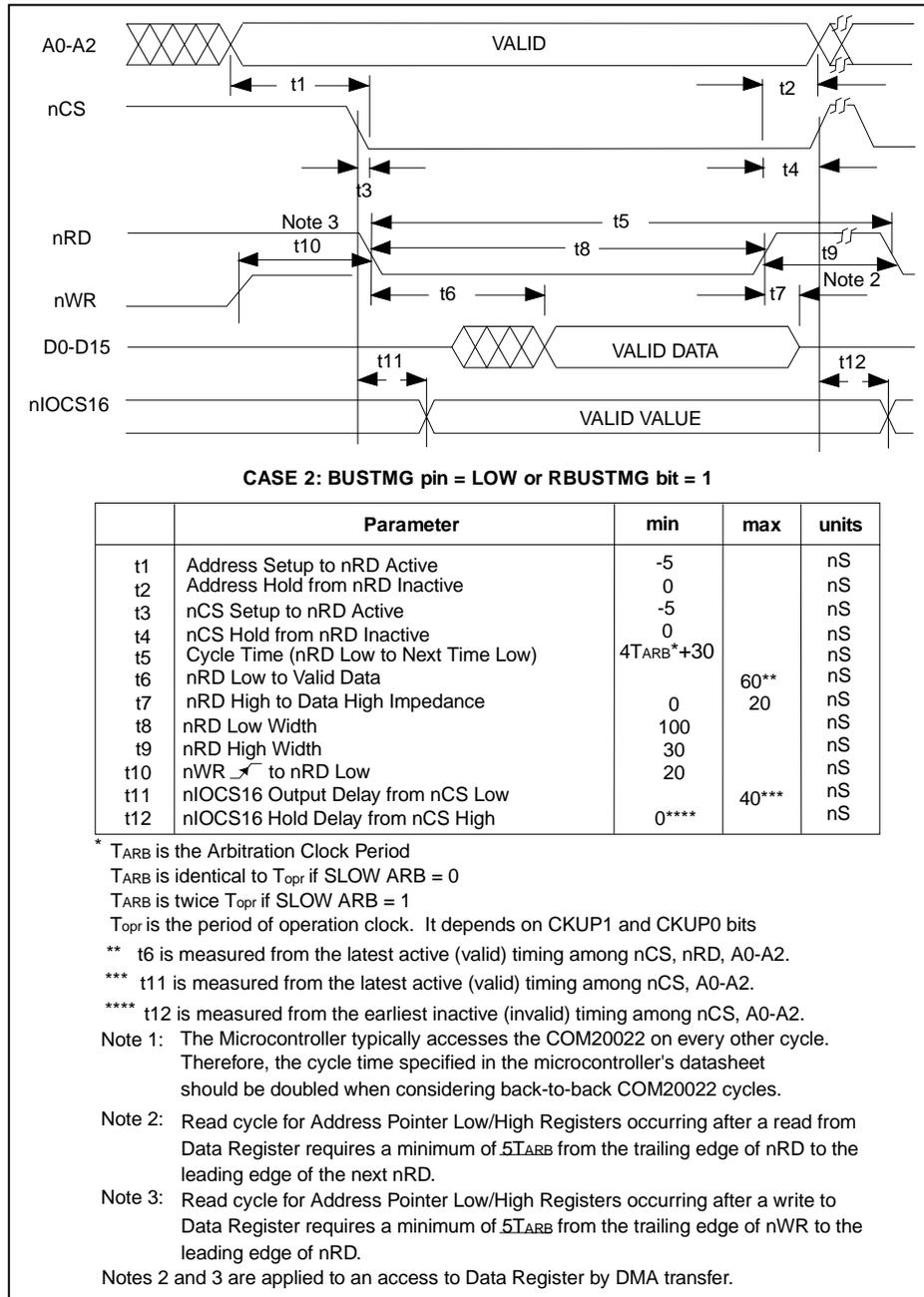
**Figure 8.6 - Non-Multiplexed Bus, 80XX-Like Control Signals; Read Cycle**
