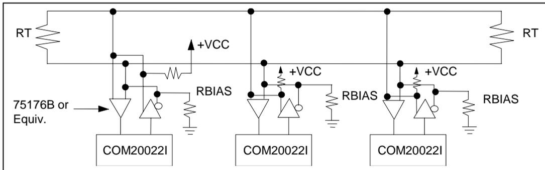
Figure 5.8 - COM20022I Network Using RS-485 Differential Transceivers
