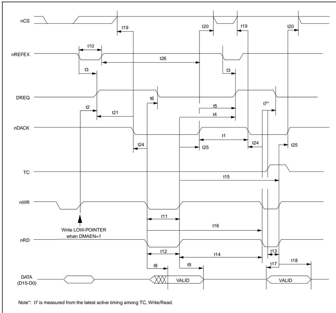
**Figure 8.17 - DMA Timing (Intel Mode 80XX)**
