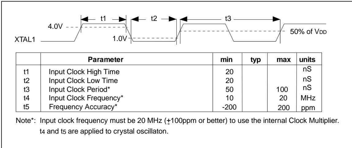
Figure 8.15 - TTL Input Timing on XTAL1 Pin
