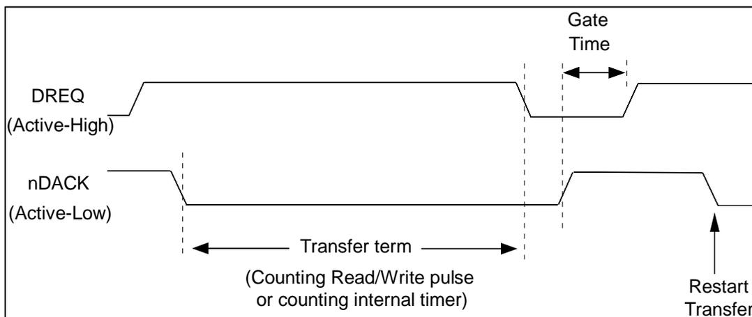
**Figure 5.4 - Programmable Burst Mode DMA Transfer (Rough Timing)**
