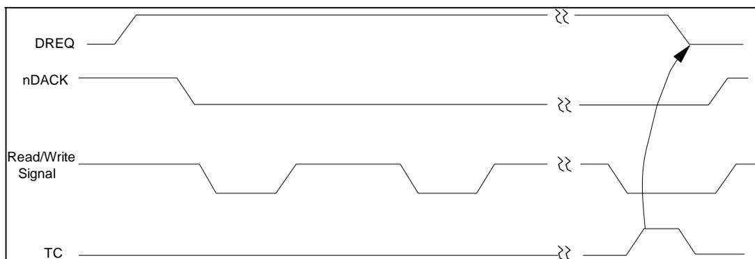
**Figure 5.6 - Burst Mode DMA Data Transfer Rough Timing**
