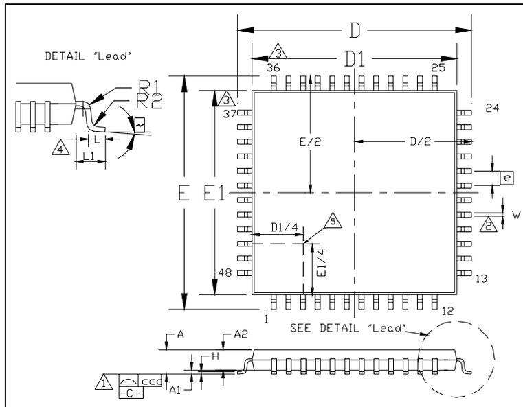
Figure 9.1 - COM20022I 48 Pin TQFP Package Outline
