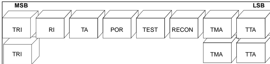
**Figure 6.4 - Command Chaining Status Register Queue**
