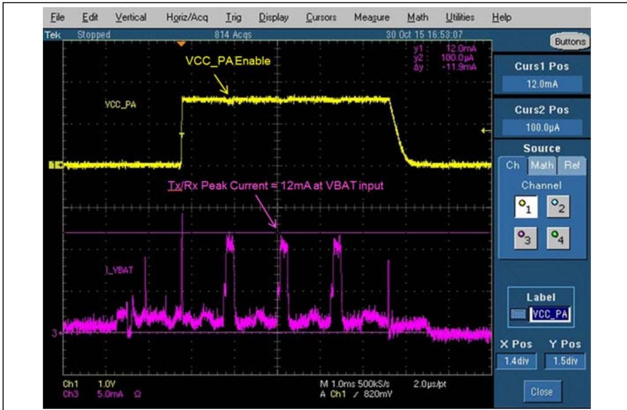
Figure 5-2 illustrates the oscilloscope screen, captured when the auto operation and Low Power mode is active on the BM70/71 module. Refer to the “*BM70/71 Bluetooth® Low Energy Module User’s Guide*” (DS50002542) for more details on the auto operation.
