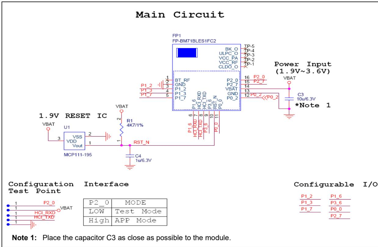
**FIGURE 2-8: BM71BLES1FC2 REFERENCE CIRCUIT - OPTIONAL**
