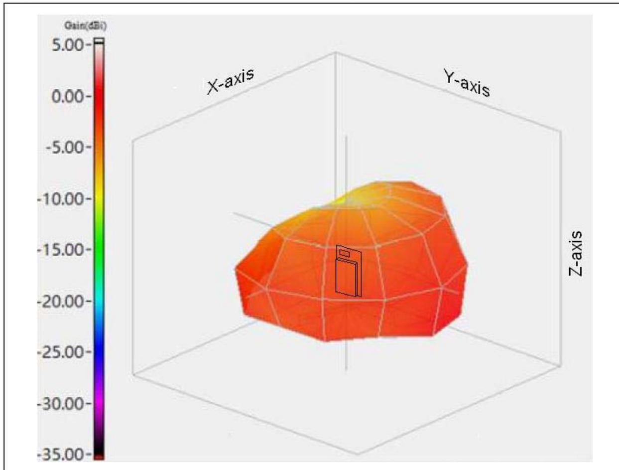
[Table 4-2](#) provides the antenna radiation pattern details of the BM71BLES1FC2 module.
