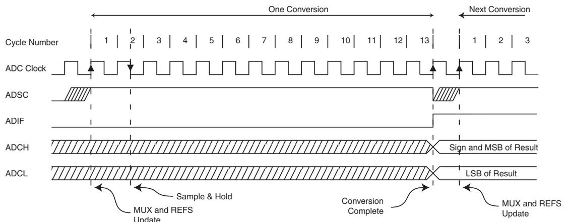
When Auto Triggering is used, the prescaler is reset when the trigger event occurs, as shown in [Figure 16-6](#) below. This assures a fixed delay from the trigger event to the start of conversion. In this mode, the sample-and-hold takes place two ADC clock cycles after the rising edge on the trigger source signal. Three additional CPU clock cycles are used for synchronization logic. Three additional CPU clock cycles are used for synchronization logic.
