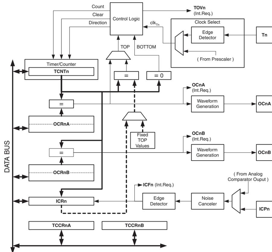
Most register and bit references in this section are written in general form. A lower case “n” replaces the Timer/Counter number, and a lower case “x” replaces the Output Compare unit channel. However, when using the register or bit defines in a program, the precise form must be used, i.e., TCNT1 for accessing Timer/Counter1 counter value and so on.
