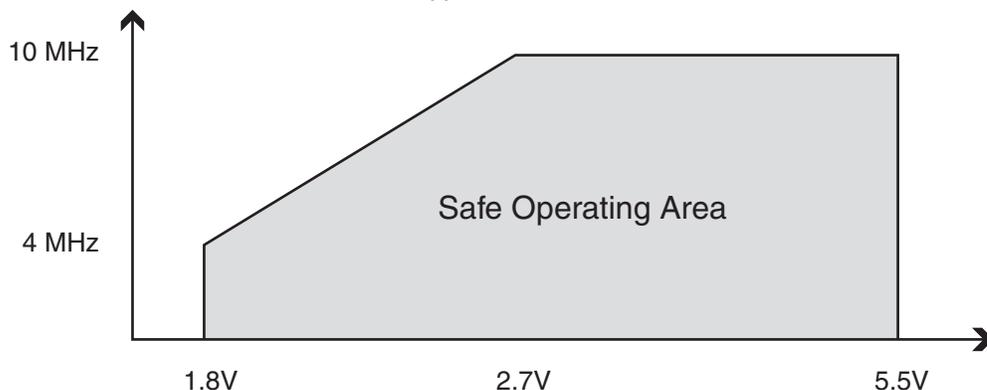
**Figure 20-2.** Maximum Frequency vs.  $V_{CC}$  (ATtiny24/44/84)
