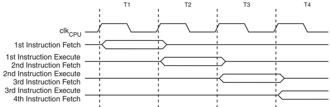
Figure 4-5 shows the internal timing concept for the Register File. In a single clock cycle an ALU operation using two register operands is executed, and the result is stored back to the destination register.
