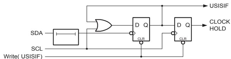
The start condition detector works asynchronously and can therefore wake up the processor from power-down sleep mode. However, the protocol used might have restrictions on the SCL hold time. Therefore, when using this feature the oscillator start-up time (set by CKSEL fuses, see [“Clock Sources” on page 25](#)) must also be taken into consideration. Refer to the description of the USISIF bit on [page 125](#) for further details.
