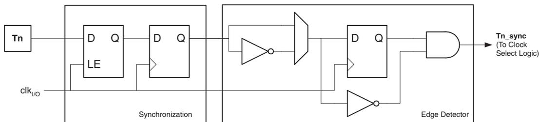
The edge detector generates one  $clk_{T0}$  pulse for each positive (CSn2:0 = 7) or negative (CSn2:0 = 6) edge it detects. The synchronization and edge detector logic introduces a delay of 2.5 to 3.5 system clock cycles from an edge has been applied to the Tn pin to the counter is updated.
