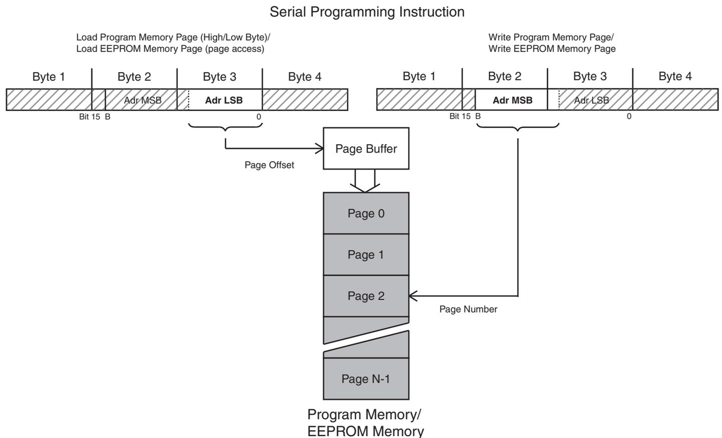
If the LSB in RDY/BSY data byte out is '1', a programming operation is still pending. Wait until this bit returns '0' before the next instruction is carried out.
