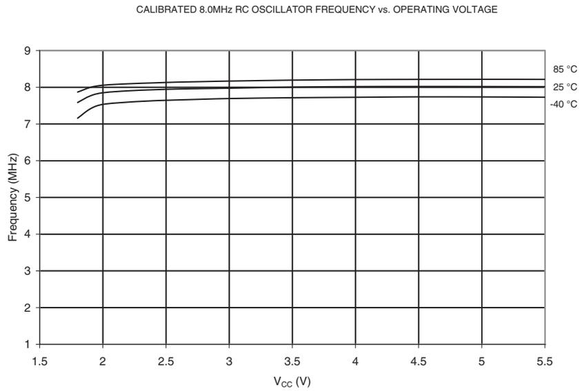
**Figure 21-41.** Calibrated 8 MHz RC oscillator Frequency vs. Temperature
