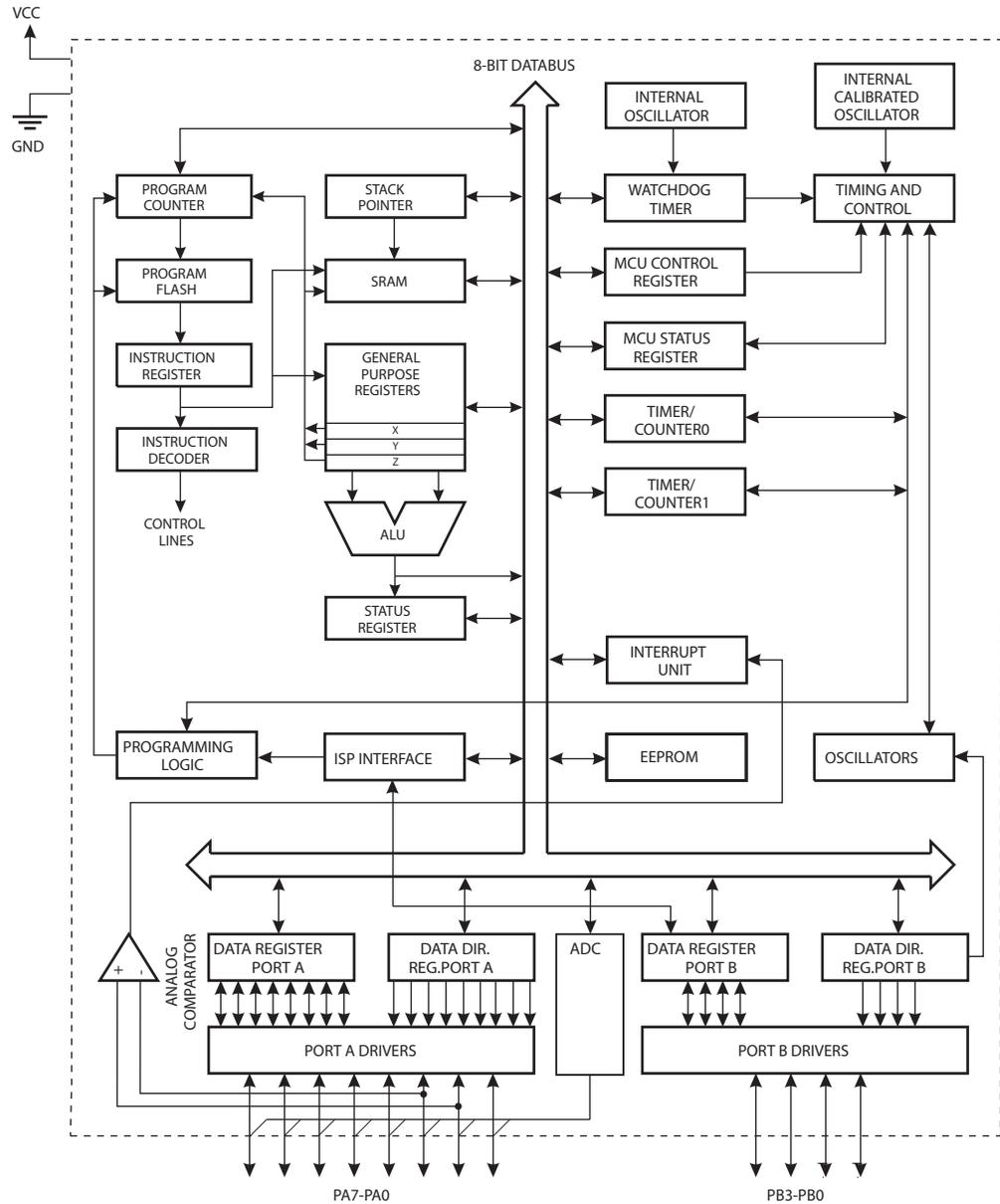
The AVR core combines a rich instruction set with 32 general purpose working registers. All 32 registers are directly connected to the Arithmetic Logic Unit (ALU), allowing two independent registers to be accessed in one single instruction executed in one clock cycle. The resulting architecture is more code efficient while achieving throughputs up to ten times faster than conventional CISC microcontrollers.
