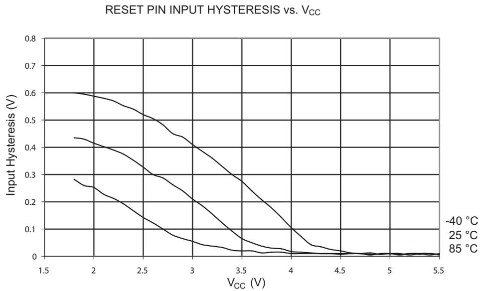
Figure 21-34. Reset Pin Input Hysteresis vs.  $V_{CC}$  (Reset Pin Used as I/O)
