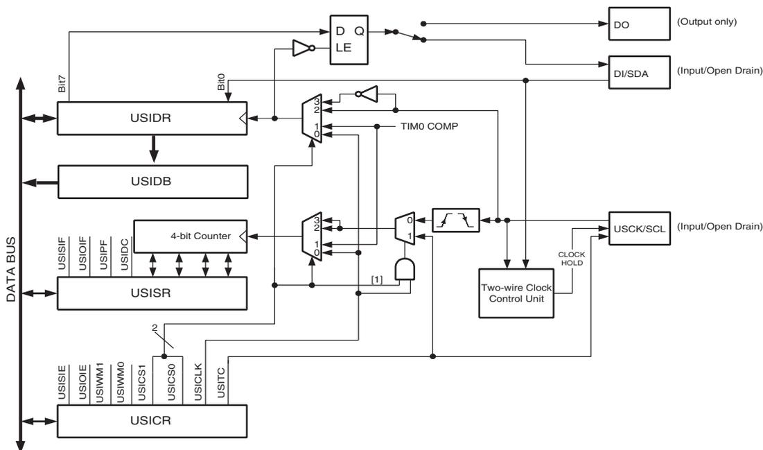
The 8-bit USI Data Register (USIDR) contains the incoming and outgoing data. It is directly accessible via the data bus but a copy of the contents is also placed in the USI Buffer Register (USIDB) where it can be retrieved later. If reading the USI Data Register directly, the register must be read as quickly as possible to ensure that no data is lost.
