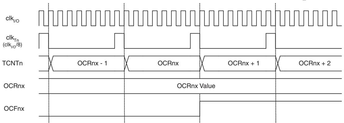
Figure 11-11 on page 80 shows the setting of OCF0A and the clearing of TCNT0 in CTC mode and fast PWM mode where OCR0A is TOP.
