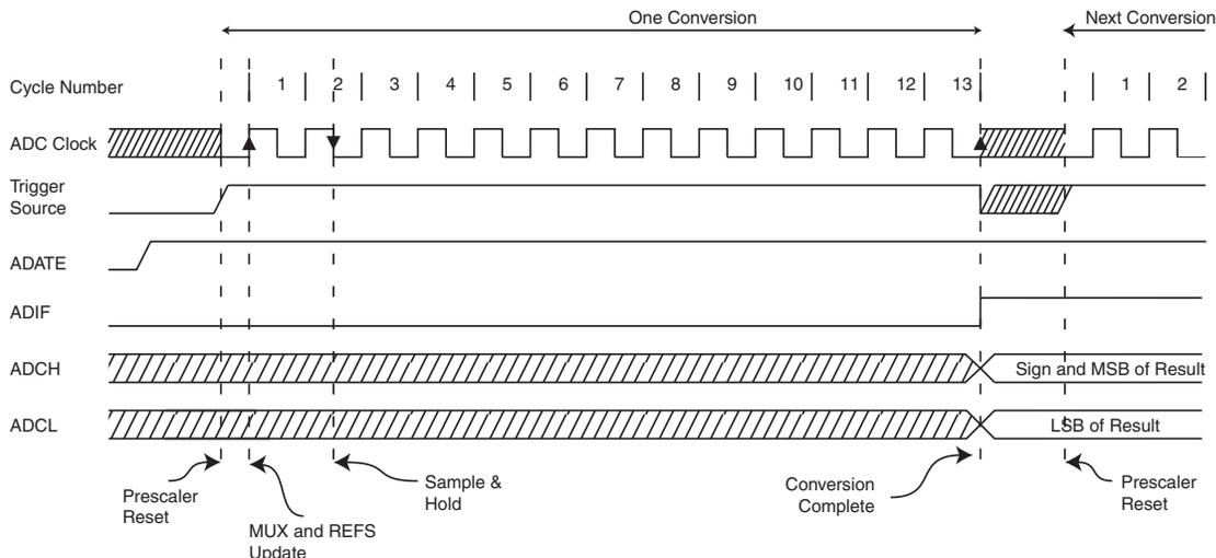
In Free Running mode, a new conversion will be started immediately after the conversion completes, while ADSC remains high. See [Figure 16-7](#).
