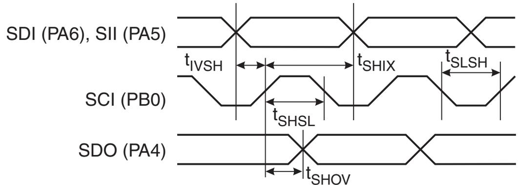
**Table 20-13.** High-voltage Serial Programming Characteristics
