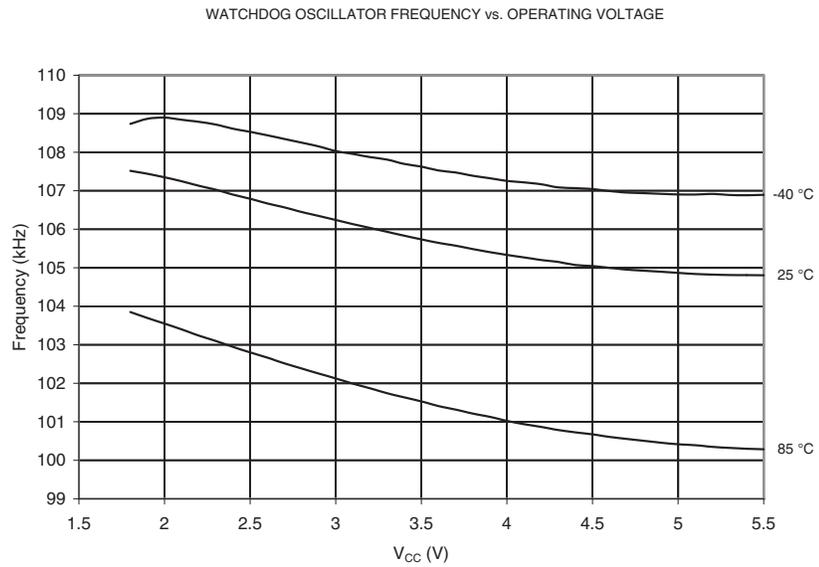
Figure 21-39. Watchdog Oscillator Frequency vs. Temperature
