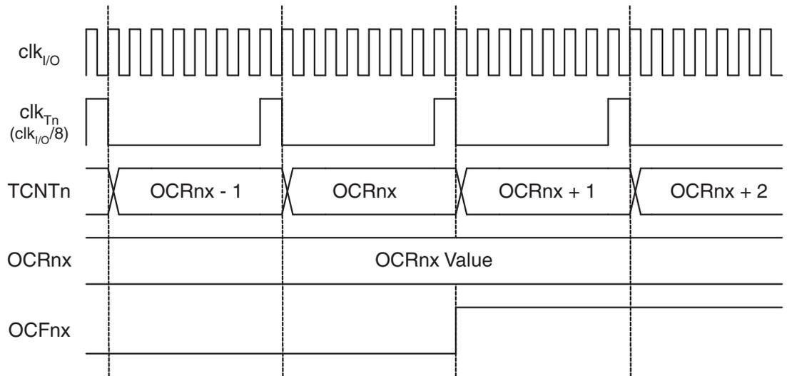
Figure 12-12 on page 104 shows the count sequence close to TOP in various modes. When using phase and frequency correct PWM mode the OCR1x Register is updated at BOTTOM. The timing diagrams will be the same, but TOP should be replaced by BOTTOM, TOP-1 by BOTTOM+1 and so on. The same renaming applies for modes that set the TOV1 flag at BOTTOM.
