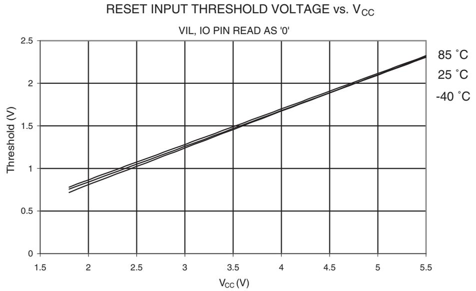
**Figure 21-33.** Reset Pin Input Hysteresis vs.  $V_{CC}$
