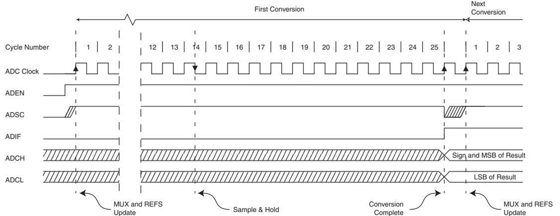
The actual sample-and-hold takes place 1.5 ADC clock cycles after the start of a normal conversion and 13.5 ADC clock cycles after the start of an first conversion. When a conversion is complete, the result is written to the ADC Data Registers, and ADIF is set. In Single Conversion mode, ADSC is cleared simultaneously. The software may then set ADSC again, and a new conversion will be initiated on the first rising ADC clock edge.
