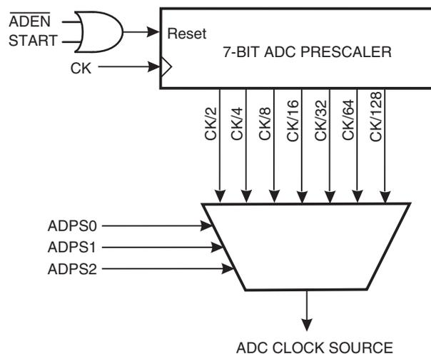
The ADC module contains a prescaler, as illustrated in [Figure 16-3 on page 135](#), which generates an acceptable ADC clock frequency from any CPU frequency above 100 kHz. The prescaling is set by the ADPS bits in ADCSRA. The prescaler starts counting from the moment the ADC is switched on by setting the ADEN bit in ADCSRA. The prescaler keeps running for as long as the ADEN bit is set, and is continuously reset when ADEN is low.
