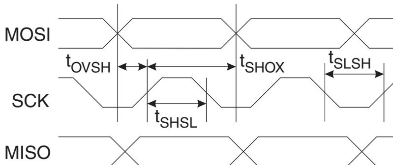
**Figure 20-5.** Serial Programming Waveform
