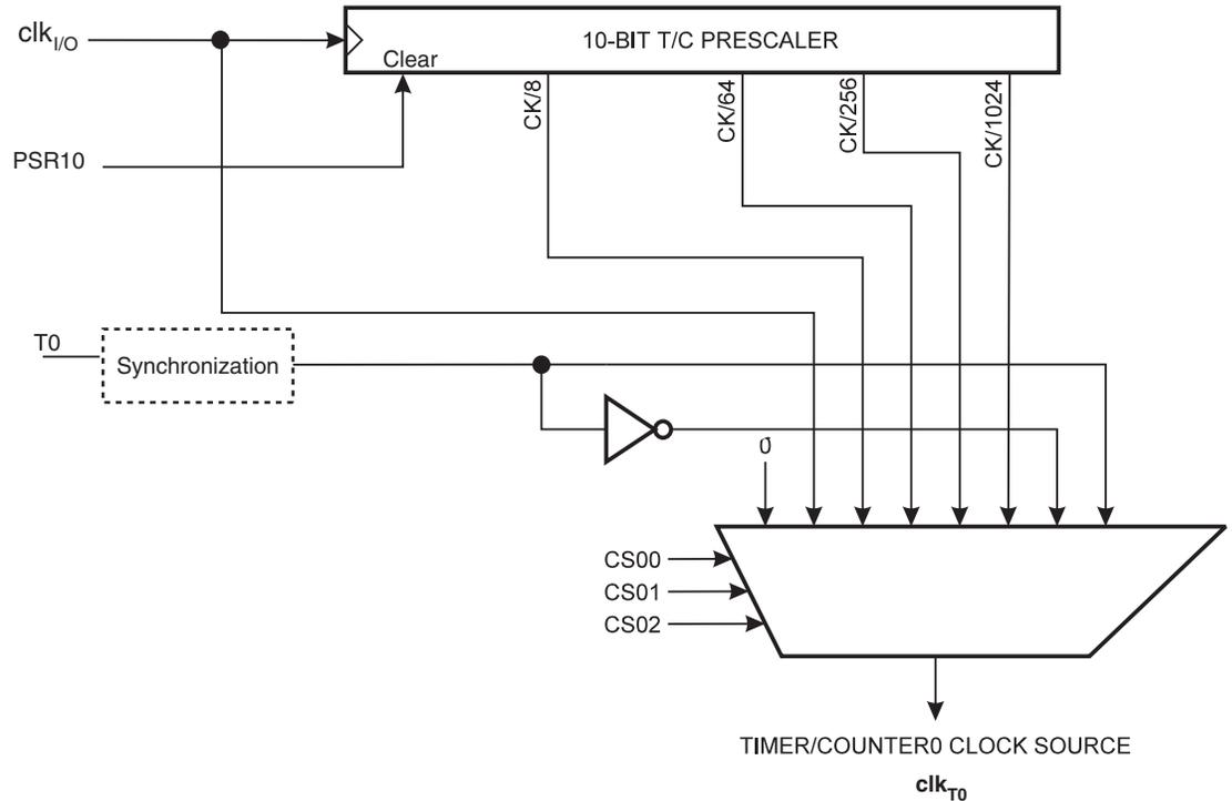
Note: 1. The synchronization logic on the input pins (T0) is shown in [Figure 13-1 on page 115](#).
