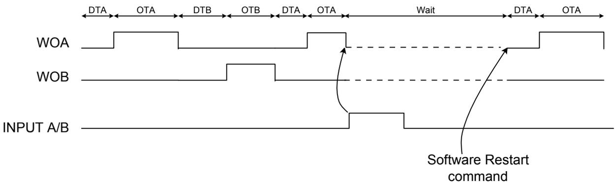
**Input Mode 8: Stop Output on Edge, Jump to Next Compare Cycle**
