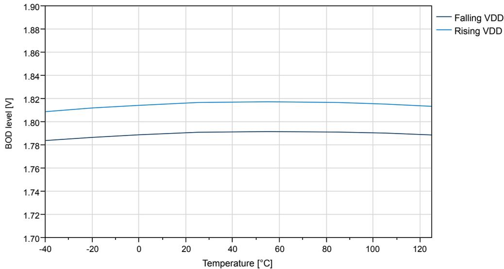
**Figure 35-39. BOD Threshold vs. Temperature (Level 2.6V)**
