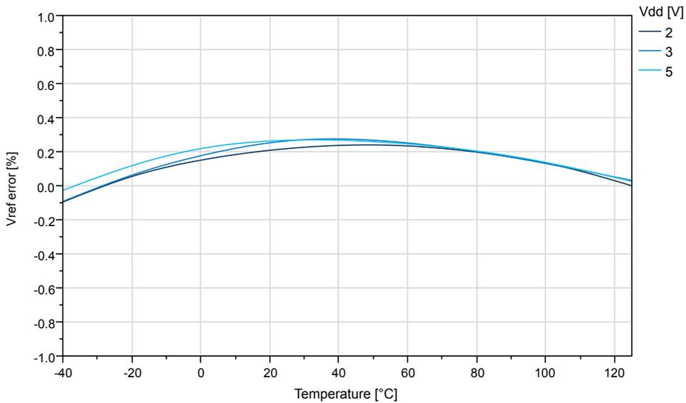
**Figure 35-33. Internal 2.5V Reference vs. Temperature**
