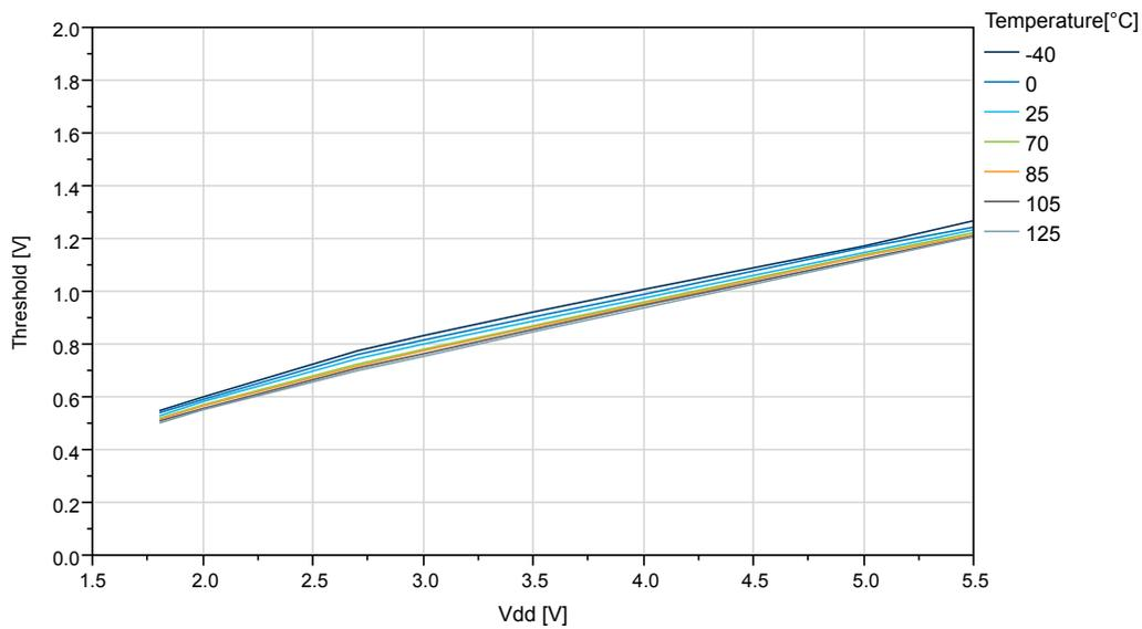
**Figure 35-17. IO Pin Input Threshold Voltage vs.  $V_{DD}$  ( $T=25^{\circ}\text{C}$ )**
