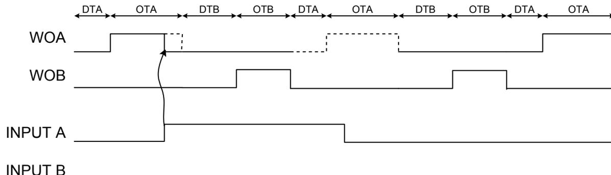
If Input mode 10 is used on input B and an input Event occurs, the WOB will be off as long as the Event lasts. If released during an on-time, it will be off for the rest of the on-time, too.
