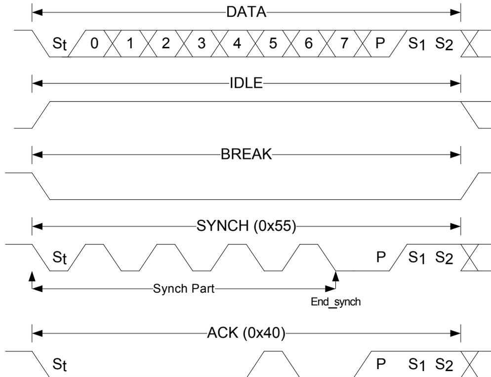
**Data Frame** Consist of 1 start bit (always low), 8 data bits, 1 parity bit (even parity) and two stop bits (always high). If the start bit, parity bit or stop bits have an incorrect value, an error will be detected and signaled by the UPDI. The parity bit check in the UPDI can be disabled by writing the PARD bit in UPDI.CTRLA, in which case the parity generation from the debugger can be ignored.
