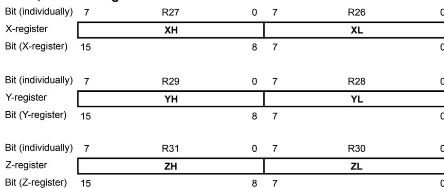
The lowest register address holds the least-significant byte (LSB), and the highest register address holds the most-significant byte (MSB). In the different addressing modes, these address registers function as fixed displacement, automatic increment, and automatic decrement.
