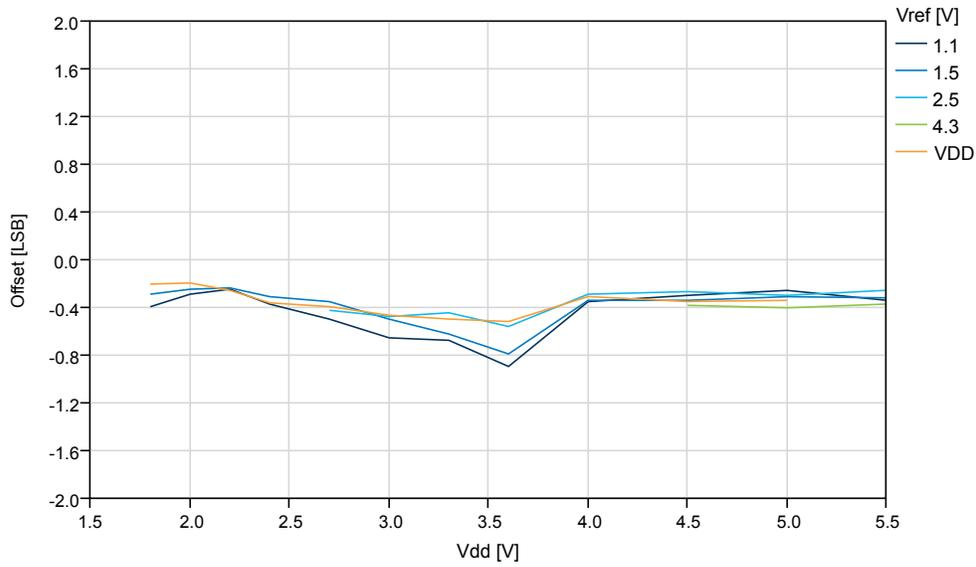
**Figure 35-50. Offset Error vs.  $V_{ref}$  ( $V_{DD}=5.0\text{V}$ , 115kps)**
