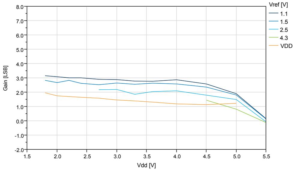
Figure 35-46. Gain Error vs.  $V_{ref}$  ( $V_{DD}=5.0\text{V}$ , 115kps)
