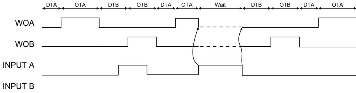
If Input mode 1 is used on input B, an Event will only have an effect if the TCD is in Dead time B or On-time B, and it will only effect the output WOB. When the event is done, the TCD counter starts at Dead time A.
