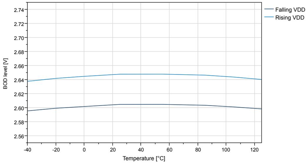
**Figure 35-40. BOD Threshold vs. Temperature (Level 4.3V)**
