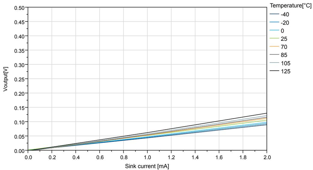
**Figure 35-21. IO Pin Output Voltage vs. Sink Current ( $V_{DD}=3.0V$ )**
