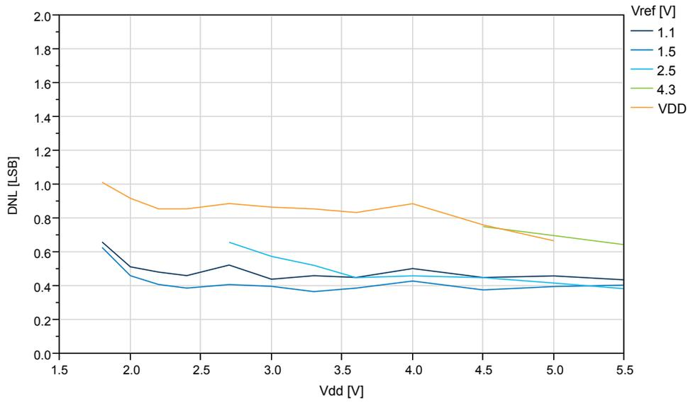
**Figure 35-44. DNL vs.  $V_{ref}$  ( $V_{DD}=5.0\text{V}$ , 115kps)**
