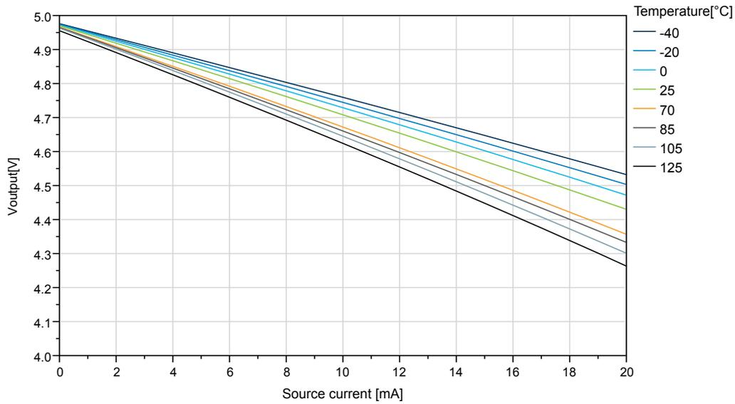
**Figure 35-27. IO Pin Output Voltage vs. Source Current (T=25°C)**
