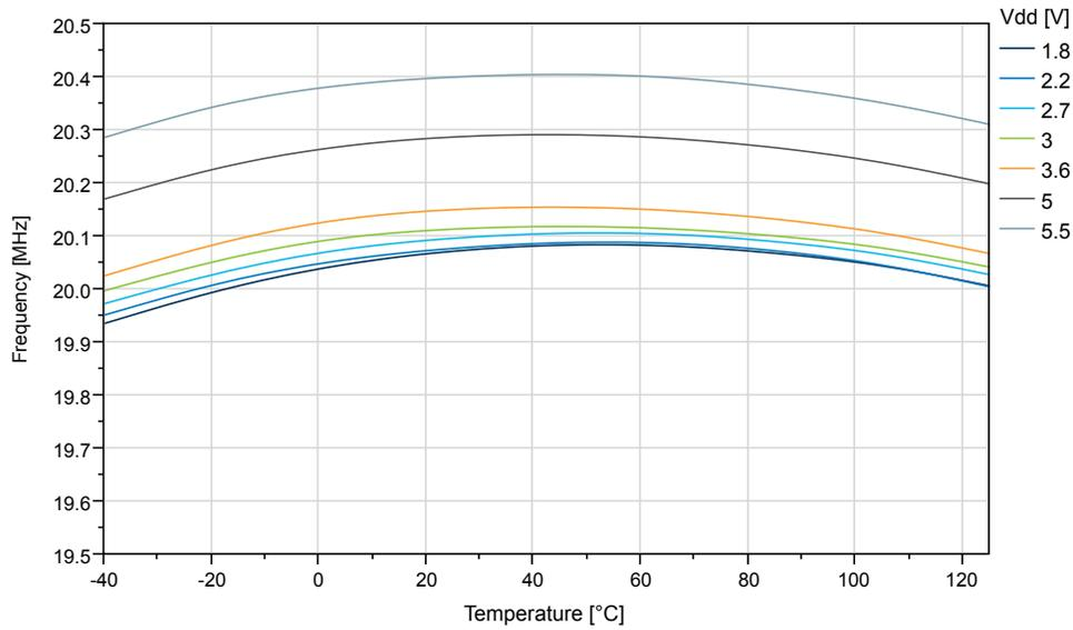
**Figure 35-58. OSC20M Internal Oscillator: Frequency vs. VDD**
