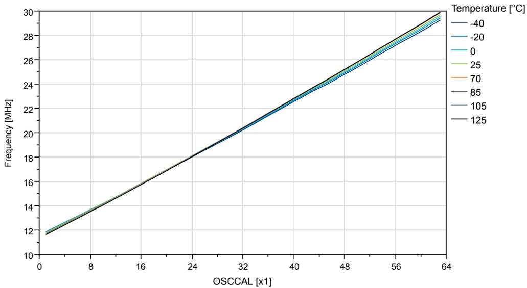
**Figure 35-57. OSC20M Internal Oscillator: Frequency vs. Temperature**
