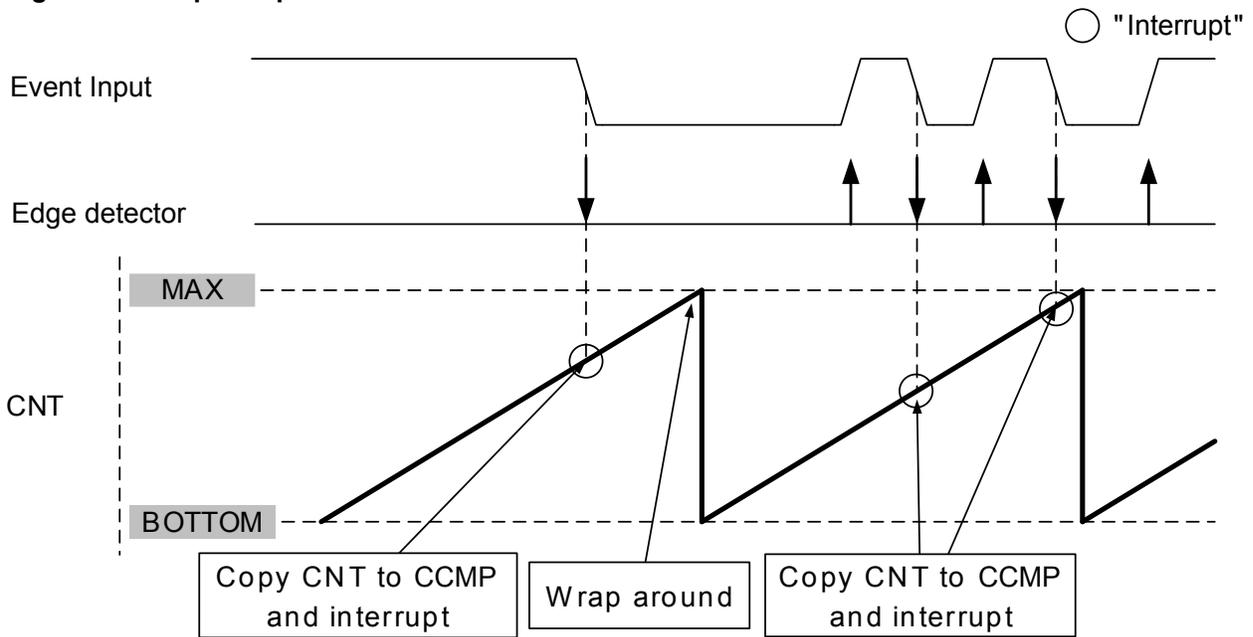
It is recommended to write zero to the TCB.CNT register when entering this mode from any other mode.
