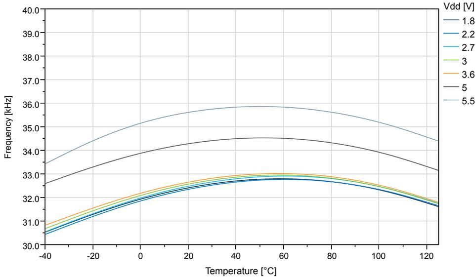
Figure 35-60. OSCULP32K Internal Oscillator Frequency vs. V<sub>DD</sub>
