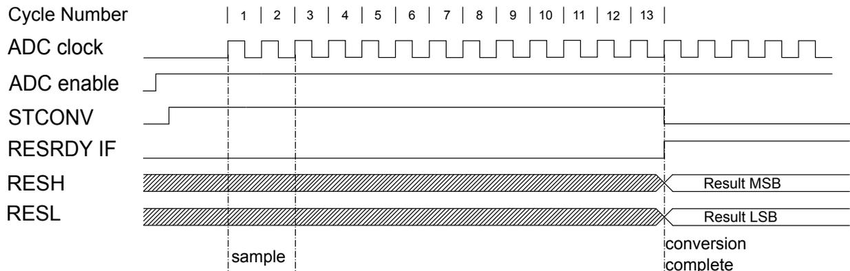
Both sampling time and sampling length can be adjusted using Sample Delay bit field in Control D (ADC.CTRLD) and sampling Sample Length bit field in the Sample Control register (ADC.SAMPCTRL). Both of these control the ADC sampling time in number of CLK\_ADC cycles. This allows sampling high-impedance sources without relaxing conversion speed. See register description for further information. Total sampling time is given by:
