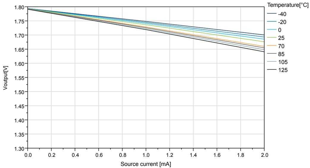
**Figure 35-25. IO Pin Output Voltage vs. Source Current ( $V_{DD}=3.0V$ )**
