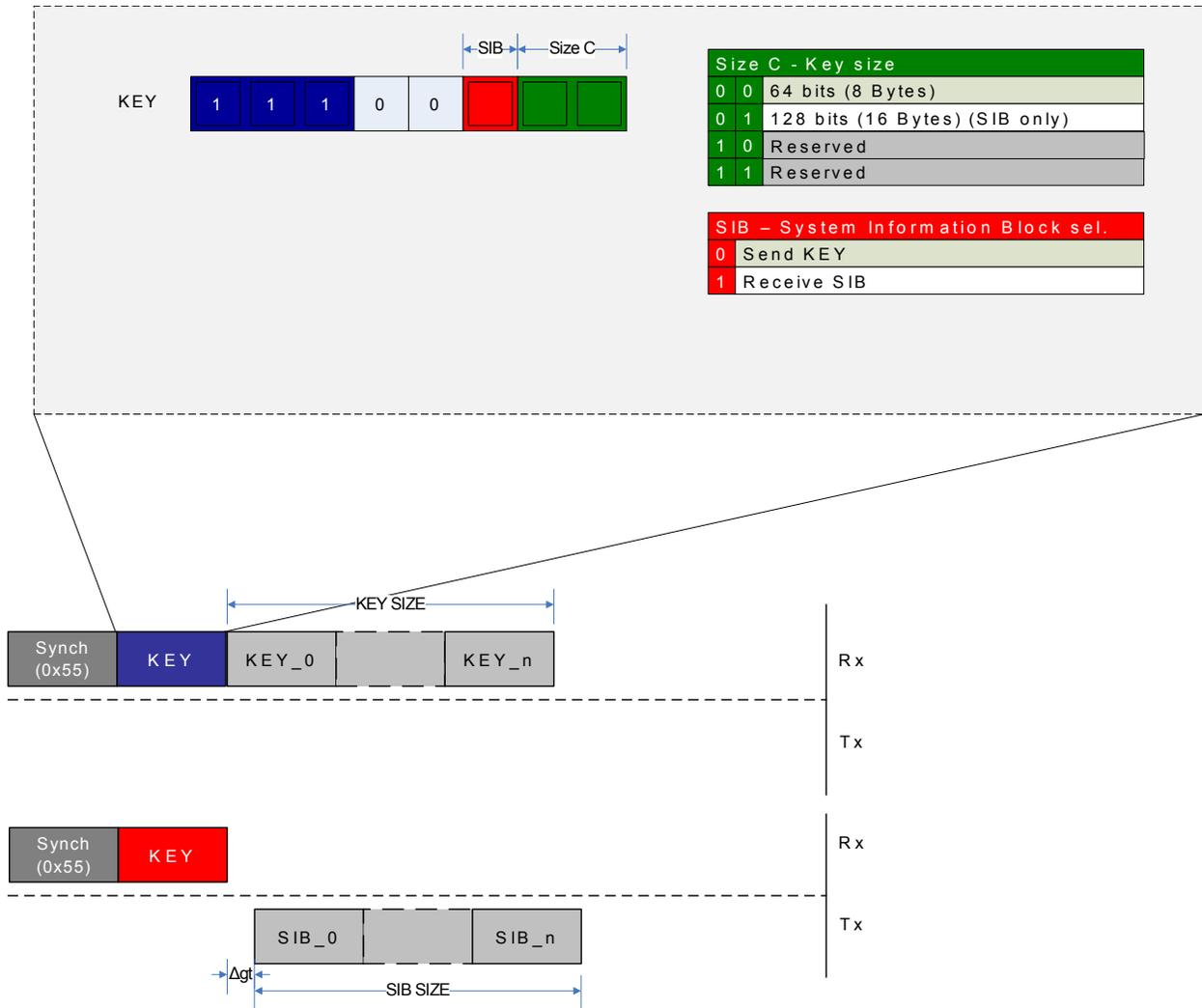
The Figure above shows the transmission of a KEY, and the reception of a SIB. In both cases, the `SIZE_C` field in the opcode determines the number of frames to be sent or received. There is no response after sending a `KEY` to the UPDI. When requesting the SIB, data will be transmitted from the UPDI according to the current Guard Time setting.
