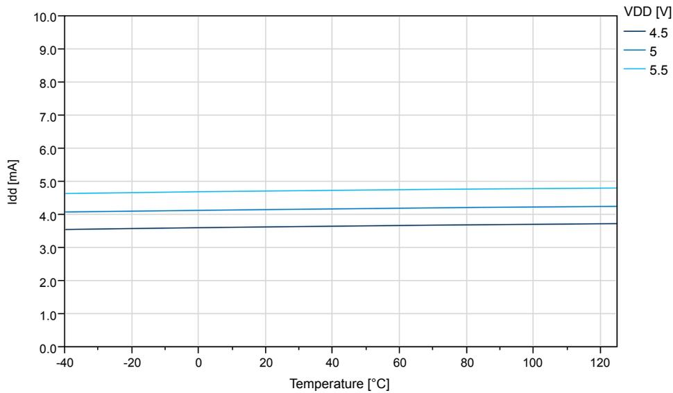
Figure 35-9. Idle Supply Current vs.  $V_{DD}$  (f=32KHz OSCULP32K)
