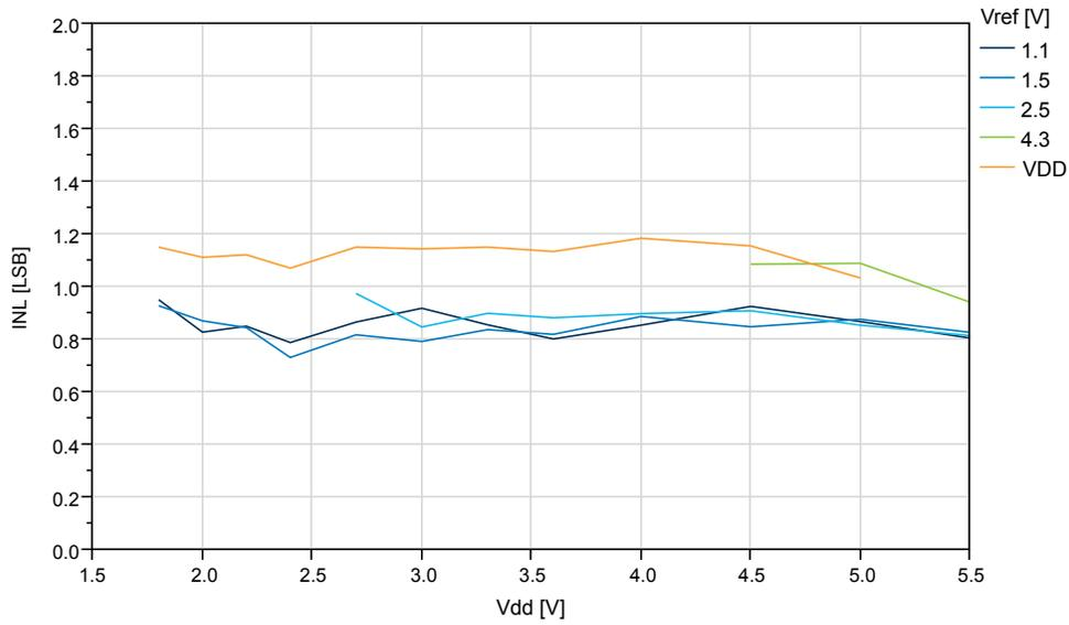
**Figure 35-48. INL vs.  $V_{ref}$  ( $V_{DD}=5.0\text{V}$ , 115ksps)**
