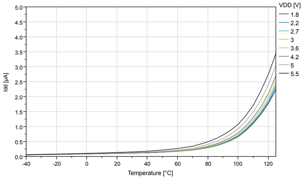
**Figure 35-11. Power Down Mode Supply Current vs.  $V_{DD}$  (all functions disabled)**
