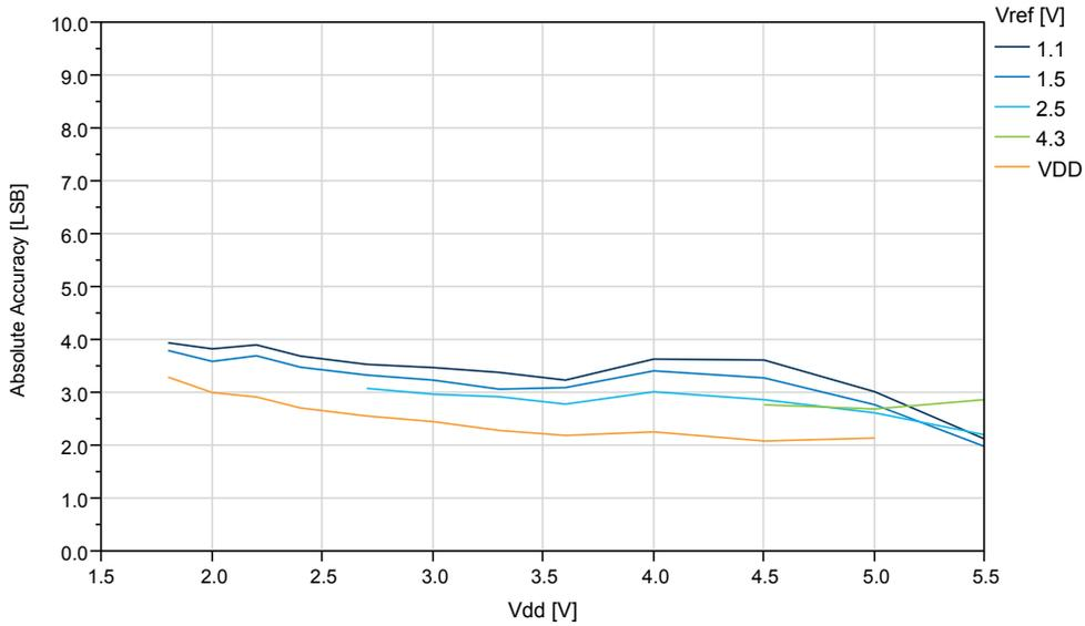
Figure 35-42. Absolute Accuracy vs.  $V_{ref}$  ( $V_{DD}=5.0\text{V}$ , 115kps)
