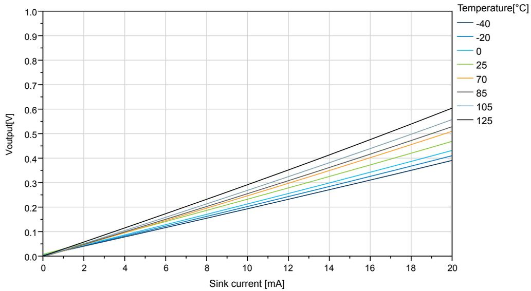
**Figure 35-23. : IO Pin Output Voltage vs. Sink Current (T=25°C)**
