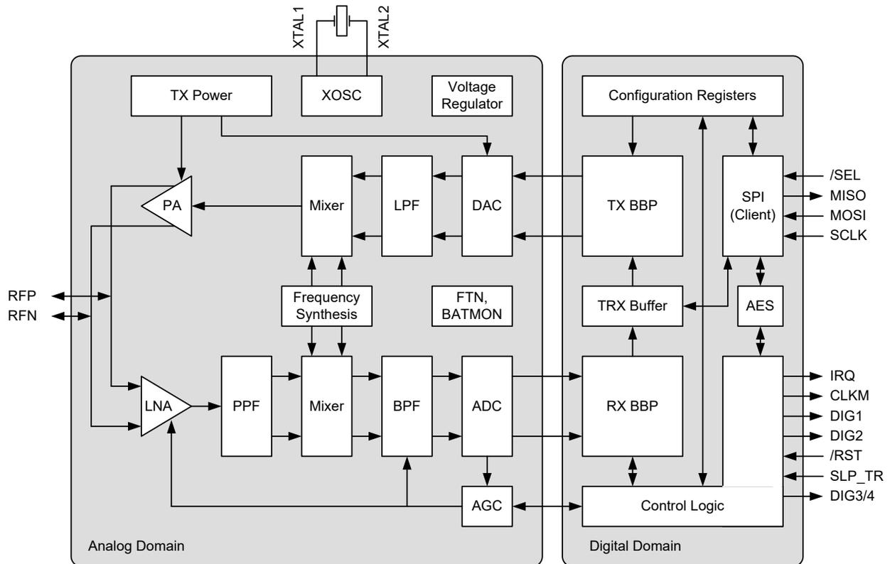
The number of required external components is minimal. The basic requirements are an antenna, a balun, harmonic filter, crystal oscillator and bypass capacitors. The RF Ports are bidirectional differential signals that do not require external TX/RX switches. Hardware control signals are automatically generated for TX/RX arbitration of high-powered PA/LNA front ends and transmitter diversity for systems with dual antennas.
