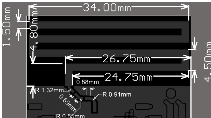
The following figure shows the bottom layer layout of the reference board directly beneath the RF traces.
