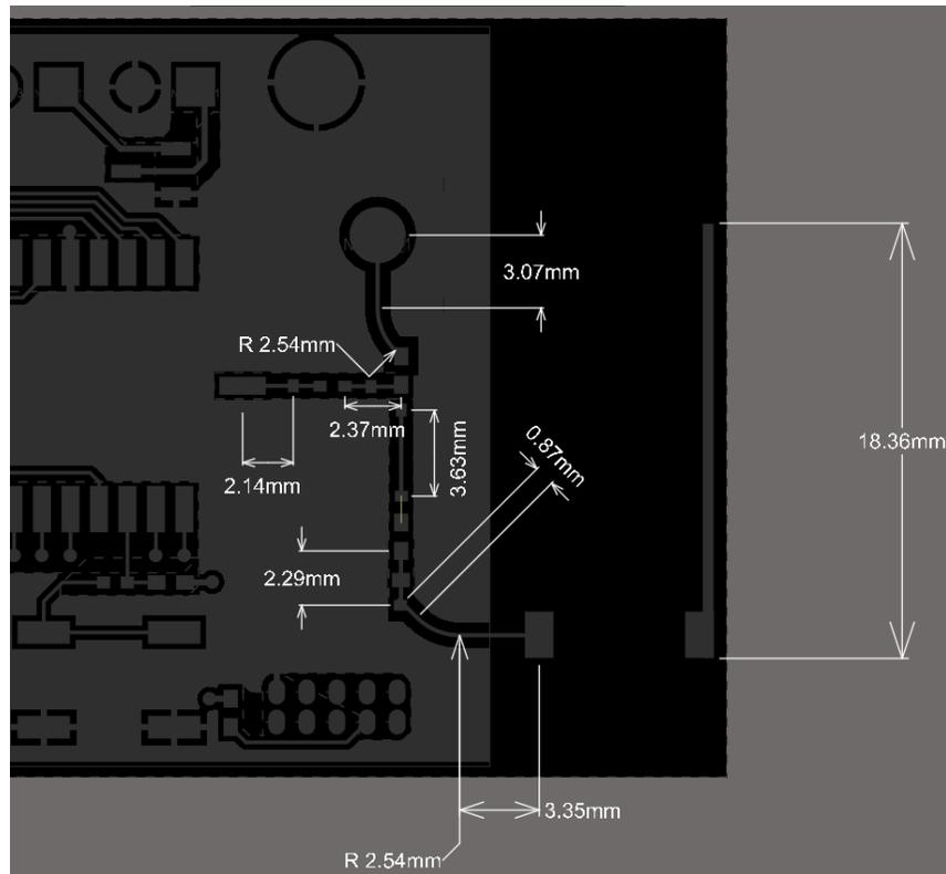
Figure 12-5. Layer 2 (GND) Layout
