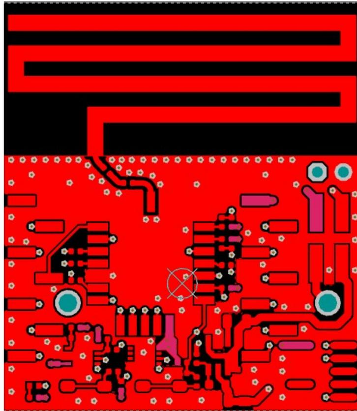
The following figure shows the top layer layout of the reference host Sensor board focussed on RF traces and PCB antenna. The snapshot also indicates the critical dimensions that are required to be replicated in the design to maintain compliance.
