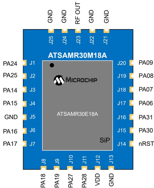
The module pin assignment is shown in the following table. The **SiP pin** column is a reference to the [ATSAMR30E18 datasheet](#) (ATSAMR30E18A).
