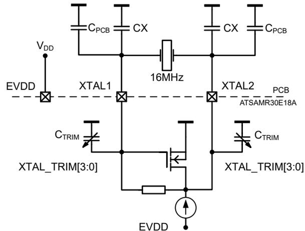
Additional internal trimming capacitors  $C_{TRIM}$  are available. Any value in the range from 0 pF to 4.5 pF with a 0.3 pF resolution is selectable using the XTAL\_TRIM bits in the XOSC\_CTRL register (XOSC\_CTRL.XTAL\_TRIM). To calculate the total load capacitance, the following formula can be used:
