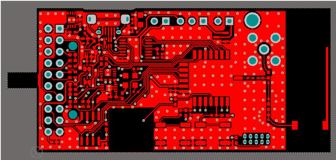
The following figure shows the top layer layout of the reference board focused on the RF traces. The snapshot also indicates the critical dimensions that are required to be replicated in the design to maintain compliance.
