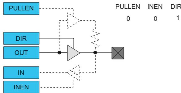
**Figure 32-7. I/O Configuration - Totem-Pole Output with Enabled Input**
