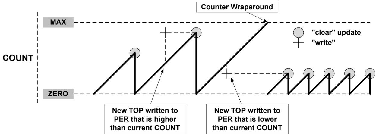
A counter wraparound can occur in any operation mode when up-counting without buffering, see [Figure 38-8](#).
