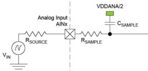
The minimum sampling time  $t_{\text{samplehold}}$  for a given  $R_{\text{source}}$  can be calculated using the following formula:
