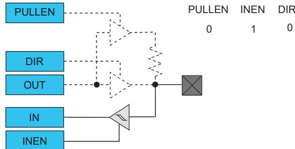
**Figure 32-5. I/O Configuration - Input with Pull**
