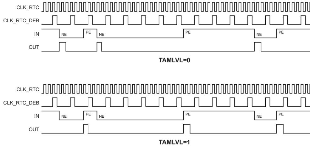
**Figure 27-7. Edge Detection with Synchronous Stability Debouncing**
