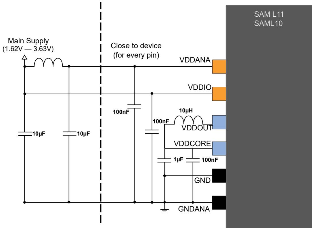
**Figure 51-2. Power Supply Connection for Linear Mode Only**
