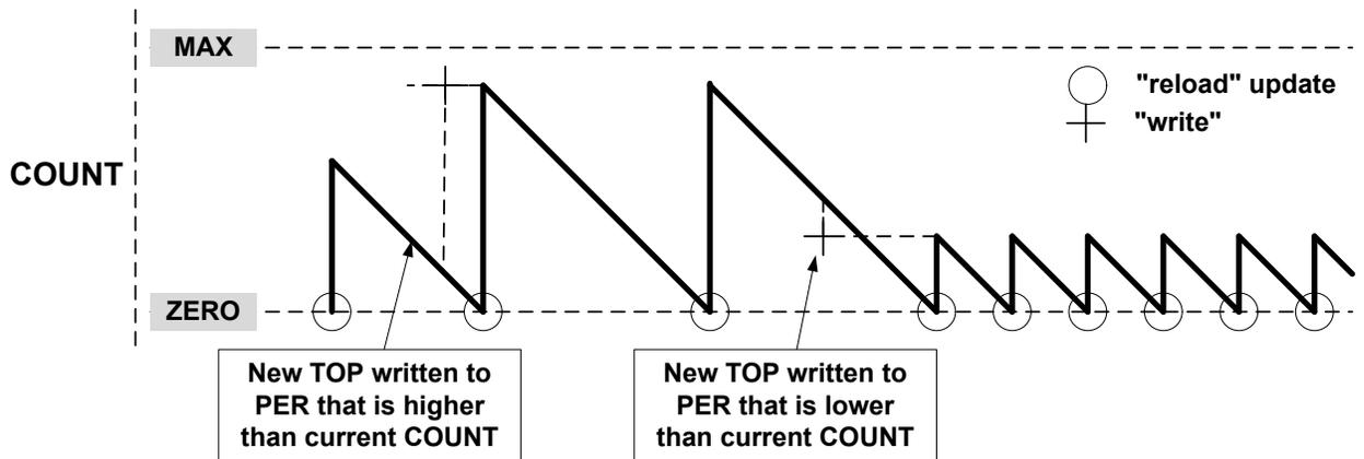
When double buffering is used, the buffer can be written at any time and the counter will still maintain correct operation. The period register is always updated on the update condition, as shown in [Figure 38-10](#). This prevents wraparound and the generation of odd waveforms.
