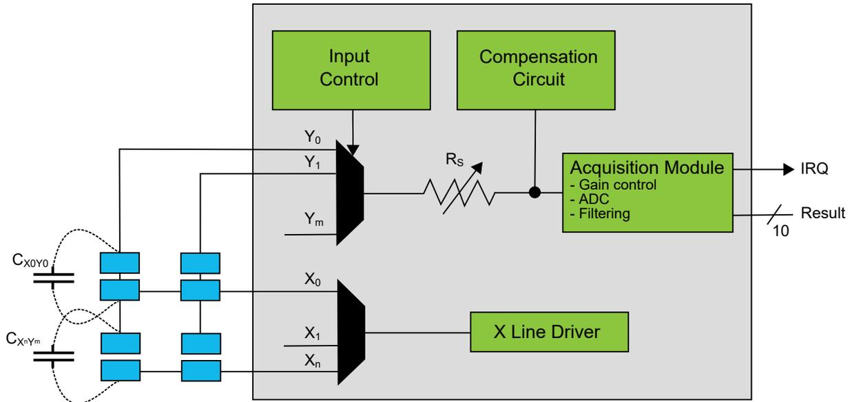
**Note:** For SAM L10/L11 the  $R_s = 100\text{ K}\Omega$ .
