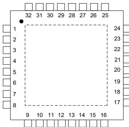
Figure 4-4. SAM L10/L11 32-pin WLCSP Pinout
