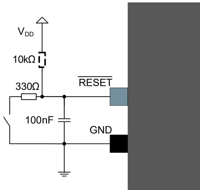
**Figure 51-6. External Reset Circuit Schematic (EFT Immunity Enhancement)**
