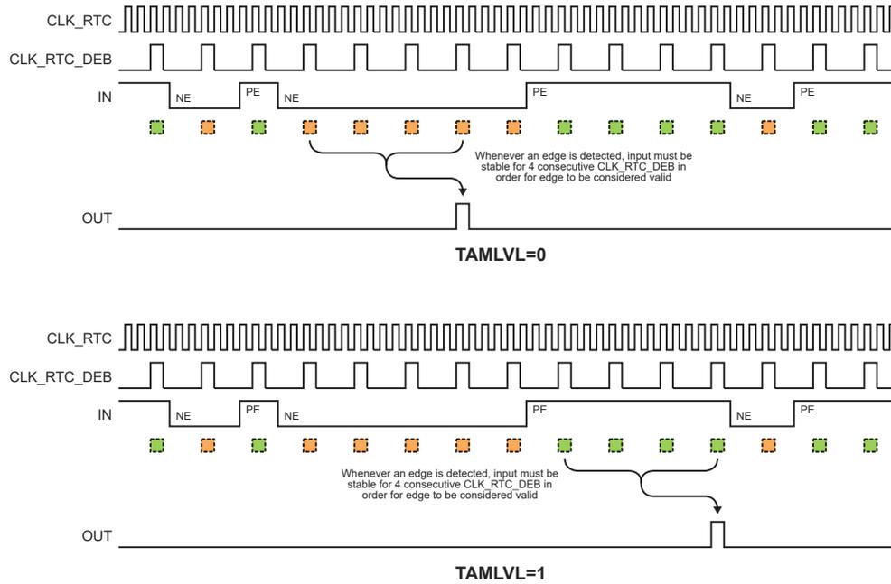
**Figure 27-8. Edge Detection with Asynchronous Stability Debouncing**
