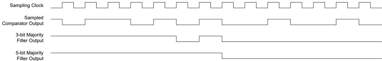
**Figure 42-7. Single-Shot Filtering**
