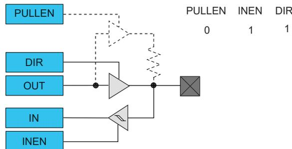
**Figure 32-8. I/O Configuration - Output with Pull**
