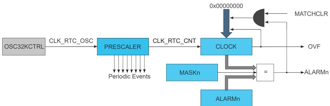
**Figure 27-4. RTC Block Diagram (Tamper Detection Use Case)**
