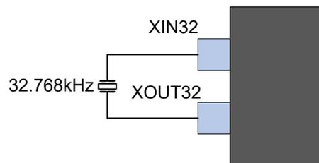
To improve accuracy and safety, it has recommended to add external capacitors, as recommend in the crystal data sheet. See figure below for additional information.
