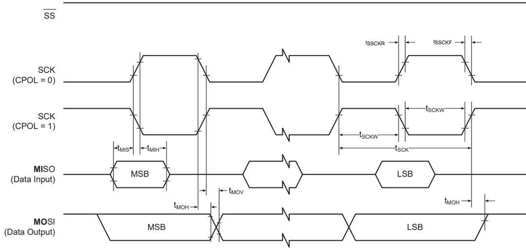
**Figure 46-8. SPI Timing Requirements in Client Mode**
