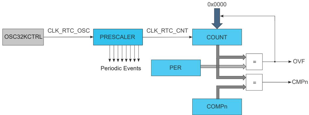
**Figure 27-3. RTC Block Diagram (Mode 2 — Clock/Calendar)**
