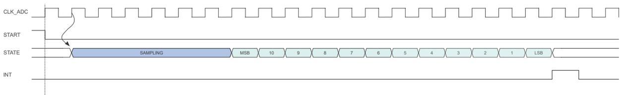
The ADC provides also offset compensation, see the following figure. The offset compensation is enabled by the Offset Compensation bit in the Sampling Control register (SAMPCTRL.OFFCOMP).
