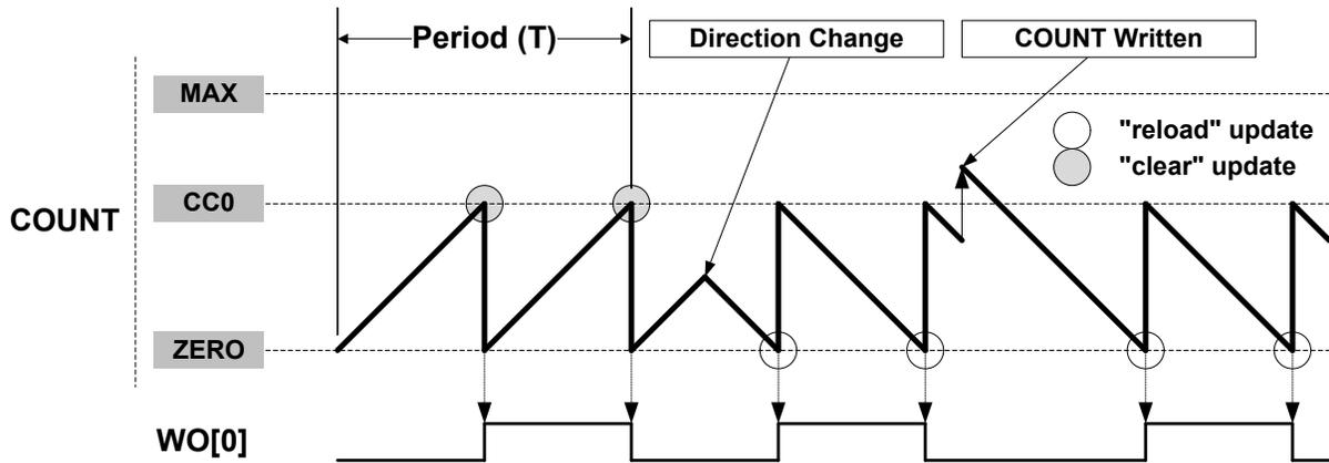
**Normal Pulse-Width Modulation Operation (NPWM)**
