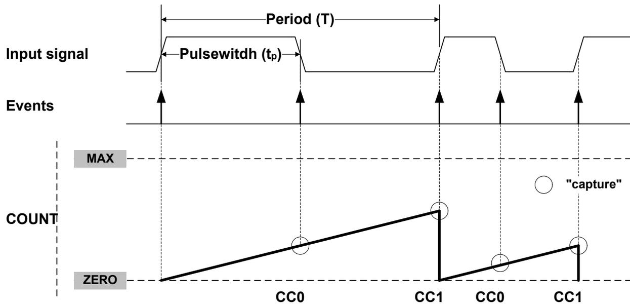
Selecting PWP in the Event Action bit group in the Event Control register (EVCTRL.EVACT) enables the TC to perform one capture action on the rising edge and another one on the falling edge. The period  $T$  will be captured into CC1 and the pulse width  $t_p$  in CC0. EVCTRL.EVACT = PPW (period and pulse-width) offers identical functionality, but will capture  $T$  into CC0 and  $t_p$  into CC1.
