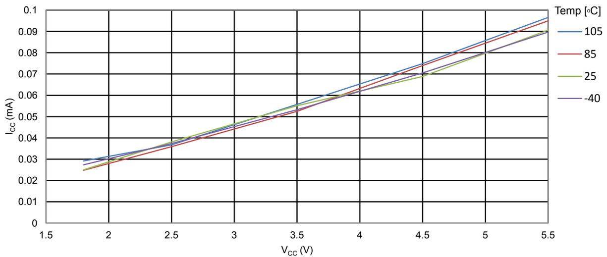
**Figure 34-4. ATmega328PB: Active Supply Current vs.  $V_{CC}$  (Internal RC Oscillator, 1MHz)**
