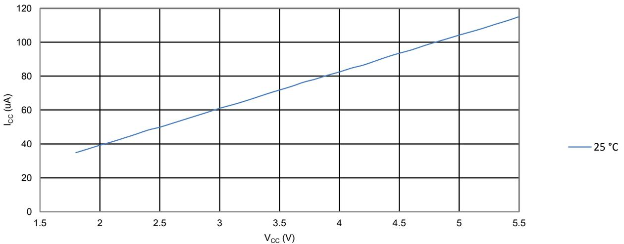
**Figure 34-50. ATmega328PB: Brownout Detector Current vs. Vcc**
