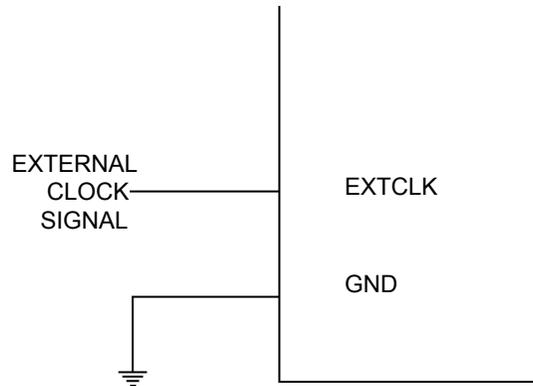
When this clock source is selected, start-up times are determined by the SUT Fuses:
