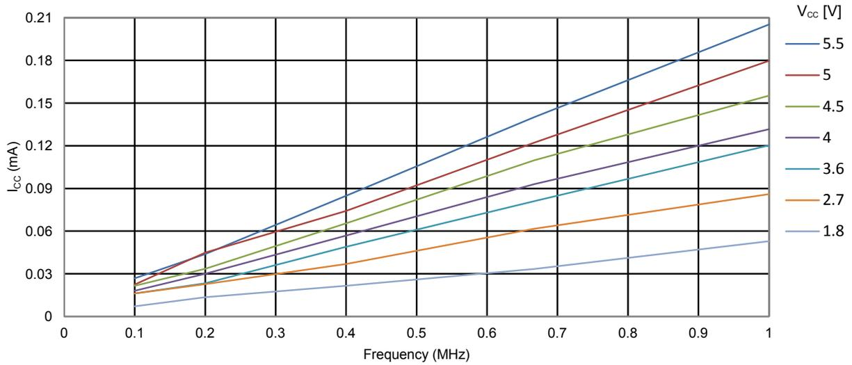
Figure 34-9. ATmega328PB: Idle Supply Current vs. Frequency (1-20MHz)
