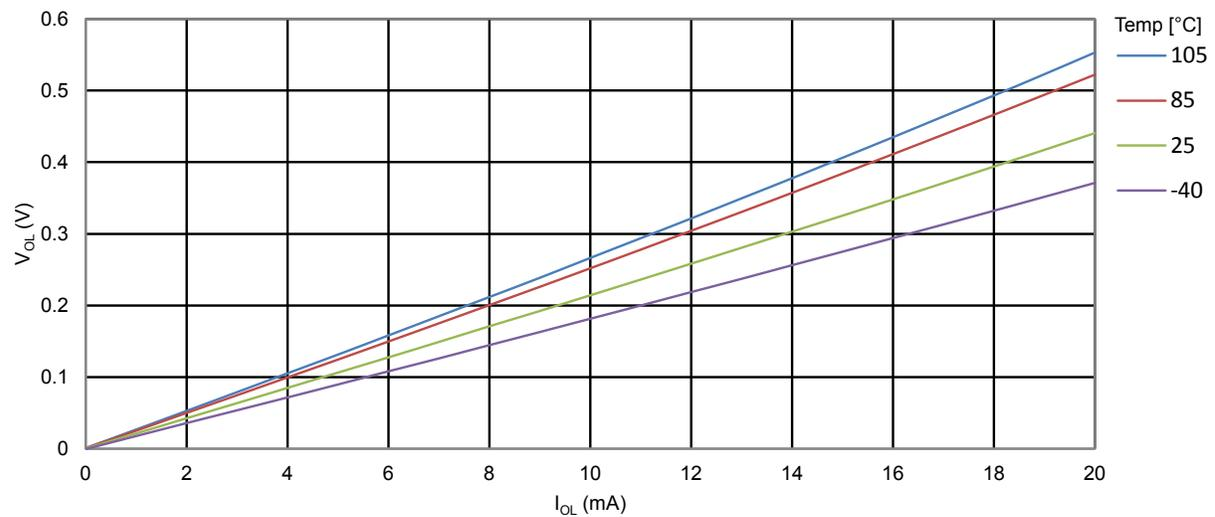
**Figure 34-24. ATmega328PB: I/O Pin Output Voltage vs. Source Current ( $V_{CC} = 3V$ )**
