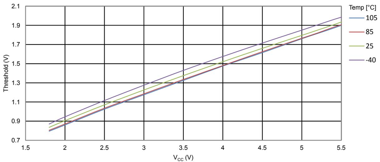
**Figure 34-28. ATmega328PB I/O Pin Input Hysteresis vs.  $V_{CC}$**
