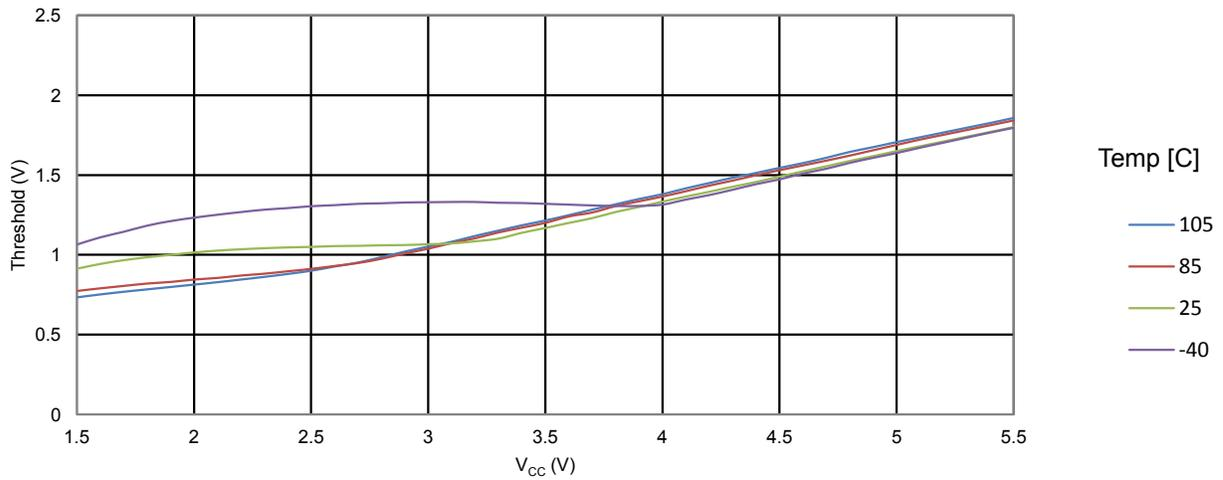
**Figure 34-30. ATmega328PB Reset Input Threshold Voltage vs.  $V_{CC}$  ( $V_{IL}$ , I/O Pin read as '0')**
