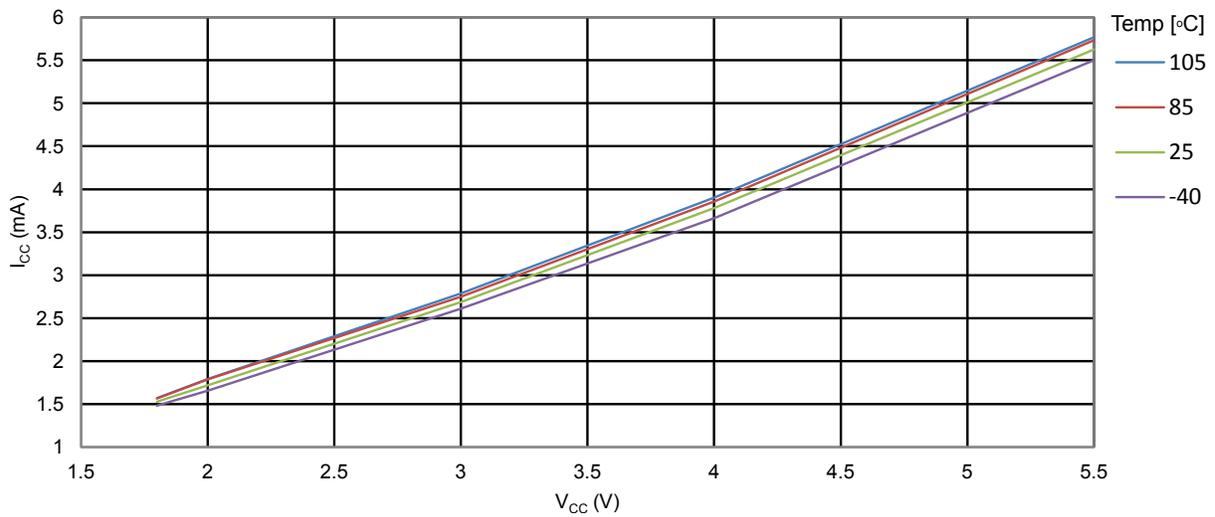
**Figure 34-6. ATmega328PB: Active Supply Current vs.  $V_{CC}$  (With ADC, conversion 50kHz)**
