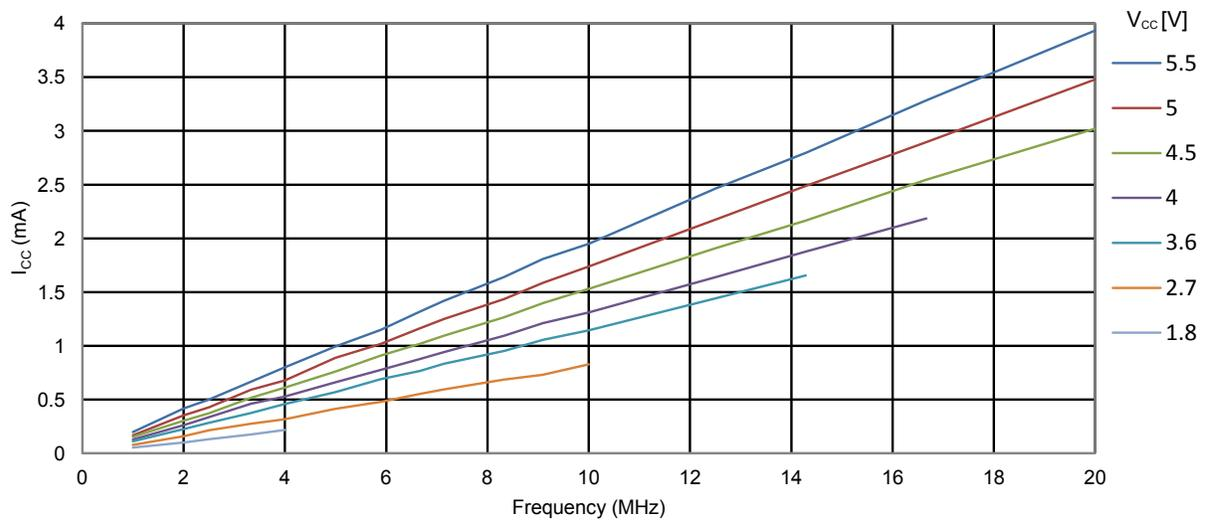
**Figure 34-10. ATmega328PB: Idle Supply Current vs.  $V_{CC}$  (Internal RC Oscillator, 128kHz)**
