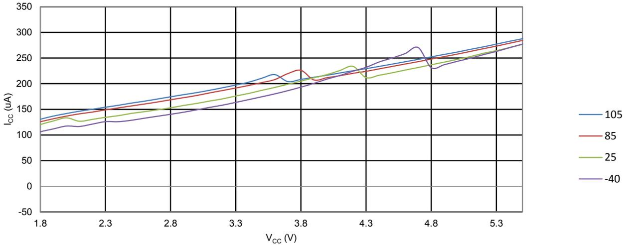
Figure 34-48. ATmega328PB: Analog Comparator Current vs. Vcc
