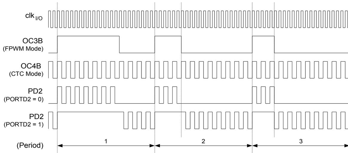
In this example, Timer/Counter4 provides the carrier, while the modulating signal is generated by the Output Compare unit B of the Timer/Counter3.
