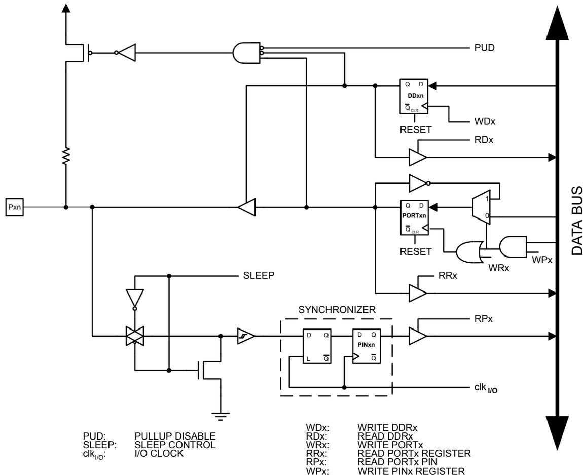
Note: 1. WRx, WPx, WDx, RRx, RPx, and RDx are common to all pins within the same port. clk<sub>I/O</sub>, SLEEP, and PUD are common to all ports.
