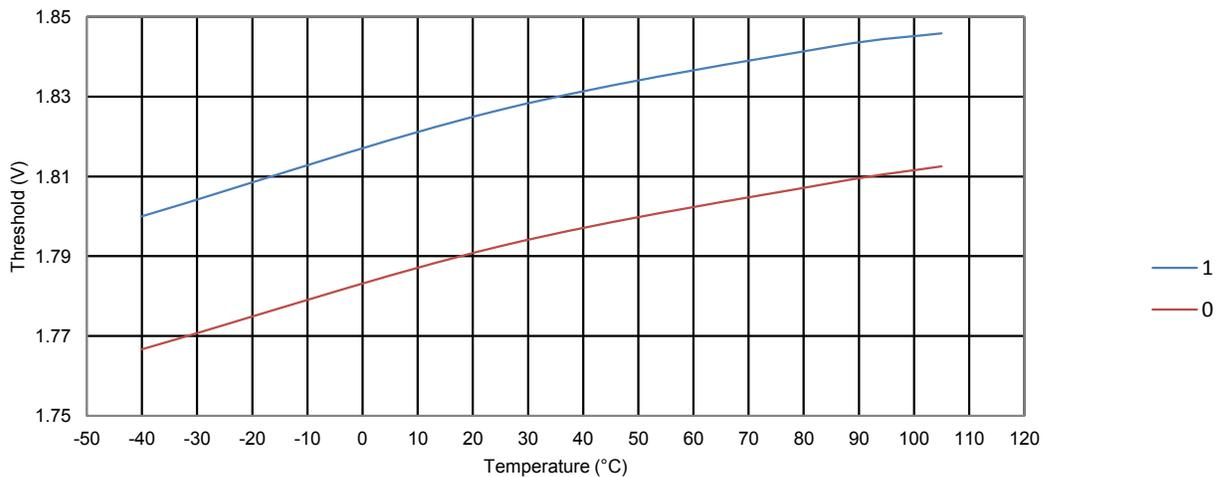
**Figure 34-33. ATmega328PB: BOD Thresholds vs. Temperature (BODLEVEL is 2.7V)**
