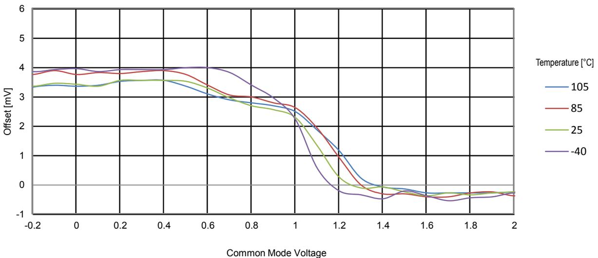
**Figure 34-39. ATmega328PB AC Offset vs. Common Voltage ( $V_{CC} = 3.0V$ )**
