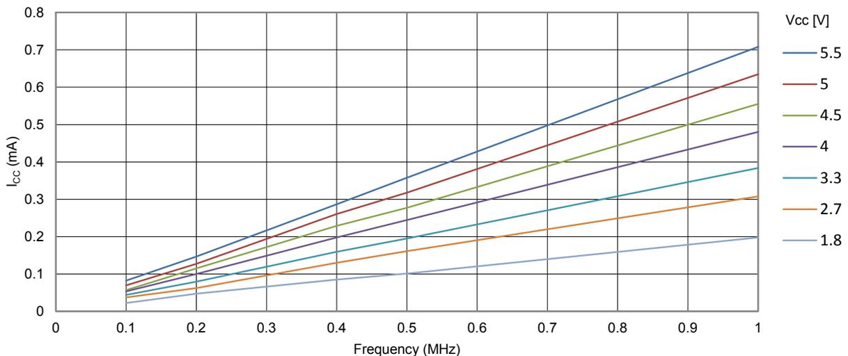
**Figure 34-2. ATmega328PB: Active Supply Current vs. Frequency (1-20MHz)**
