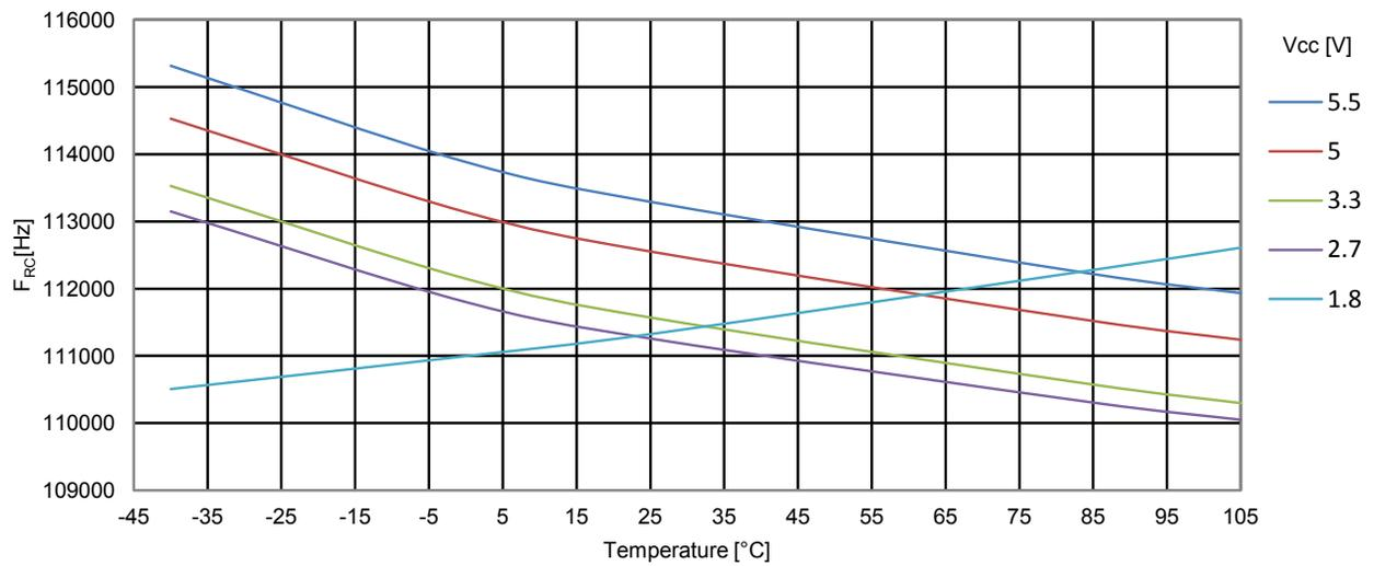
Figure 34-42. ATmega328PB: Watchdog Oscillator Frequency vs.  $V_{CC}$
