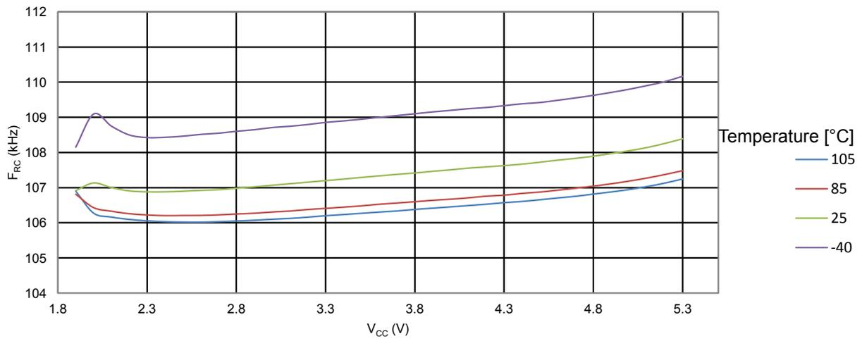
**Figure 34-43. ATmega328PB: Calibrated 8MHz RC Oscillator Frequency vs.  $V_{CC}$**
