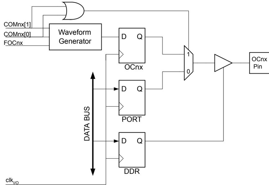
**Note:** The “n” in the register and bit names indicates the device number (n = 1, 3, 4 for Timer/Counter 1, 3, 4), and the “x” indicates Output Compare unit (A/B).
