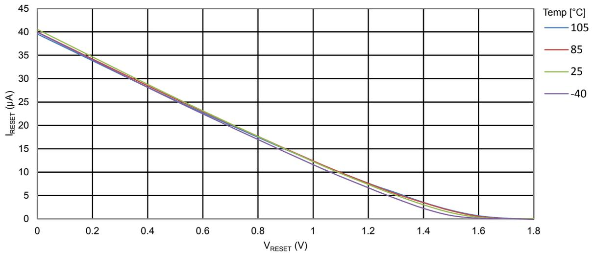
**Figure 34-20. ATmega328PB: Reset Pull-up Resistor Current vs. Reset Pin Voltage ( $V_{CC} = 2.7V$ )**
