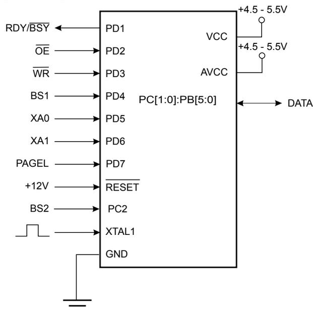
Note:  $V_{CC} - 0.3V < AV_{CC} < V_{CC} + 0.3V$ ; however,  $AV_{CC}$  should always be within 4.5 - 5.5V
