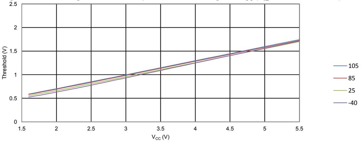
**Figure 34-31. ATmega328PB Reset Pin Input Hysteresis vs.  $V_{CC}$**
