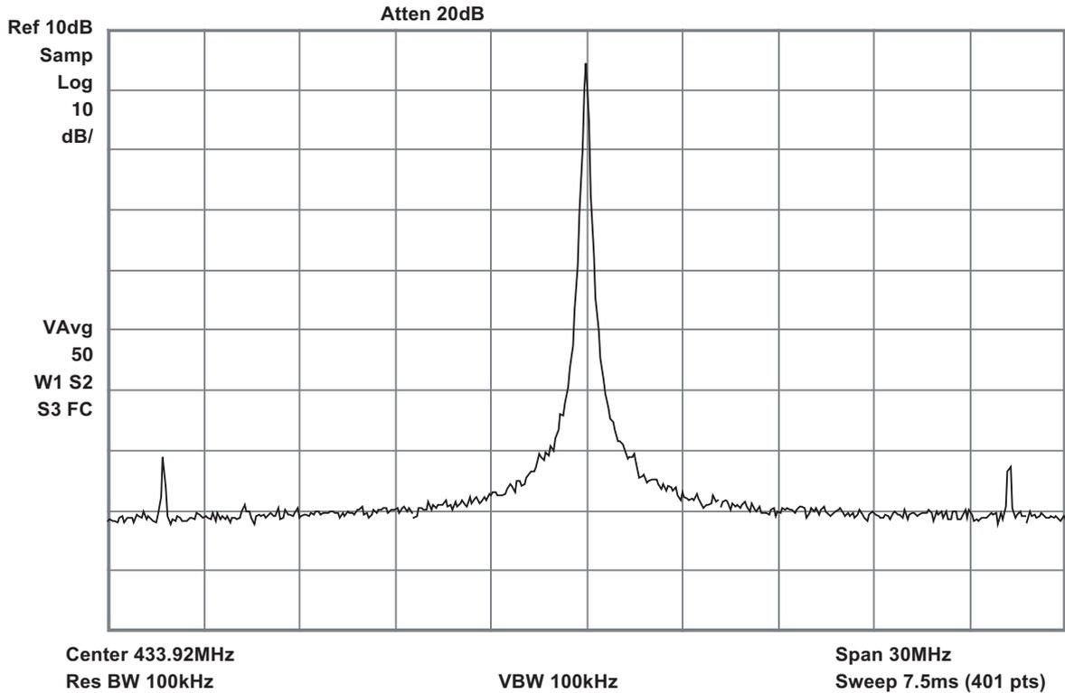
Figure 3-8. Unmodulated TX Spectrum 433.92MHz – 16.17kHz ( $f_{FSK\_L}$ )
