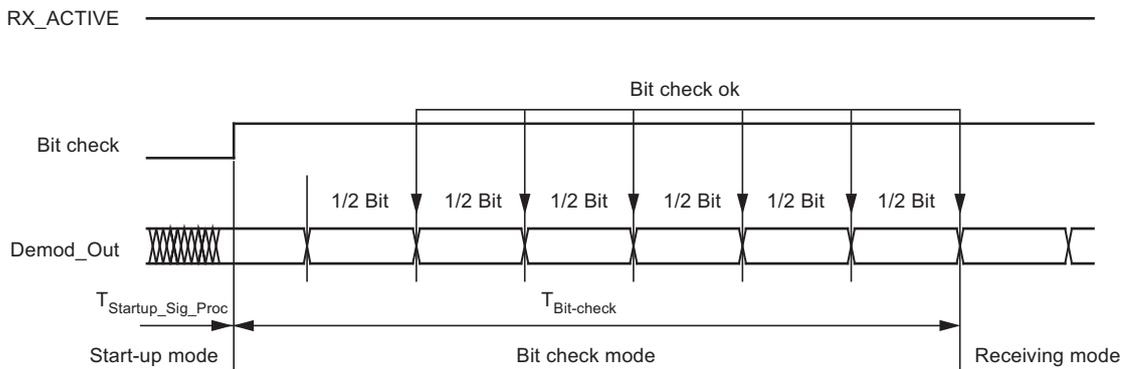
As seen in Figure 9-4, the time window for the bit check is defined by two separate time limits. If the edge-to-edge time  $t_{ee}$  is in between the lower bit-check limit  $T_{\text{Lim\_min}}$  and the upper bit-check limit  $T_{\text{Lim\_max}}$ , the check will be continued. If  $t_{ee}$  is smaller than limit  $T_{\text{Lim\_min}}$  or exceeds  $T_{\text{Lim\_max}}$ , the bit check will be terminated and the transceiver switches to sleep mode.
