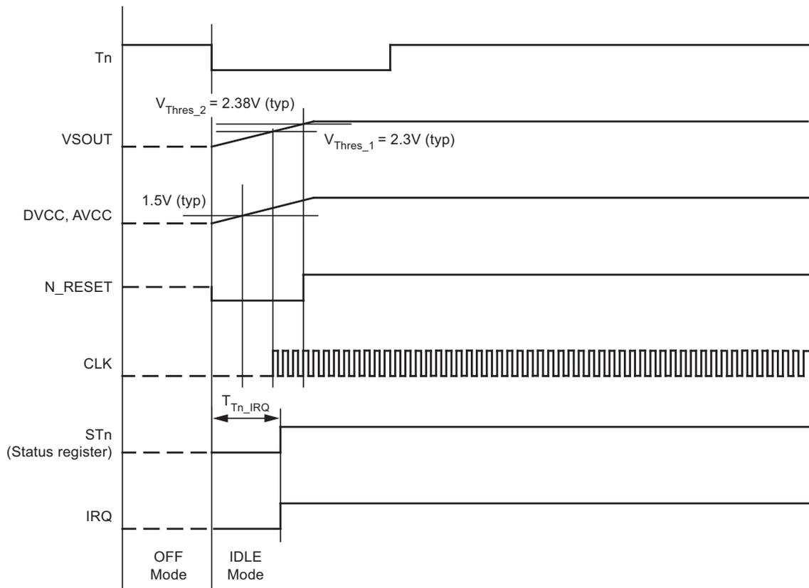
If the transceiver is in any active mode (IDLE, AUX, TX, RX, RX\_Polling), an integrated debounce logic is active. If there is an event on pin Tn a debounce counter is set to 0 ( $T = 0$ ) and started. The status is updated, an interrupt is issued and the debounce counter is stopped after reaching the counter value  $T = 8195 \times T_{DCLK}$ .
