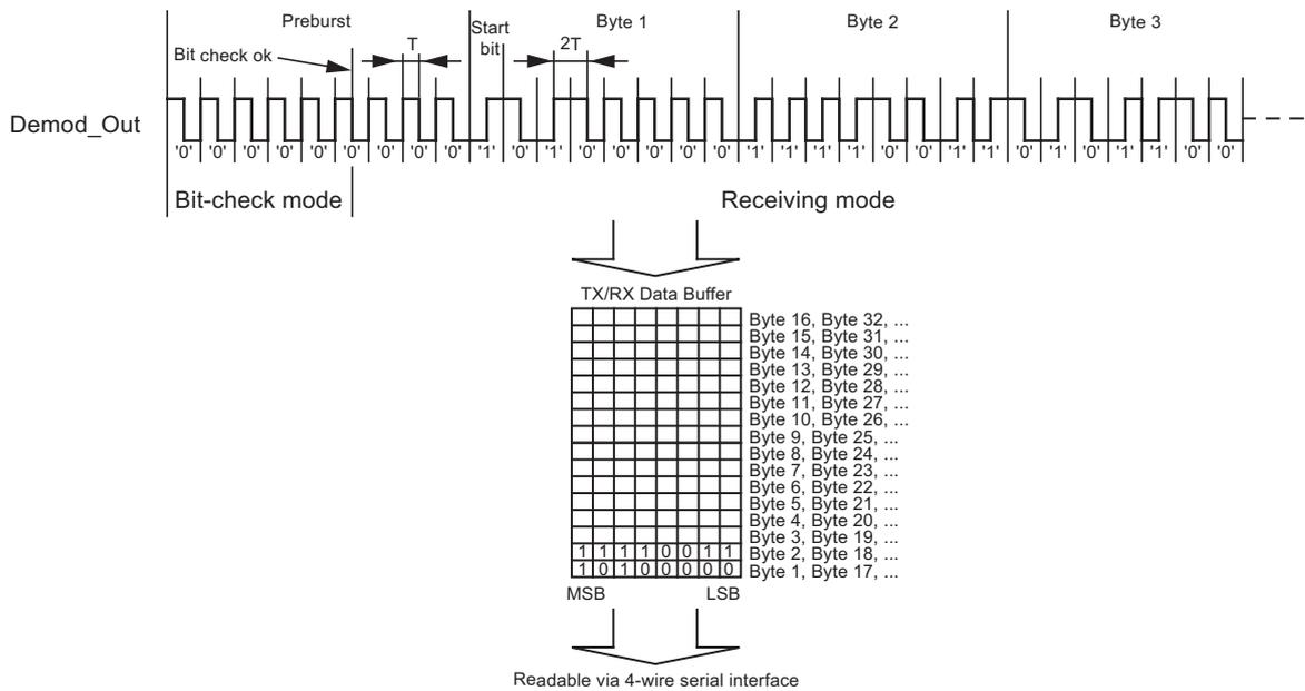
If the TX/RX data buffer control logic detects a bit error, an interrupt is issued and the transceiver is set back to the start-up mode (see Figure 9-1 on page 46, Figure 9-2 on page 47 and Figure 9-10).
