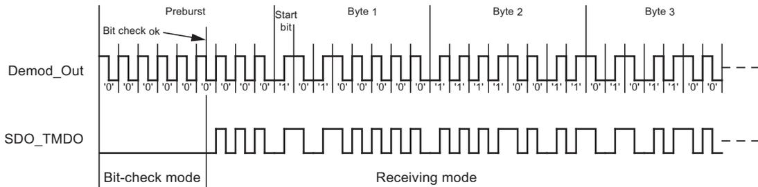
If the transparent mode is inactive (T\_MODE = 0), the received data stream is buffered in the TX/RX data buffer (see Figure 9-9 on page 52). The TX/RX data buffer is only usable for Manchester and Bi-phase coded signals. It is always possible to transfer the data from the data buffer via the 4-wire serial interface to a microcontroller (see Figure 8-1 on page 41).
