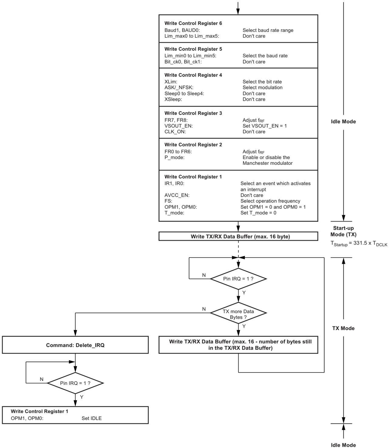
**Figure 9-12. TX Transparent Mode (T\_MODE = 1)**
