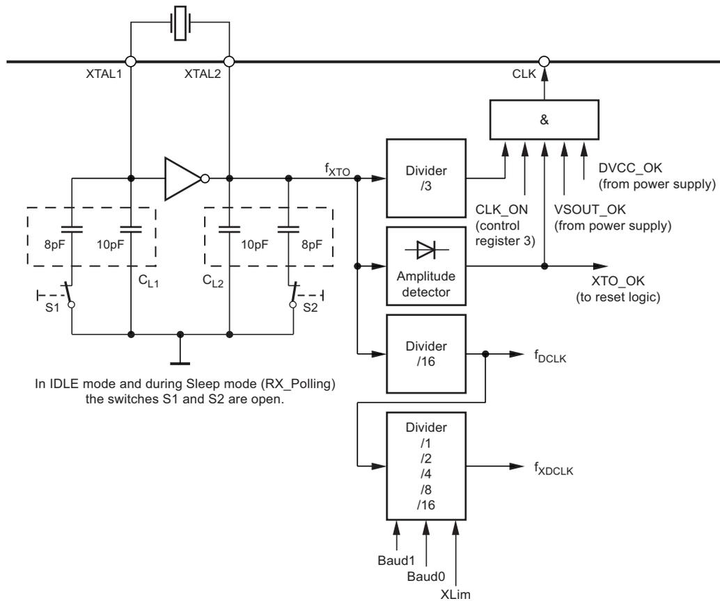
To find the right values used in control registers 2 and 3 (see [Table 7-7 on page 32](#) and [Table 7-10 on page 33](#)), the relationship between  $f_{XTO}$  and the  $f_{RF}$  is shown in [Table 4-1 on page 23](#). To determine the right content, the frequency at pin CLK as well as the output frequency at RF\_OUT in ASK mode can be measured, then the FREQ value can be calculated according to [Table 4-1 on page 23](#) so that  $f_{RF}$  is exactly the desired radio frequency.
