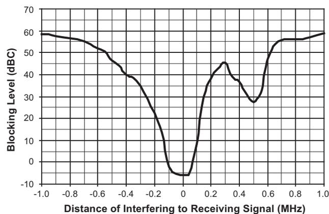
This high blocking performance even makes it possible for some applications using quarter wave whip antennas to use a simple LC band-pass filter instead of a SAW filter in the receiver.
