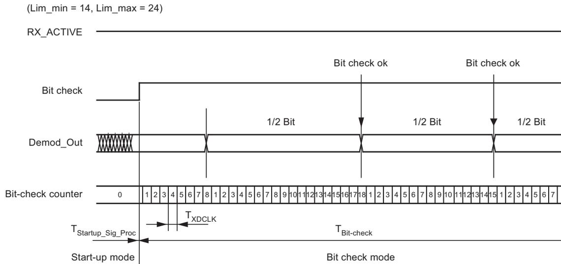
**Figure 9-6. Timing Diagram for Failed Bit Check (Condition  $CV\_Lim < Lim\_min$ )**
