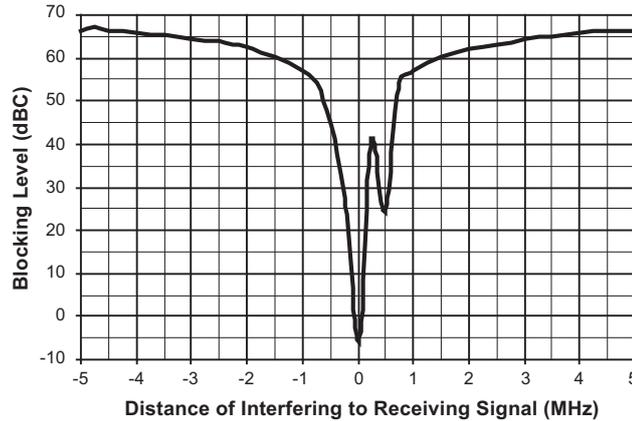
**Figure 3-4. Wide Band 3dB Blocking Characteristic at 433.92MHz**
