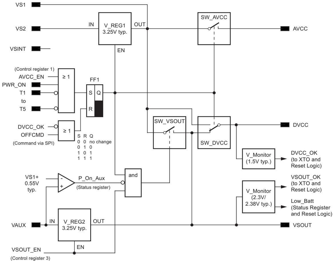
The supply voltage range of the ATA5428 is 2.4V to 3.6V or 4.4V to 6.6V.
