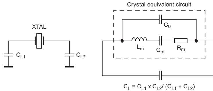
With  $C_m \leq 14\text{fF}$ ,  $C_0 \geq 1.5\text{pF}$ ,  $C_{LN} = 9\text{pF}$  and  $C_L = 7.4\text{pF}$  to  $10.6\text{pF}$ , the pulling amounts to  $P \leq \pm 100\text{ppm}$  and with  $C_m \leq 7\text{fF}$ ,  $C_0 \geq 1.5\text{pF}$ ,  $C_{LN} = 9\text{pF}$  and  $C_L = 7.4\text{pF}$  to  $10.6\text{pF}$ , the pulling is  $P \leq \pm 50\text{ppm}$ .
