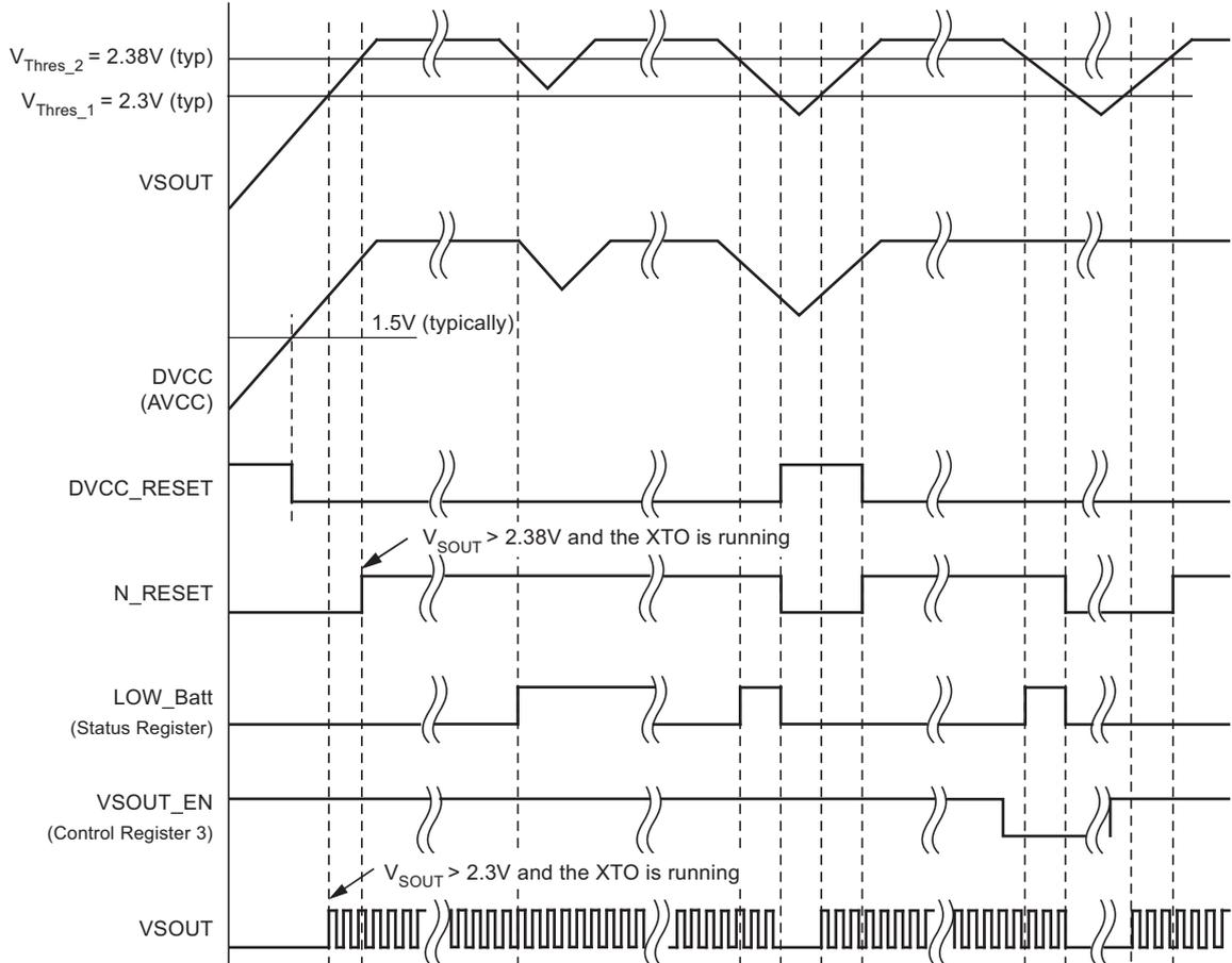
**Figure 5-4. Reset Logic, SR Latch Generates the Hysteresis in the NRESET Signal**
