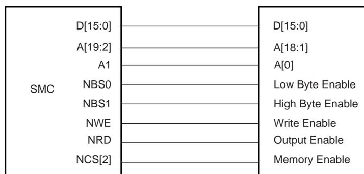
Figure 20-5. Memory Connection for a 32-bit Data Bus
