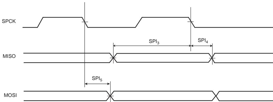
**Figure 38-10. SPI Slave mode with (CPOL = 0 and NCPHA = 1) or (CPOL = 1 and NCPHA = 0)**
