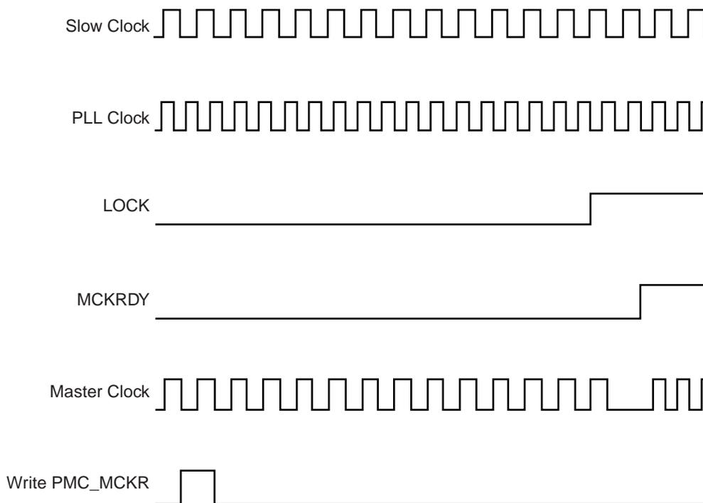
**Figure 24-4. Switch Master Clock from Main Clock to Slow Clock**
