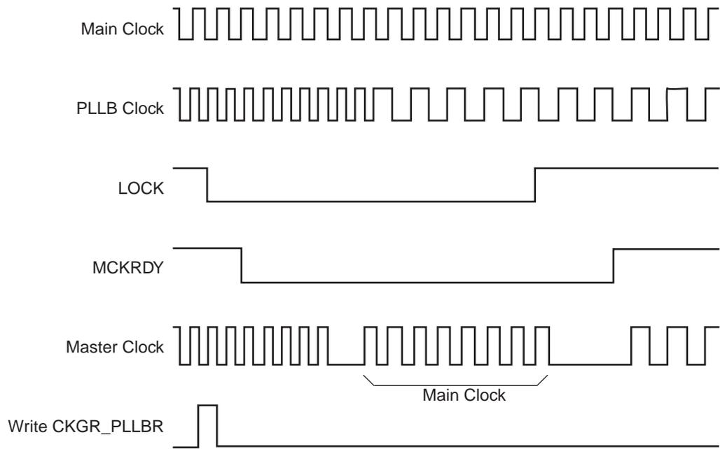
**Figure 24-7. Programmable Clock Output Programming**
