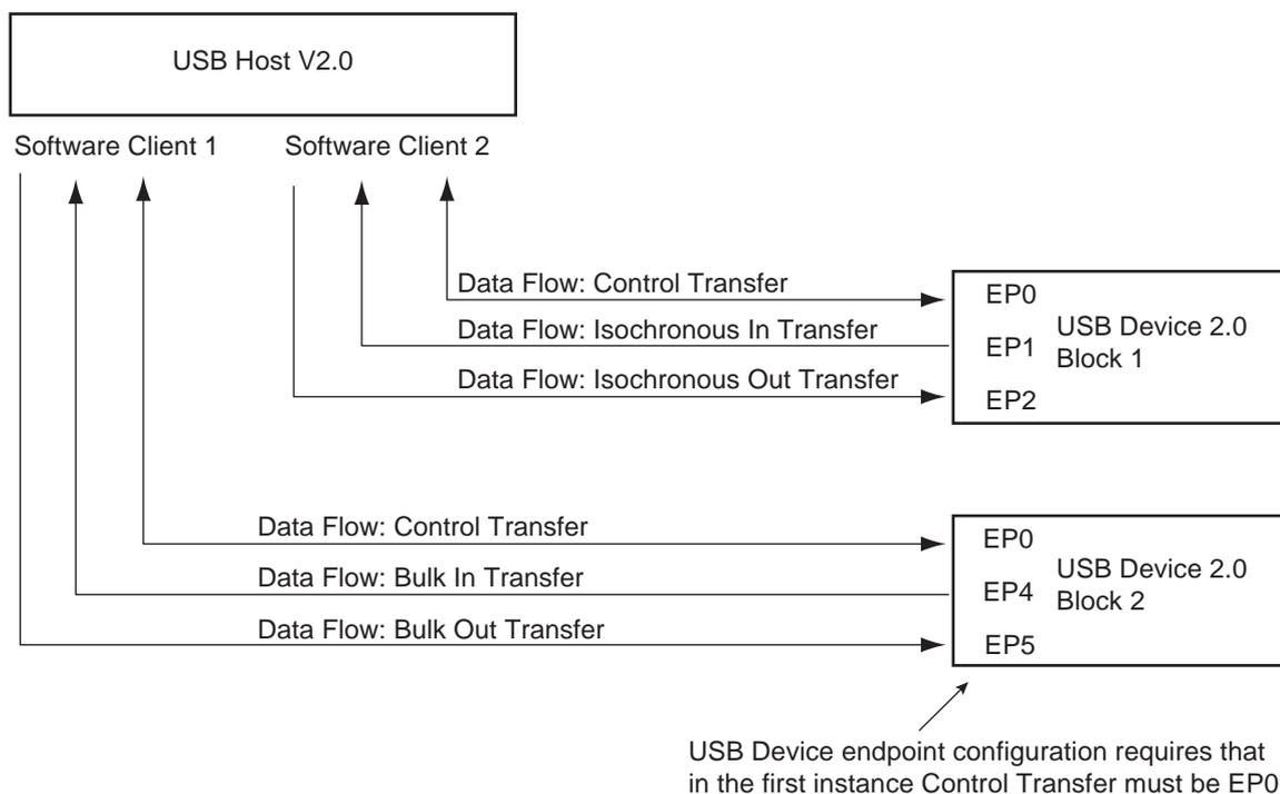
The Control Transfer endpoint EP0 is always used when a USB device is first configured (USB v. 2.0 specifications).
