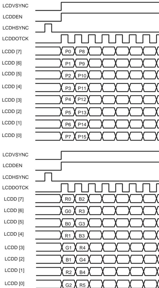
**Figure 37-9. Dual Scan Monochrome and Color 8-bit Panel Timing (First Line Expanded View)**
