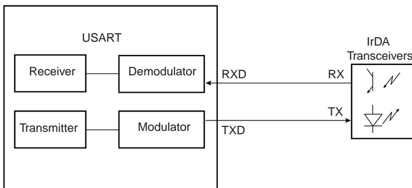
The receiver and the transmitter must be enabled or disabled according to the direction of the transmission to be managed.
