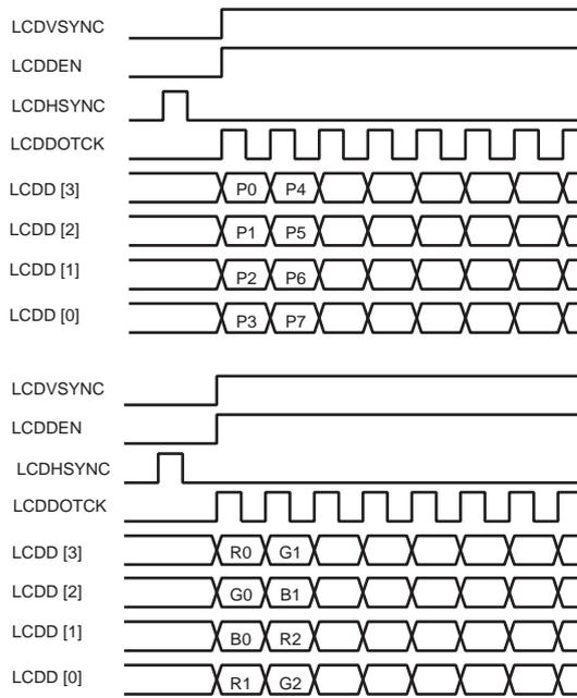
**Figure 37-8. Single Scan Monochrome and Color 8-bit Panel Timing (First Line Expanded View)**
