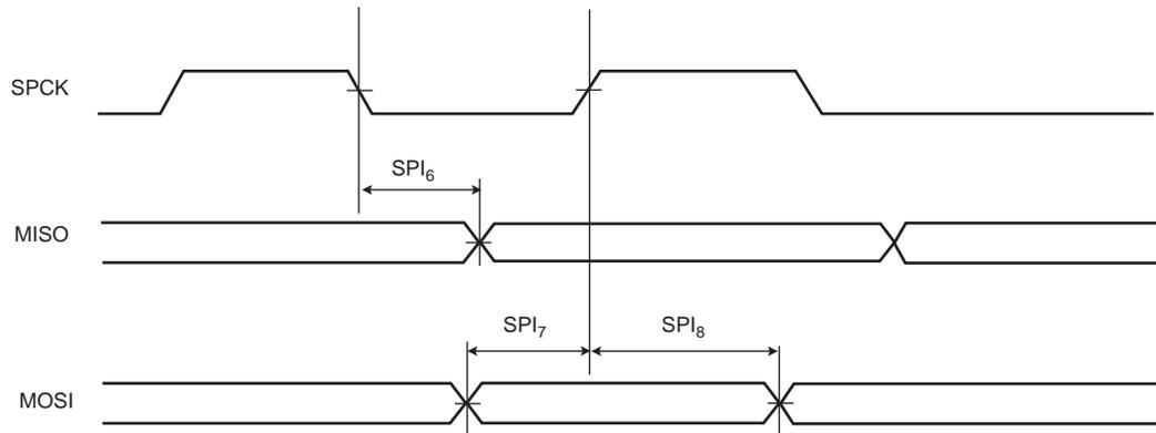
**Figure 38-11. SPI Slave mode with (CPOL = NCPHA = 0) or (CPOL = NCPHA = 1)**
