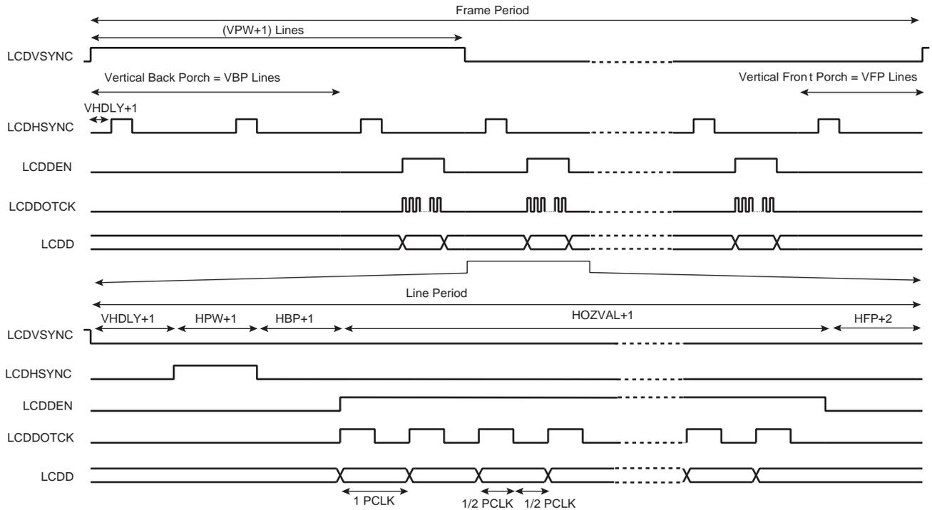
**Figure 37-5. TFT Panel Timing (Line Expanded View), CLKMOD=1**
