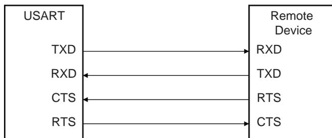
Setting the USART to operate with hardware handshaking is performed by writing the USART\_MODE field in the Mode Register (US\_MR) to the value 0x2.
