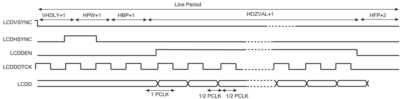
Usually the LCD\_FRM rate is about 70 Hz to 75 Hz. It is given by the following equation:
