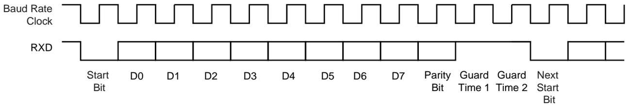
**Figure 31-22. T = 0 Protocol with Parity Error**
