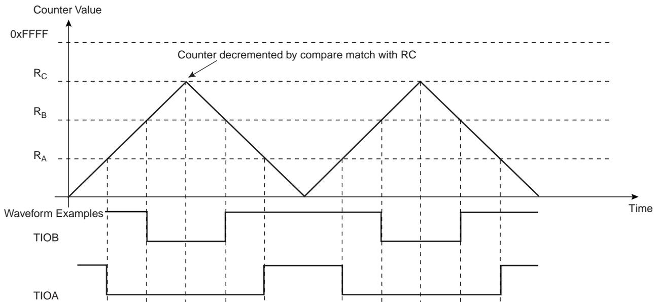
**Figure 33-14. WAVSEL = 11 With Trigger**
