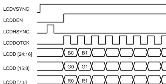
**Figure 37-7. Single Scan Monochrome and Color 4-bit Panel Timing (First Line Expanded View)**
