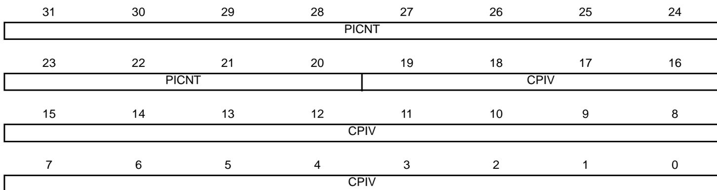
Reading this register clears PITS in PIT\_SR.
