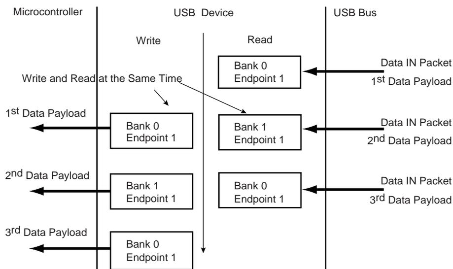
When using a ping-pong endpoint, the following procedures are required to perform Data OUT transactions:
