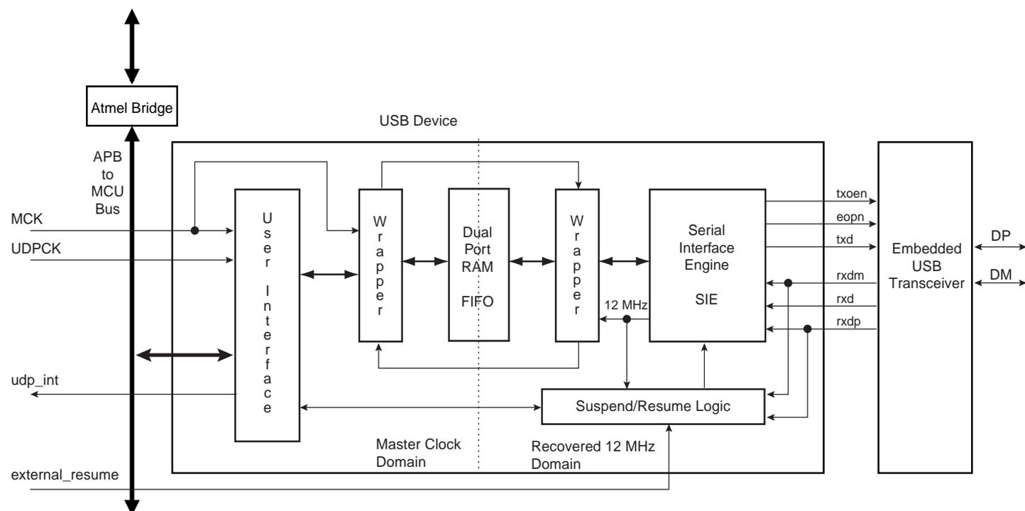
Access to the UDP is via the APB bus interface. Read and write to the data FIFO are done by reading and writing 8-bit values to APB registers.
