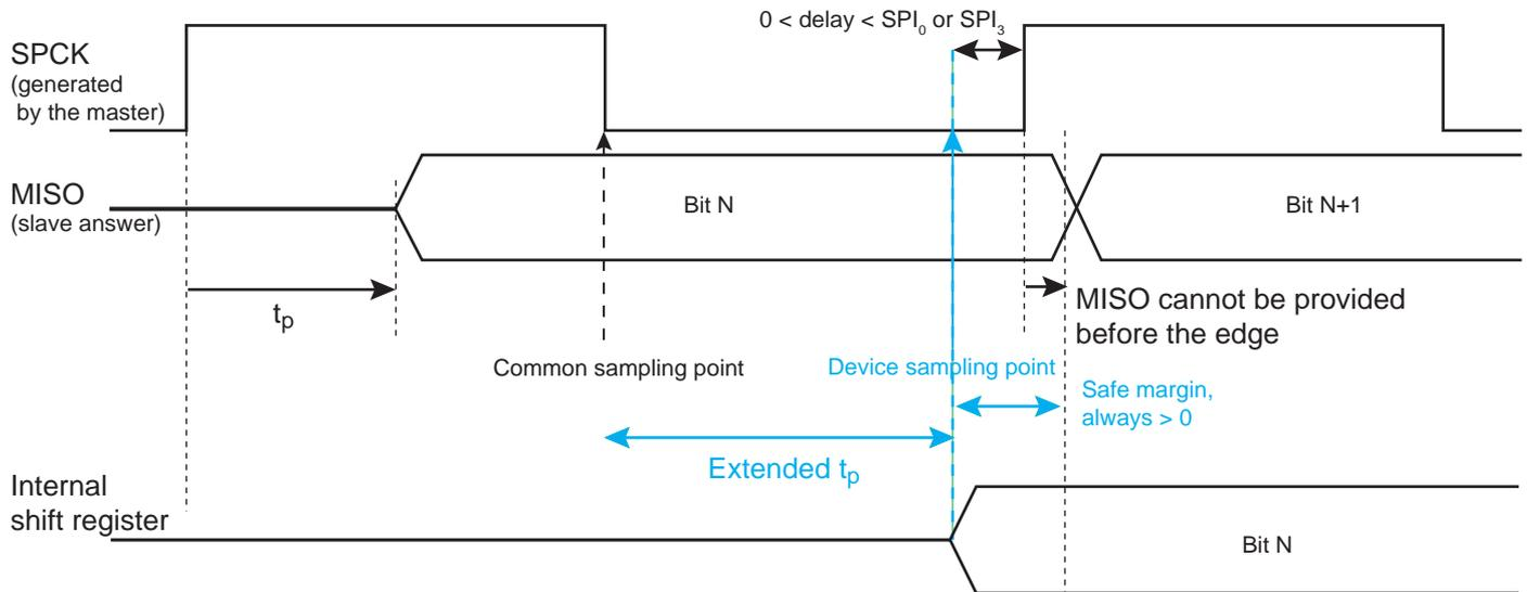
**Figure 38-8. SPI Master mode with (CPOL = 0 and NCPHA = 1) or (CPOL = 1 and NCPHA = 0)**
