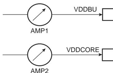
These figures represent the power consumption measured on the power supplies.
