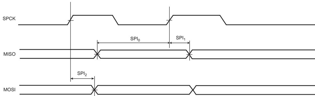
**Figure 38-9. SPI Master mode with (CPOL = NCPHA = 0) or (CPOL = NCPHA = 1)**
