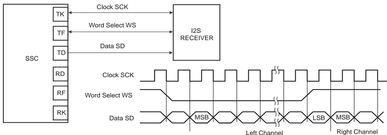
**Figure 32-18. Codec Application Block Diagram**
