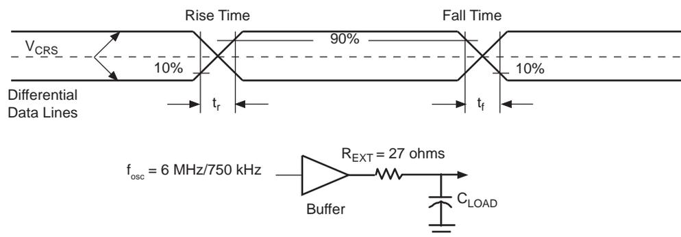
Table 38-24. USB Data Signal Rise and Fall Time Characteristics (Low Speed)
