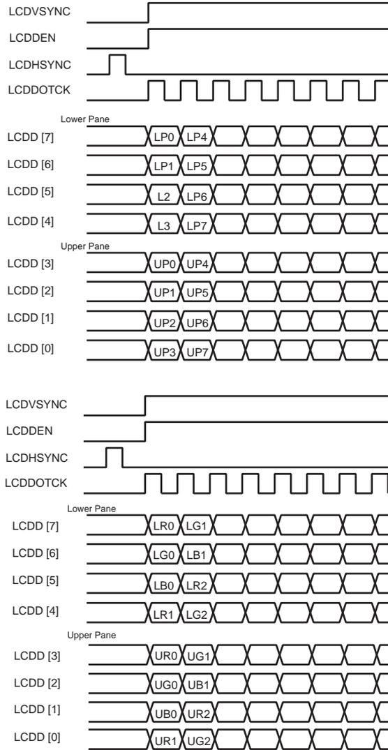
**Figure 37-10. Dual Scan Monochrome and Color 16-bit Panel Timing (First Line Expanded View)**
