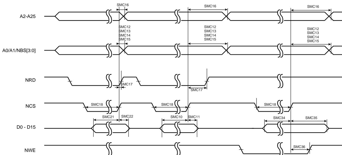
**Figure 38-5. SMC Signals for NRD and NWR Controlled Access**
