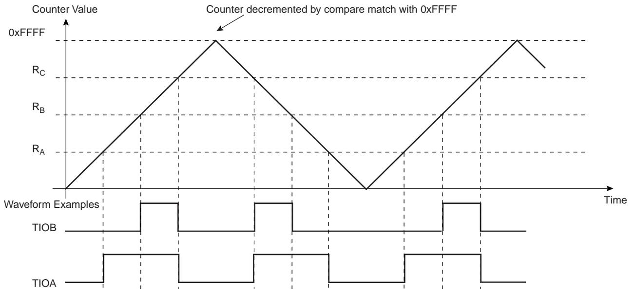
**Figure 33-12. WAVSEL = 01 With Trigger**
