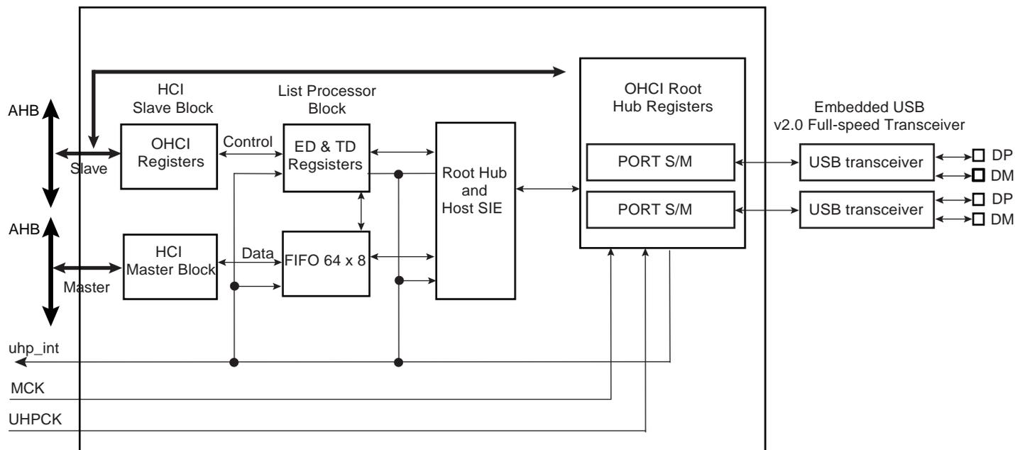
Access to the USB host operational registers is achieved through the AHB bus slave interface. The OpenHCI host controller initializes master DMA transfers through the ASB bus master interface as follows:
