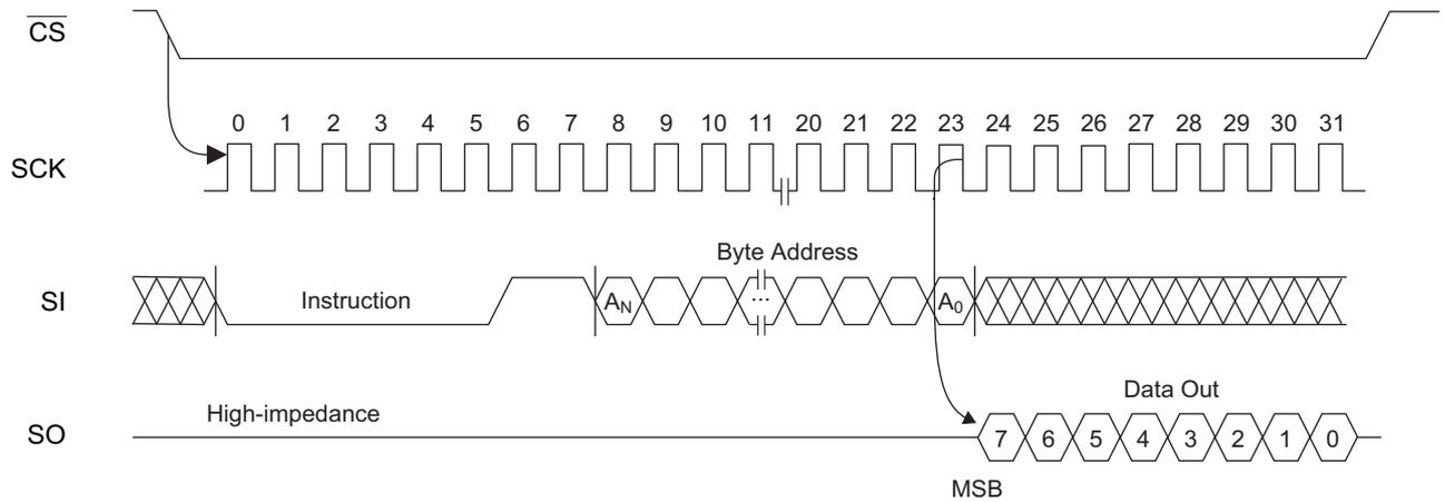
**Figure 7-7. WRITE Timing**
