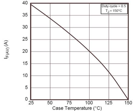
Figure 7. Maximum Average Forward Current vs. Case Temperature
