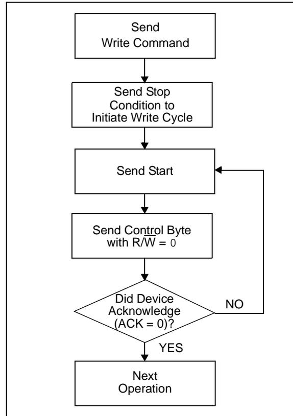
FIGURE 7-2: BYTE WRITE
