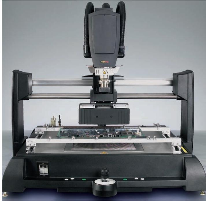
Featured on the APR-5000-XLS Advanced Package Rework System is an innovative Split Vision System, which allows operators to view the opposite corners of a component, including splitting on rectangular components, with the necessary magnification to make its placement and registration fast and accurate.
