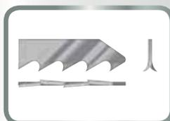
**Teeth ground, offset for clearance gap**
