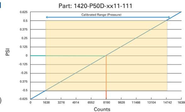
**LP Series - Digital** is a surface mountable pressure sensor package with a compensated digital output suitable for ultra-low pressure sensing applications.
