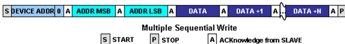
Figure 22 – Avocet 2 Wire Serial Interface Multiple Write
