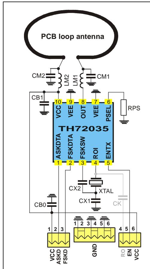
Fig. 6: Circuit diagram with loop antenna matching network
