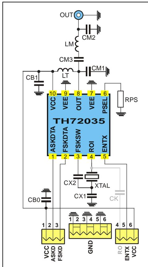
Fig. 7: Circuit diagram with 50 Ω matching network
