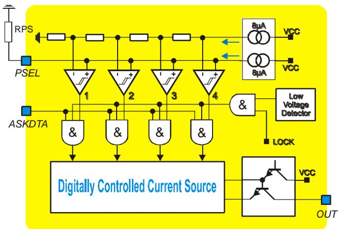
Fig. 4: Block diagram of output power control circuitry
