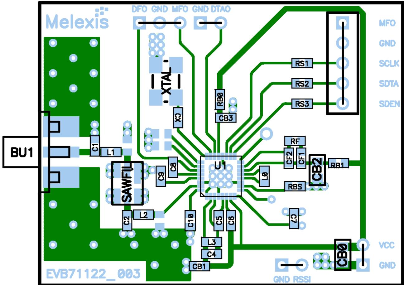
Fig. 7: PCB Top-side view (averaging data slicer option)
