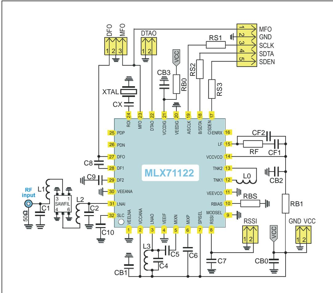
Fig. 6: Application circuit for SPI Mode (averaging data slicer option)
