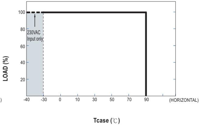
If XLG-200 operates in Constant Power mode with the rated current the maximum workable Ta is 50°C (Typ. 230VAC) or 40°C (typ.110VAC)
