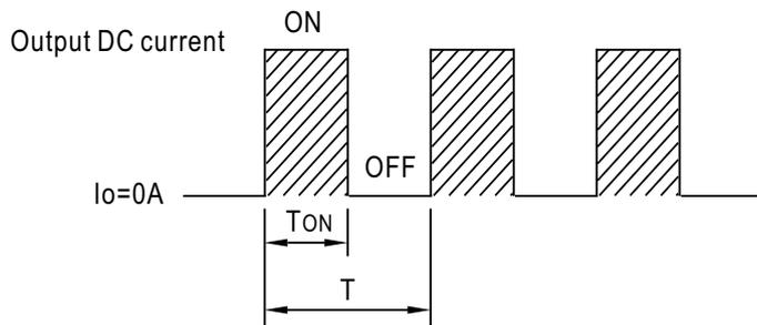
$$\text{Duty cycle(\%)} = \frac{T_{ON}}{T} \times 100\%$$
