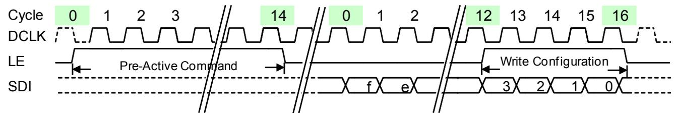
“Write configuration” command is used to program the configuration register of MBI5153. The “Pre-Active” command must be sent in advance. When this command is received, the last 16 bits data before the falling edge of LE will be latched into configuration register, as shown in the above waveform, and MSB bit needs to be sent first.
