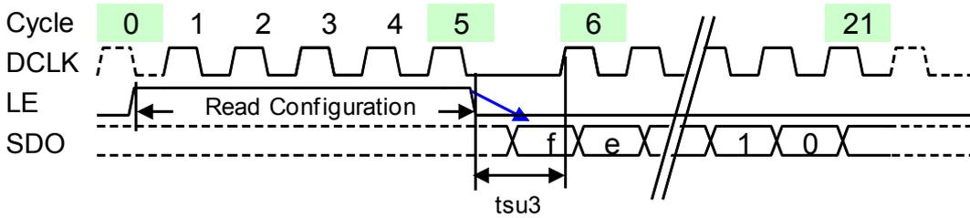
“Read configuration” command is used to read the configuration register of MBI5153. When this command is received, the 16-bit data of configuration register will be shifted out from SDO pin, as shown in the above waveform, and MSB bit will be shifted out first.
