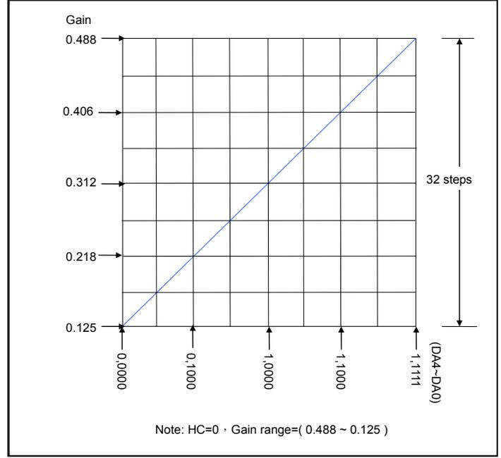
The 6 bits (bit 5~bit 0) of the configuration register set the gain of output current, i.e., G. As total 6-bit in number, i.e., ranging from 6'b000000 to 6'b111111, these bits allow user to set the output current gain up to 64 levels. These bits can be further defined inside configuration register as follows:
