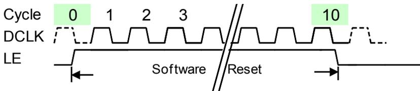
“Software reset” command makes MBI5153 go back to the initial state except configuration register value. After this command is received, the output channels will be turned off and will display again with last gray-scale value after new “Vsync” command is received.
