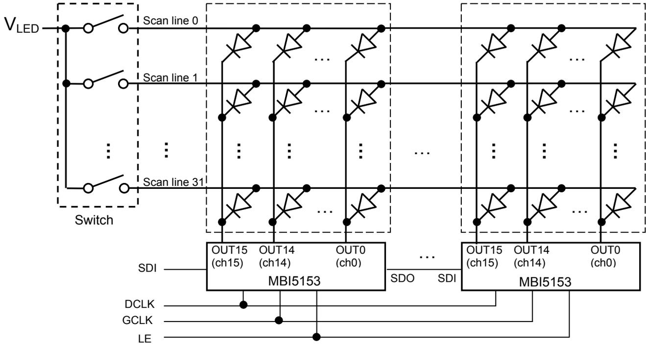
The above figure shows the suggested application structure of scan type scheme with 32 scan lines. The gray-scale data are sent by pin “SDI and SDO” with the commands formed by pin “LE” and “DCLK”. The output ports from 16 channels (OUT0~OUT15) will output the PWM result for each scan line at different time, so there must be one “Switch” to multiplex for each scan line. The switching sequence and method and the command usage will be described in the application note.
