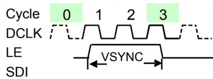
“VSYNC” command is used to update frame data on output channels ( $\overline{OUTC}$ ~ $\overline{OUT15}$ ). There are some timing limitations between signal “LE” and “GCLK”; and please refer to the section of “Vsync Command Operation” for details.
