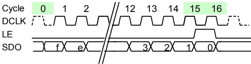
Data Latch command is used to latch the 16-bit shift register from SDI to internal SRAM buffer. When this command is received, the last 16 bits data before the falling edge of LE will be latched into SRAM, as shown in the above waveform, and MSB bit needs to be sent first.
