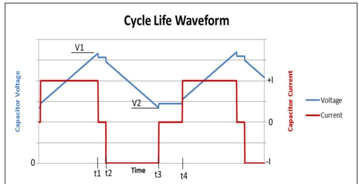
$V1 = V_{rated}$        $t2 - t1 = 5 \text{ seconds (I=0)}$
