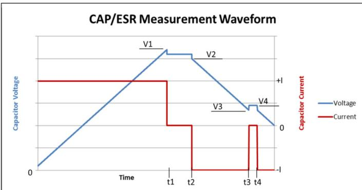
$V1 = V_{rated}$        $t2 - t1 = 15 \text{ seconds}$        $\text{Capacitance} = I \times (t3 - t2) / (V2 - V3)$
