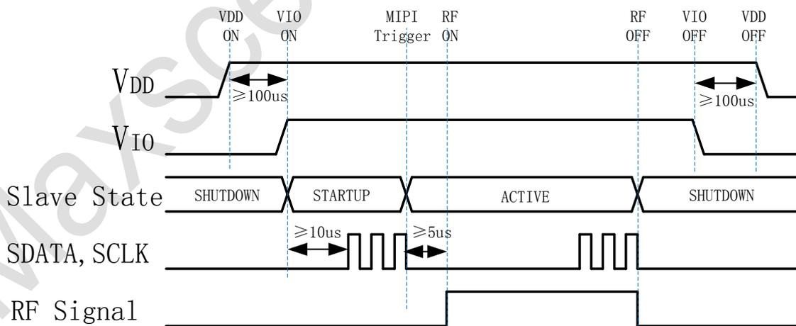
**Note:** V<sub>IO</sub> can be applied to the device before V<sub>DD</sub> or removed after V<sub>DD</sub>.
