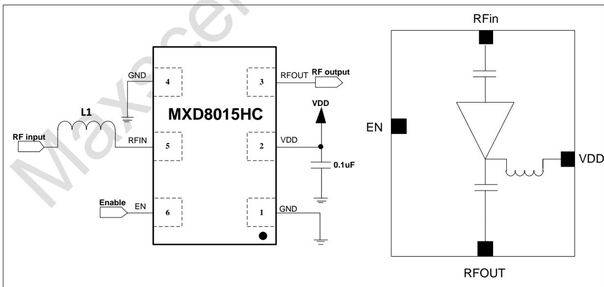
Figure 1 MXD8015HC application circuit
