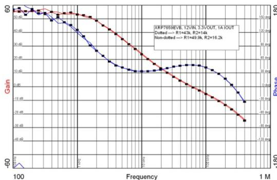
Fig. 18: Gain and Phase Margin Plots of XRP7659EVB
