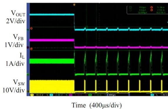
Fig. 14: Onset of Short-circuit Protection
