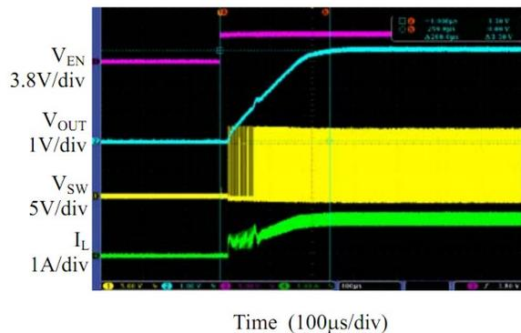
Fig. 12: Enable Turn-on Characteristic
