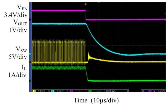
Fig. 13: Enable Turn-off Characteristic
