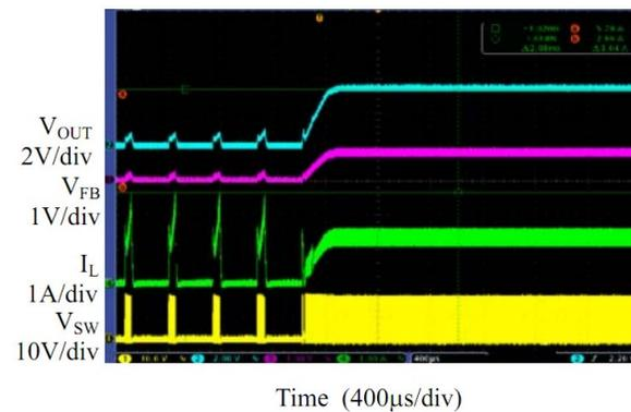
Fig. 15: Short-circuit recovery
