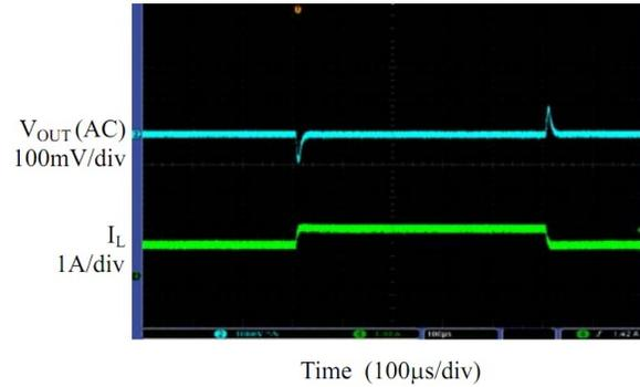
Fig. 11: Load Step Transient,  $I_{OUT}=1A$  to 1.5A
