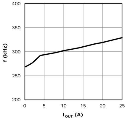
Fig. 22: frequency versus I<sub>OUT</sub>, Forced CCM
