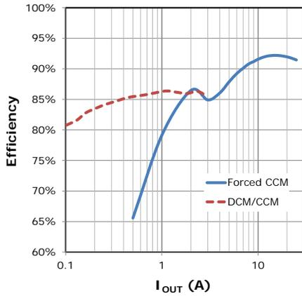
Fig. 16: Efficiency, 12V<sub>IN</sub>, 2.5V<sub>OUT</sub>, 1uH, 300kHz
