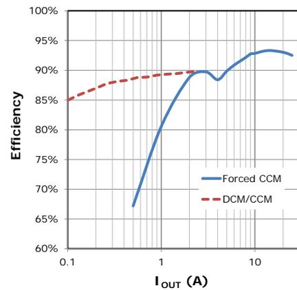
Fig. 15: Efficiency,  $12V_{IN}$ ,  $3.3V_{OUT}$ ,  $1\mu H$ ,  $300kHz$
