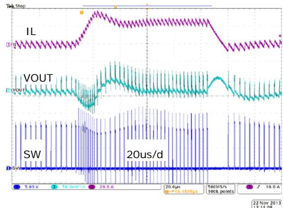
Fig. 27: Load step, Forced CCM, 0A-25A-0A
