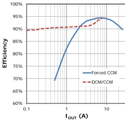
Fig. 12: Efficiency,  $5V_{IN}$ ,  $1.8V_{OUT}$ ,  $0.47\mu H$ ,  $300kHz$
