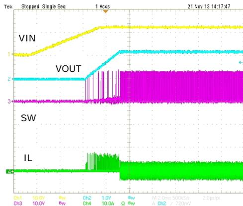
Fig. 8: Powerup, Forced CCM,  $I_{OUT} = 0A$
