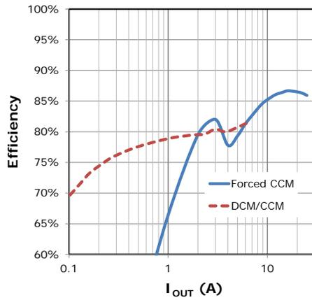
Fig. 18: Efficiency, 12V<sub>IN</sub>, 1.2V<sub>OUT</sub>, 0.47uH, 300kHz
