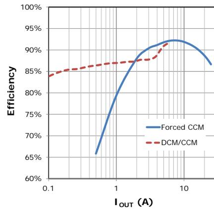
Fig. 13: Efficiency,  $5V_{IN}$ ,  $1.2V_{OUT}$ ,  $0.47\mu H$ ,  $300kHz$
