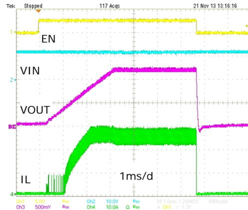
Fig. 20: Enable turn on/turn off, 12V<sub>IN</sub>, 1.2V<sub>OUT</sub>, 25A
