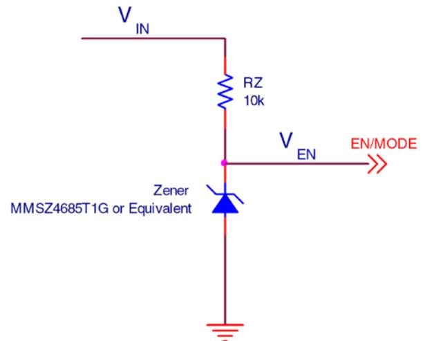
Figure 29. Selecting DCM/CCM by deriving EN/MODE from V<sub>IN</sub>
