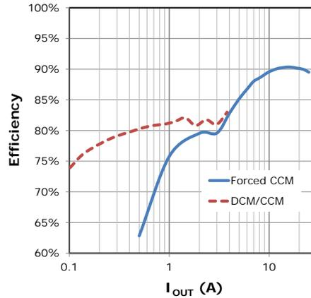
Fig. 17: Efficiency, 12V<sub>IN</sub>, 1.8V<sub>OUT</sub>, 1uH, 300kHz
