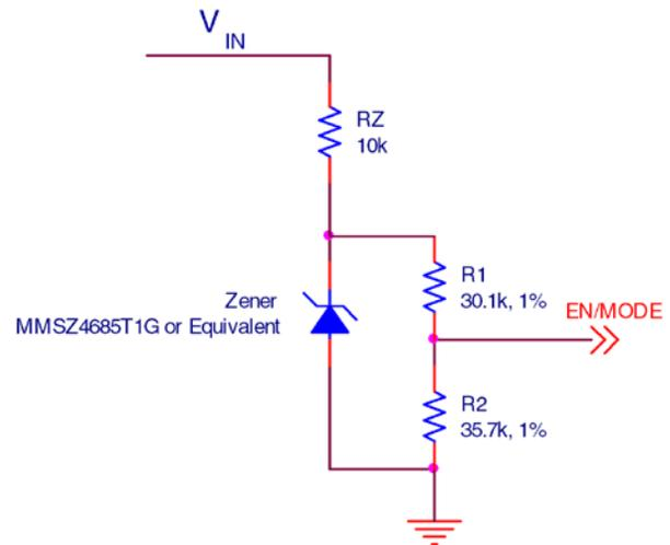
Figure 28. Selecting Forced CCM by deriving EN/MODE from V<sub>IN</sub>
