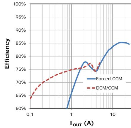
Fig. 19: Efficiency, 12V<sub>IN</sub>, 1.0V<sub>OUT</sub>, 0.47uH, 300kHz
