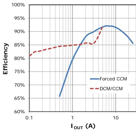
Fig. 14: Efficiency,  $5V_{IN}$ ,  $1.0V_{OUT}$ ,  $0.47\mu H$ ,  $300kHz$
