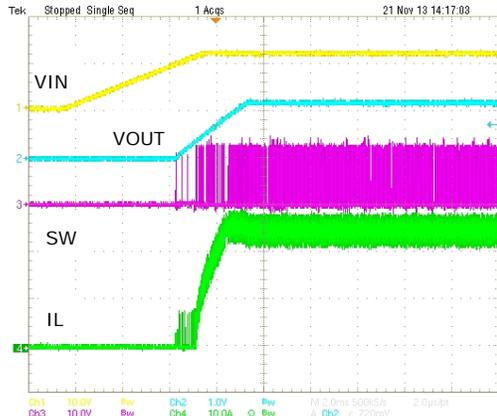
Fig. 9: Powerup, Forced CCM,  $I_{OUT} = 25A$
