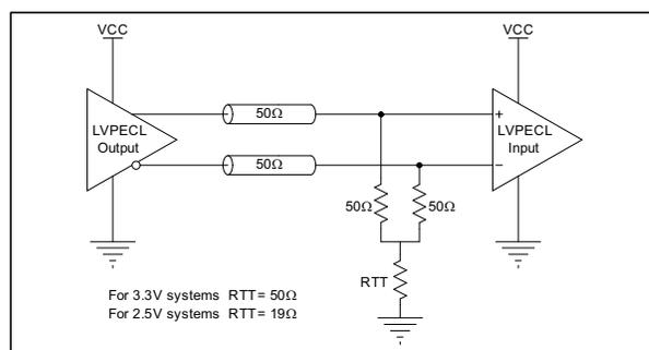
Figure 7: XR81111 Alternate LVPECL Output Termination Using Y-termination
