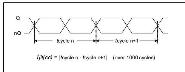
Figure 8: Cycle-to-Cycle Jitter
