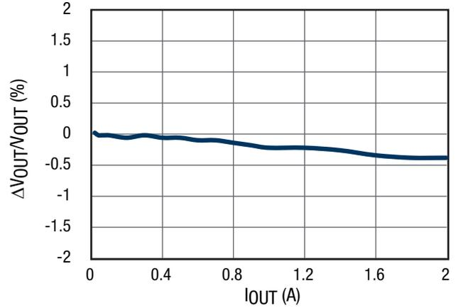
Figure 5. Load Regulation Channel 2,  $5V_{IN}$ ,  $1.8V_{OUT}$
