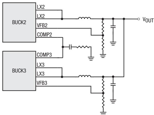
Figure 31. Parallel Operation
