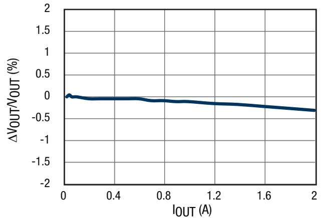
Figure 3. Load Regulation Channel 1,  $5V_{IN}$ ,  $3.3V_{OUT}$
