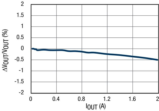
Figure 2. Load Regulation Channel 1,  $12V_{IN}$ ,  $3.3V_{OUT}$
