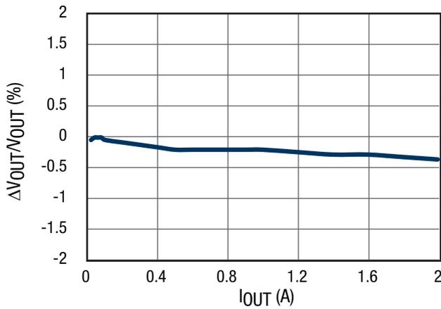
Figure 4. Load Regulation Channel 2,  $12V_{IN}$ ,  $1.8V_{OUT}$
