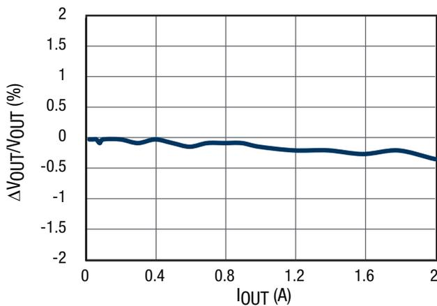
Figure 6. Load Regulation Channel 3,  $12V_{IN}$ ,  $1.2V_{OUT}$
