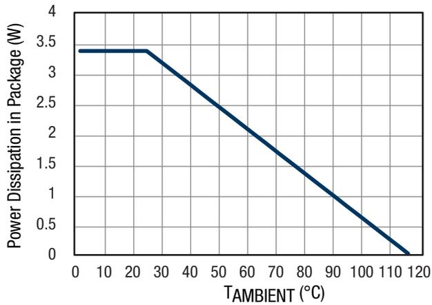
Figure 20. Package Thermal Derating
