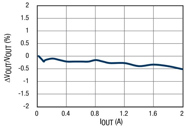
Figure 7. Load Regulation Channel 3,  $5V_{IN}$ ,  $1.2V_{OUT}$
