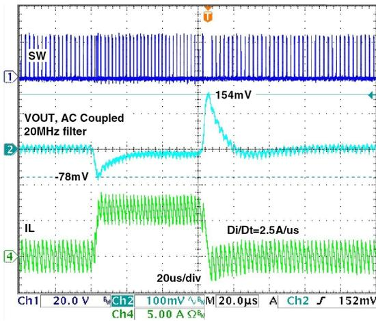
Figure 3: Load Step, Forced CCM, 0A - 6.5A - 0A
