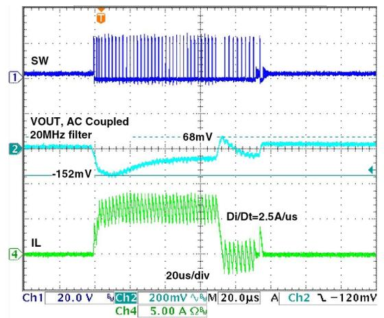
Figure 4: Load Step, DCM / CCM, 0A - 6.5A - 0A
