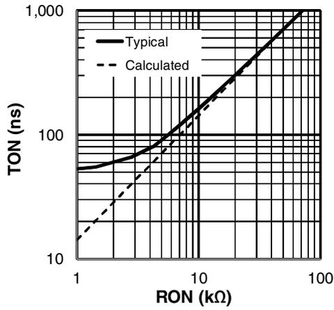
Figure 7: TON versus RON,  $V_{IN} = 24V$
