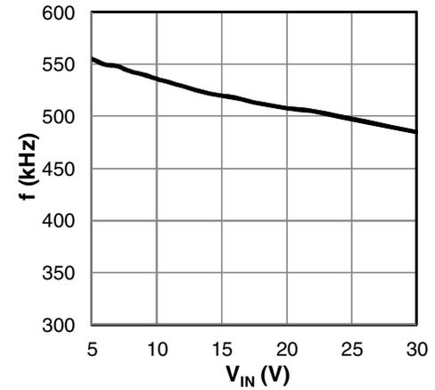
Figure 10: Frequency versus  $V_{IN}$ ,  $I_{OUT} = 10A$
