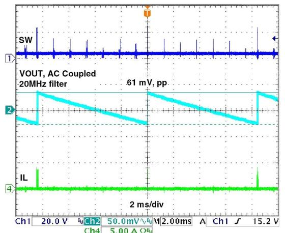
Figure 6: Steady State, DCM,  $V_{OUT,ripple} = 61mV$ ,  $I_{OUT} = 0A$
