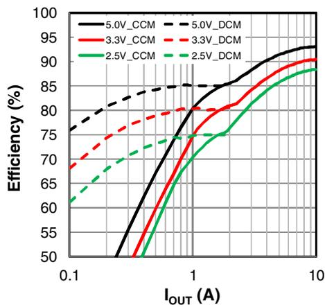
**Figure 17: Efficiency, V<sub>IN</sub> = 24V, f = 500kHz**
