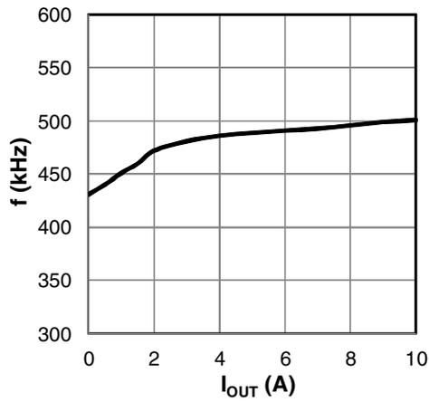
Figure 9: Frequency versus  $I_{OUT}$ ,  $V_{IN} = 24V$
