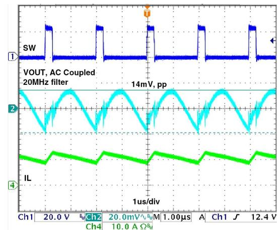
Figure 5: Steady State,  $V_{OUT,ripple} = 14mV$ ,  $I_{OUT} = 10A$
