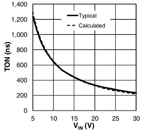
Figure 8: TON versus  $V_{IN}$ ,  $R_{ON} = 19.1k\Omega$
