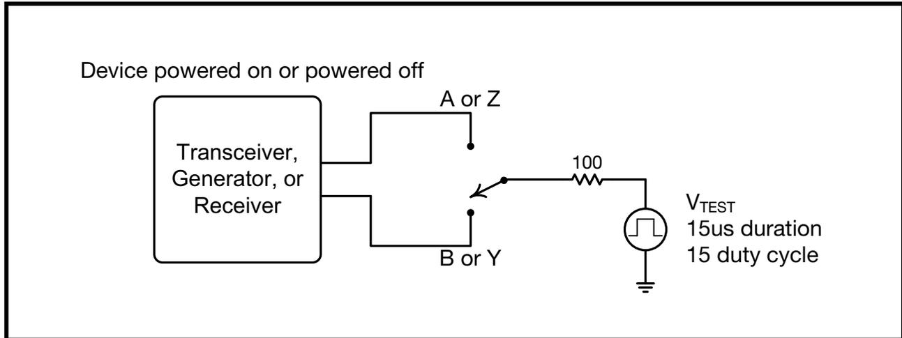
FIGURE 6. DRIVER PROPAGATION DELAY TEST CIRCUIT & TIMING DIAGRAM
