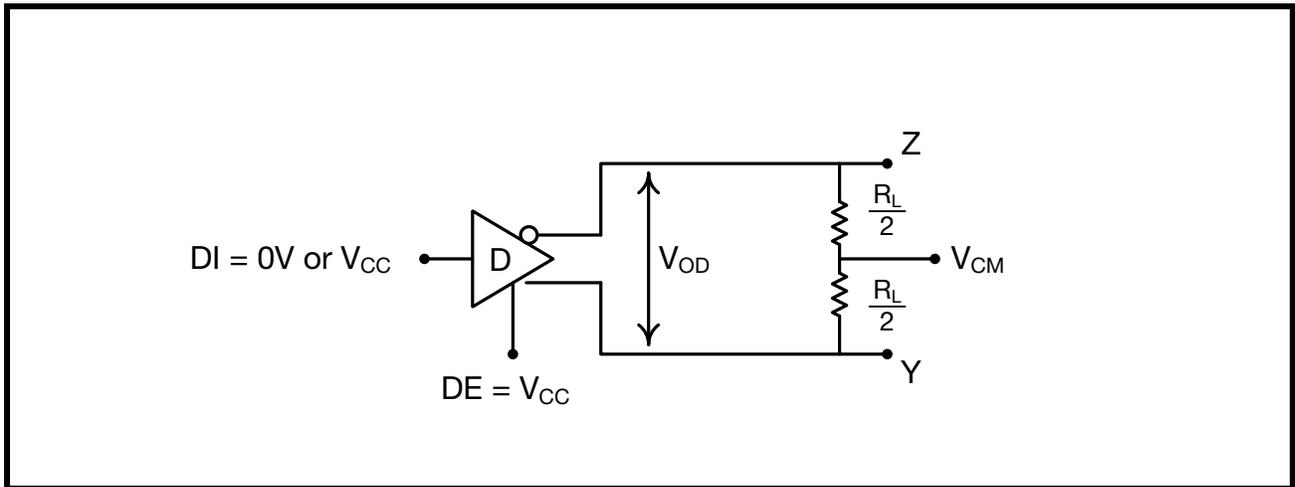
**FIGURE 3. DIFFERENTIAL DRIVER OUTPUT VOLTAGE OVER COMMON MODE**
