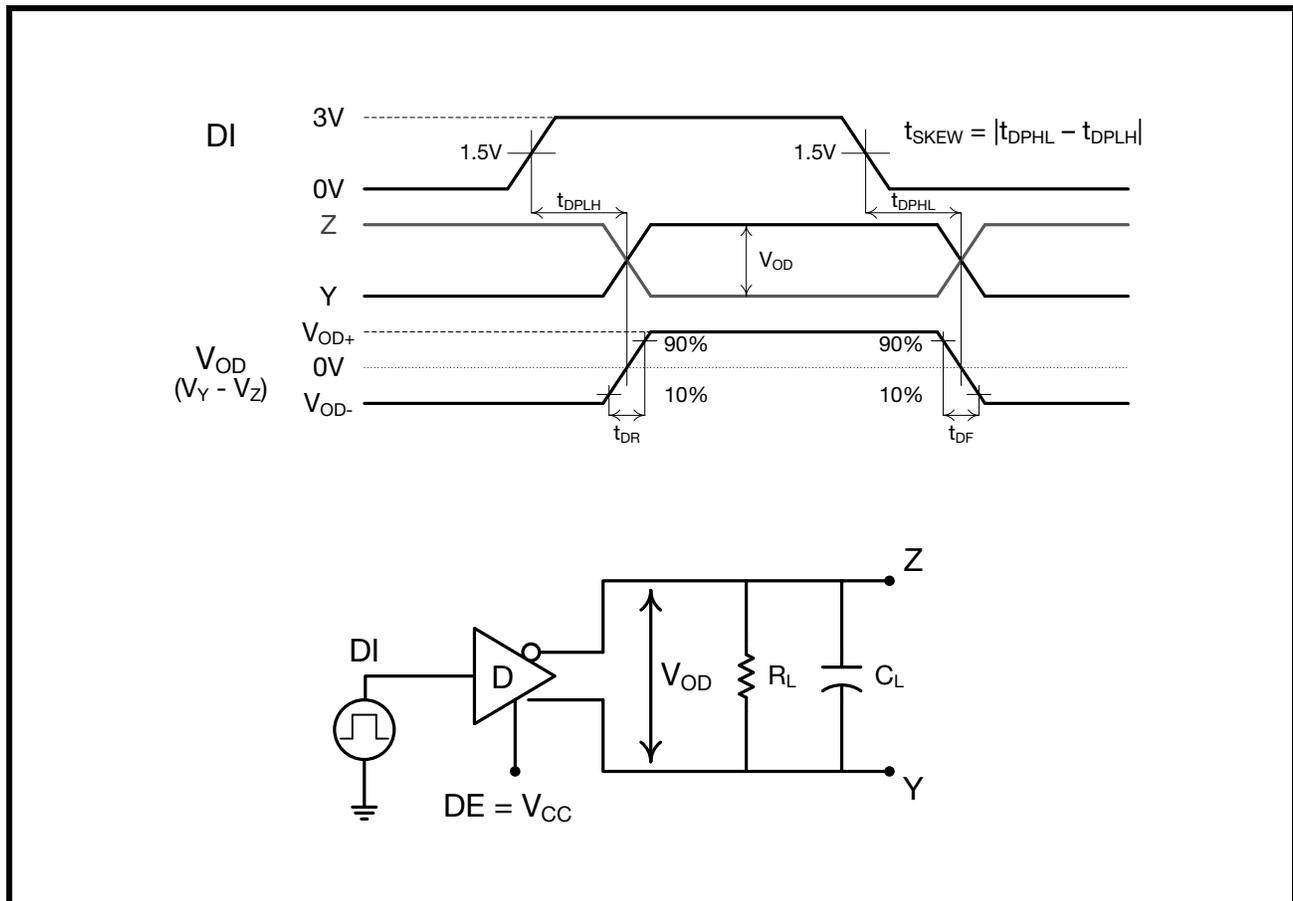
**FIGURE 7. DRIVER ENABLE AND DISABLE TIMING TEST CIRCUITS & TIMING DIAGRAMS**
