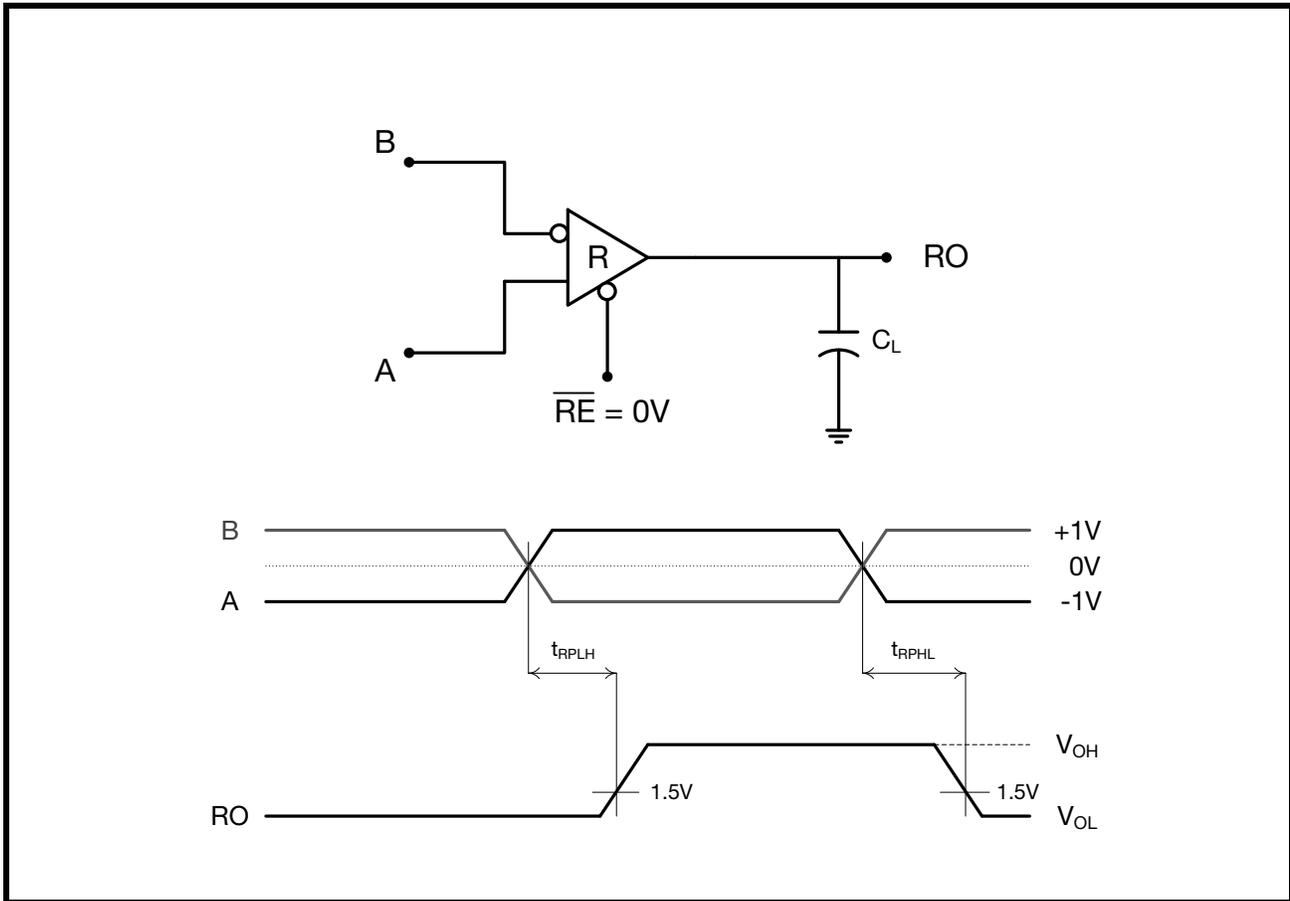
**FIGURE 9. RECEIVER ENABLE AND DISABLE TEST CIRCUITS & TIMING DIAGRAMS**
