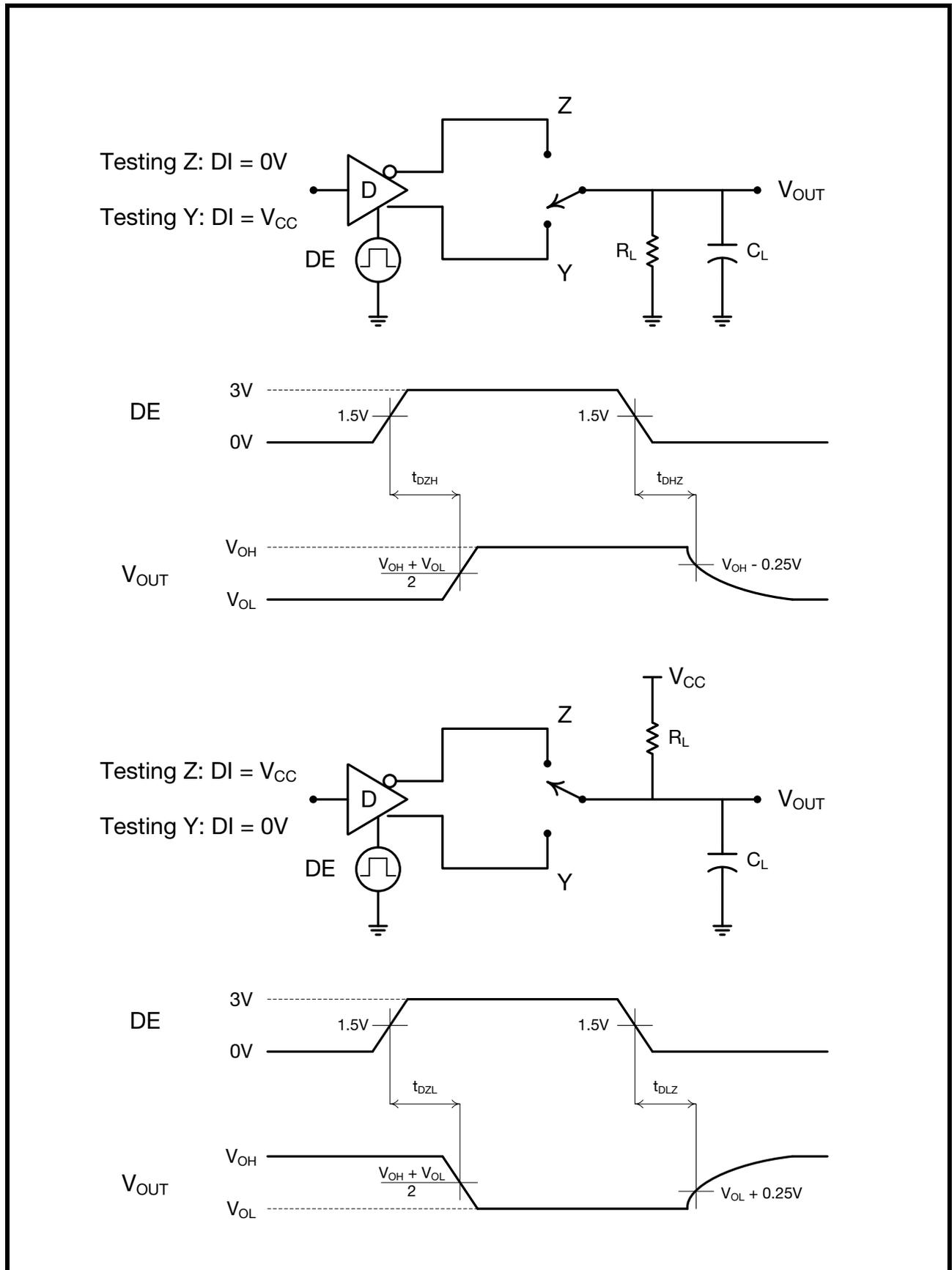
FIGURE 8. RECEIVER PROPAGATION DELAY TEST CIRCUIT & TIMING DIAGRAM
