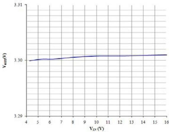
**Figure 6: Line Regulation:  $I_{OUT} = 10mA$ ,  $V_{OUT} = 3.3V$**
