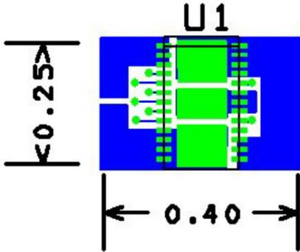
Fig. 15: Minimum Footprint = 0.10in<sup>2</sup>
