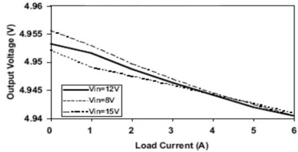
Fig. 4: Output Voltage versus Output Current
