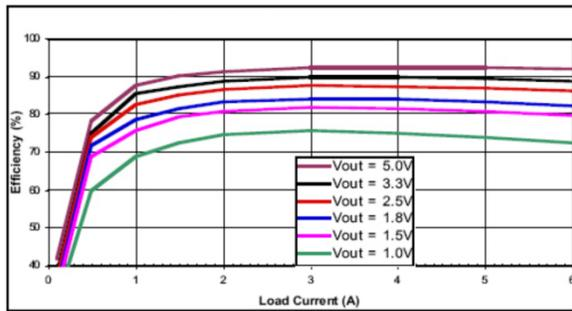
Fig. 9: Efficiency versus Output Current
