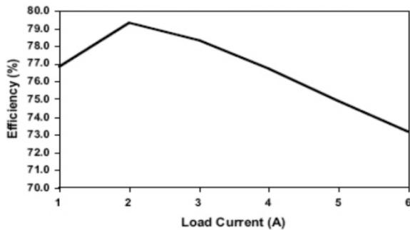
Fig. 7: Efficiency versus Output Current
