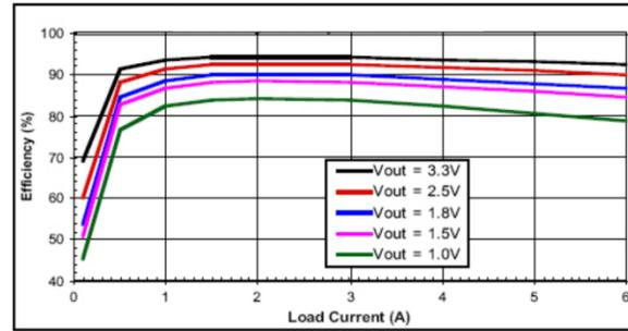
Fig. 10: Efficiency versus Output Current
