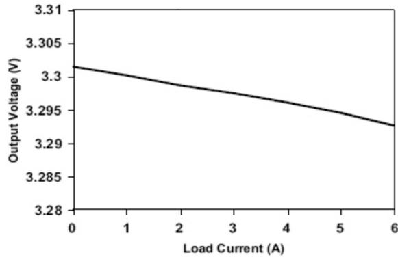
Fig. 6: Output Voltage versus Output Current
