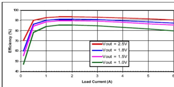
Fig. 11: Efficiency versus Output Current
