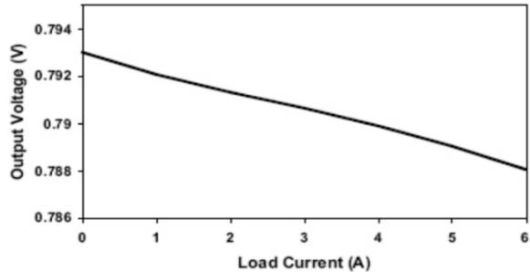
Fig. 8: Output Voltage versus Output Current
