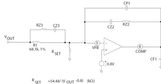
Fig. 14: Type III Error Amplifier Compensation Circuit
