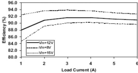
Fig. 3: Efficiency versus Output Current
