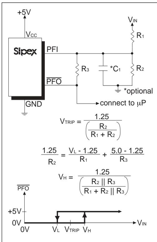
Figure 18. Adding Hysteresis to the POWER-FAIL Comparator
