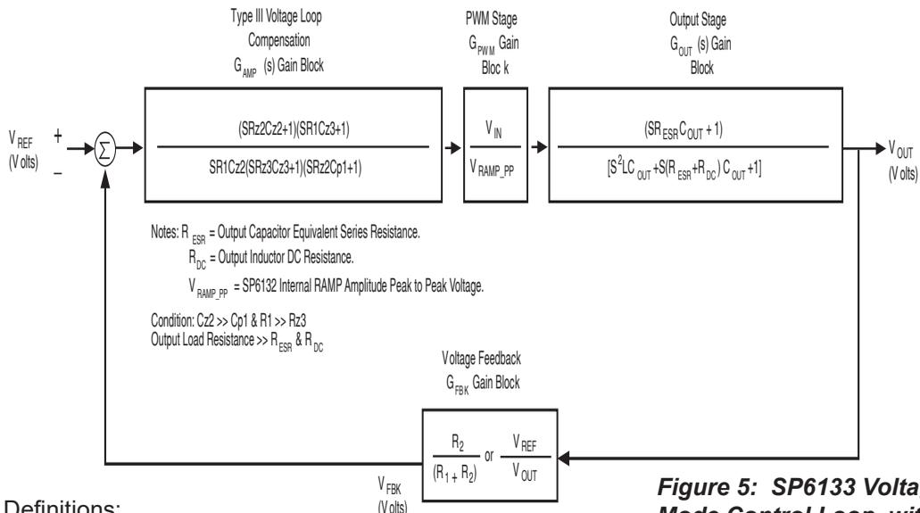
**Figure 5: SP6133 Voltage Mode Control Loop with Loop Dynamic**
