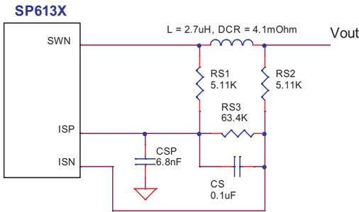
**Figure 2- Over-current detection circuit for  $I_{max} > 60mV / DCR$**
