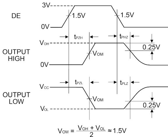
**Figure 13: Driver Enable and Disable Timing Waveforms**
