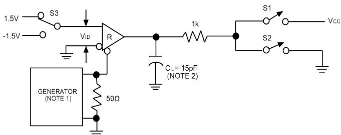
**Figure 9: Receiver Enable and Disable Timing Circuit**
