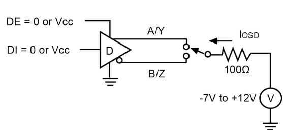
**Figure 10: Driver Short Circuit Current Limit Test**
