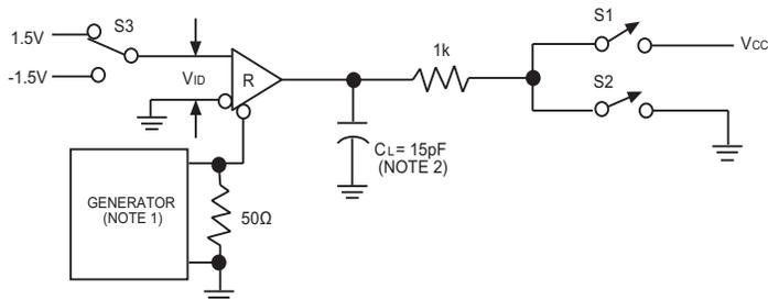
Figure 7: Receiver Enable and Disable Timing Circuit
