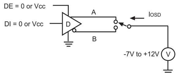
Figure 8: Driver Short Circuit Current Limit Test
