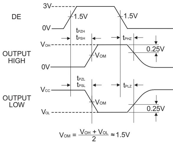
Figure 11: Driver Enable and Disable Timing Waveforms
