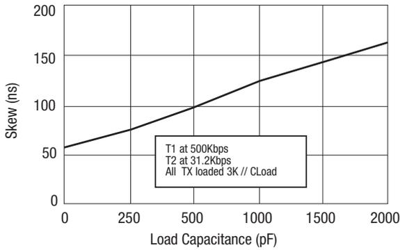
**Figure 1: Transmitter Skew vs. Load Capacitance**
