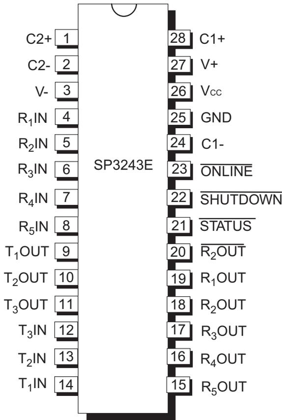
**Figure 8: SP3243E Pinout (Top View) SSOP / TSSOP**
