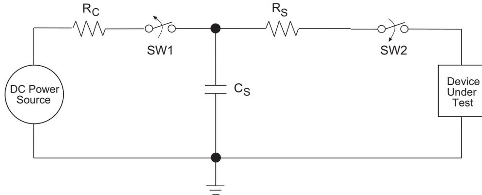
**Figure 25: ESD Test Circuit for Human Body Model**
