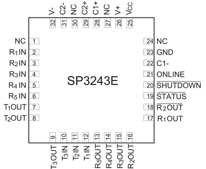
**Figure 9: SP3243E Pinout (Top View) QFN32**
