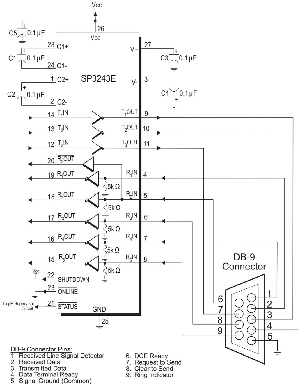
**Figure 22: Attaching SP3243E to a DB-9 Connector**
