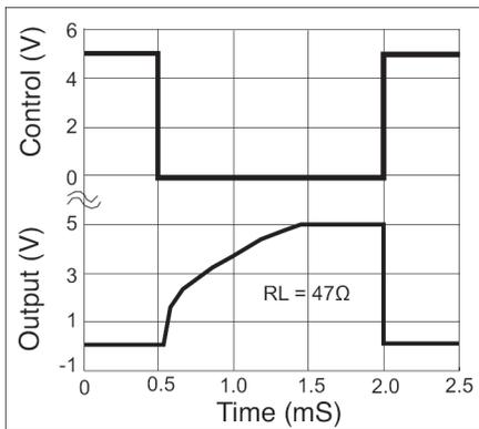
Fig. 12: Turn-on/Turn-off Characteristics
