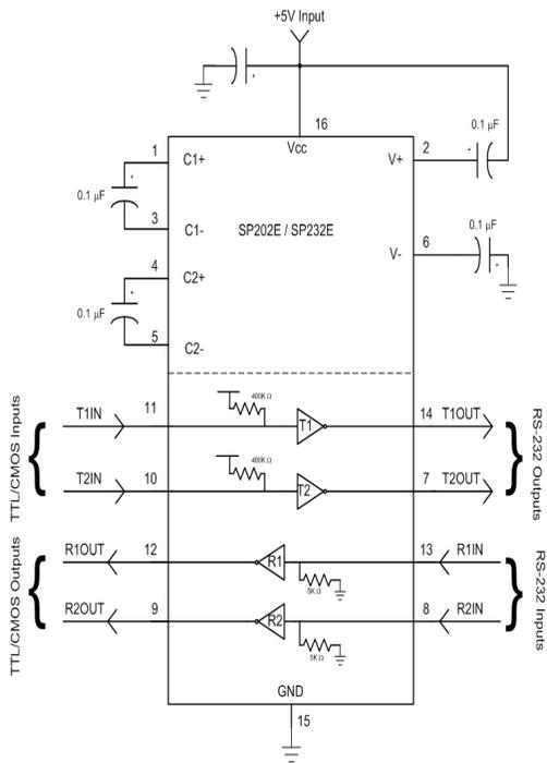
Figure 7, SP202E and SP232E Typical Application circuit
