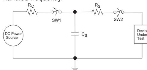
Figure 2. ESD test circuit for Human Body Model
