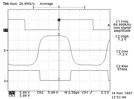
**Figure 3: SP208E Transmitter Output @ 120kbps**
