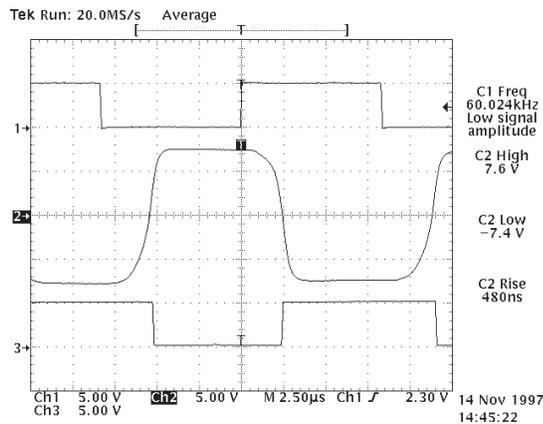
**Figure 2: SP208E Transmitter Output @ 120kbps**
