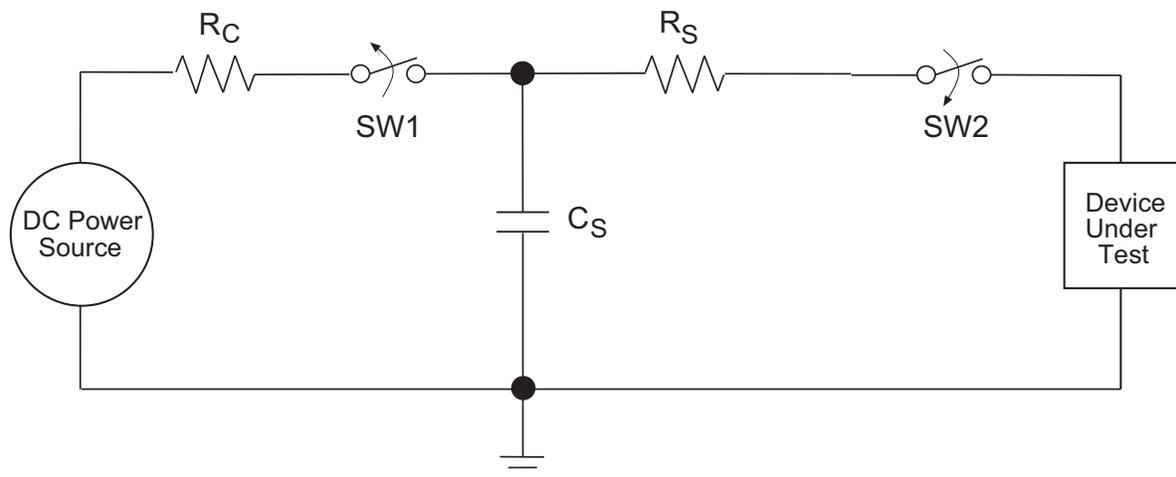
**Figure 12: ESD Test Circuit for Human Body Model**
