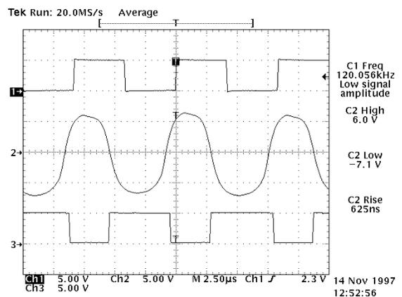
**Figure 5: SP208E Transmitter Output @ 240kbps**
