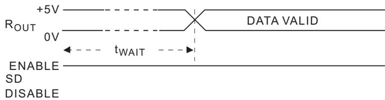
POWER UP WITH SD DISABLED (Charge pump in active mode)
