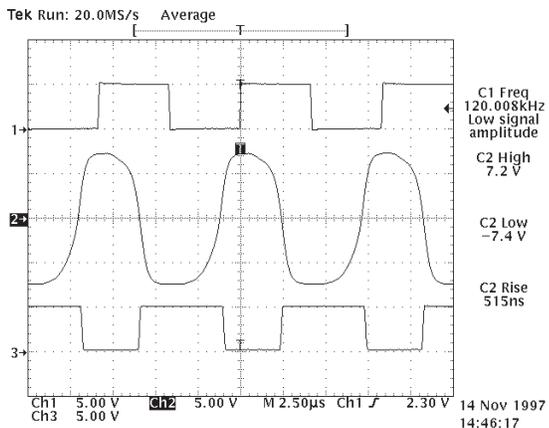
**Figure 4: SP208E Transmitter Output @ 240kbps**
