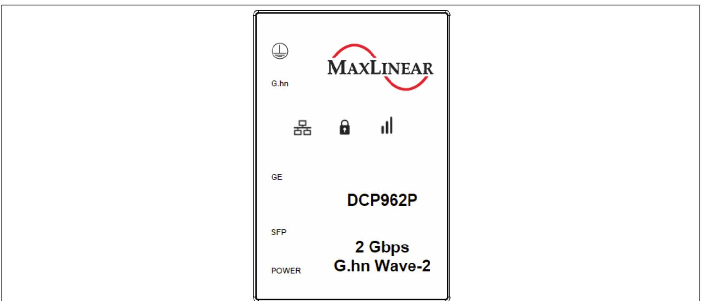
**Figure 7: Front Panel of the DCP962P Adapter**
