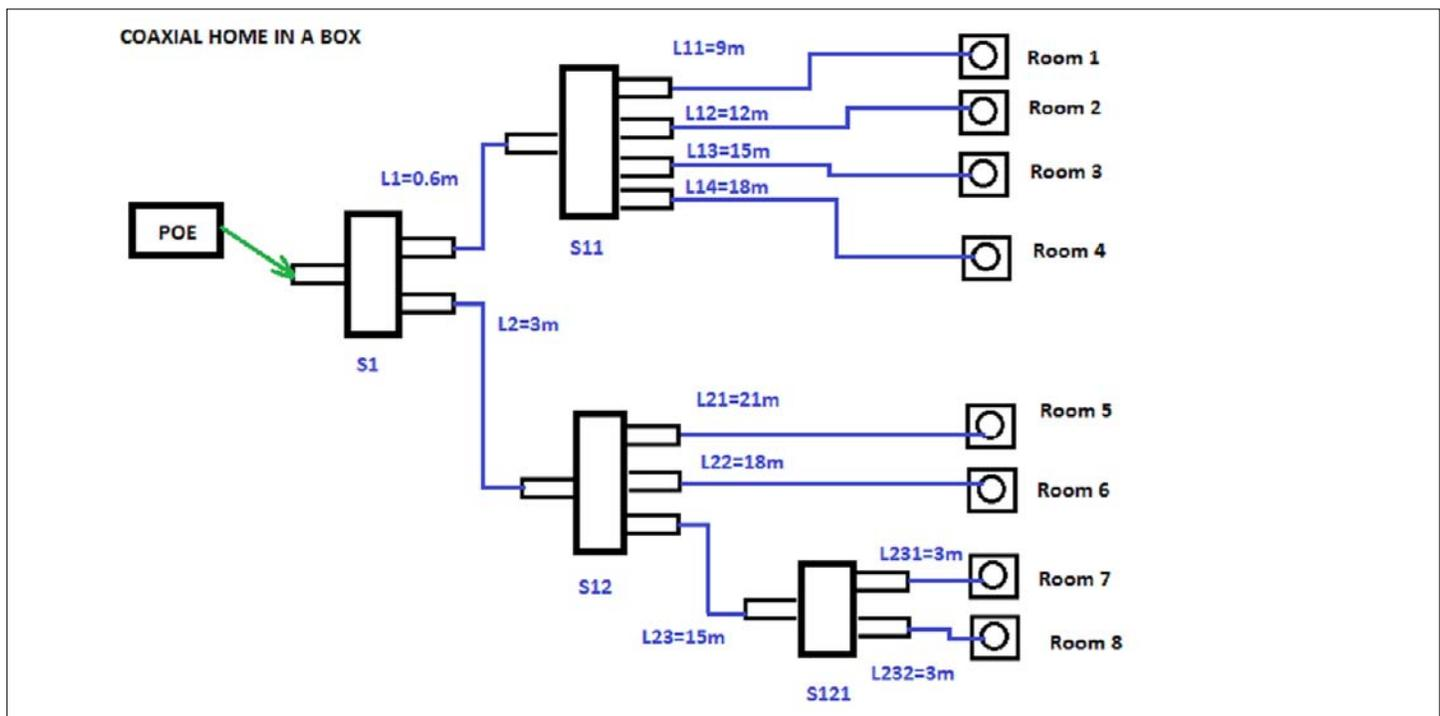
**Figure 8:** Coax "Home In A Box" Test Bench
