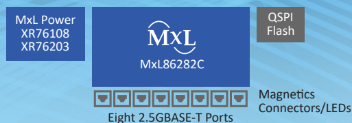
Switch without uplinks
