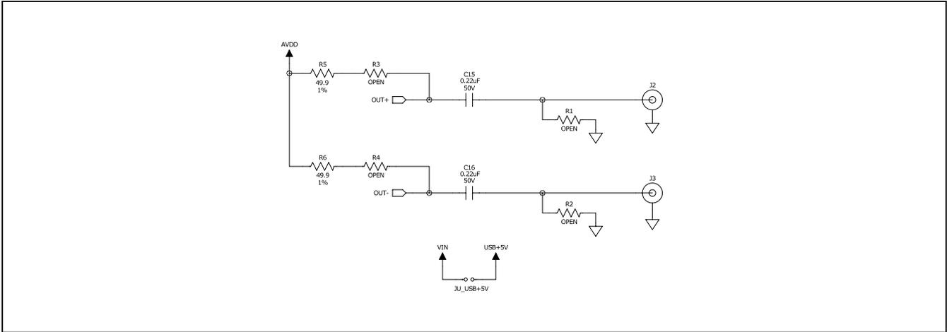
Figure 10c. MAX9271 Coax EV Kit Schematic (Sheet 3 of 3)
