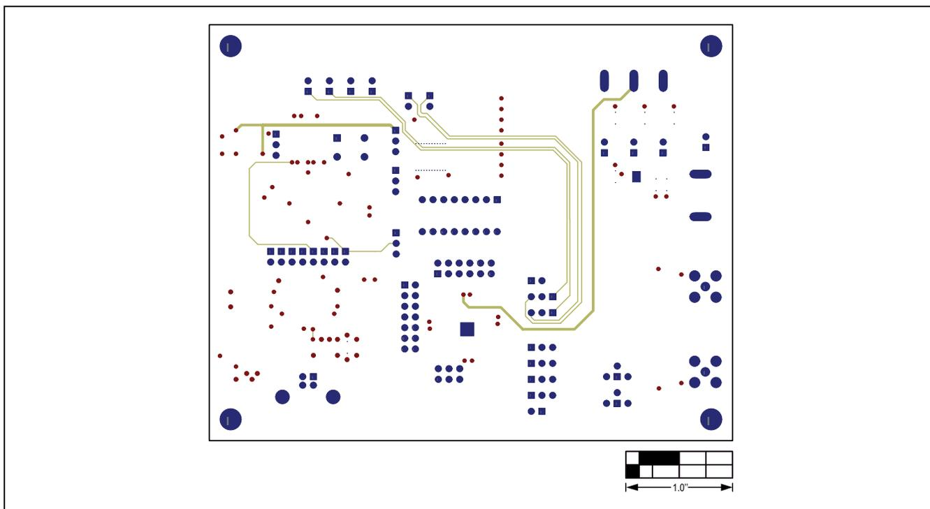
Figure 15. MAX9271 Coax EV Kit PCB Layout—Solder Side
