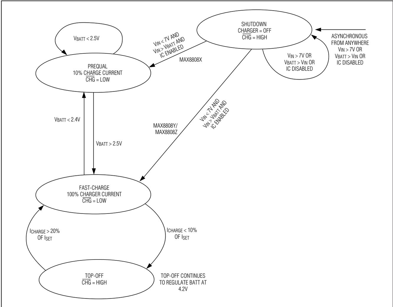
Figure 2. Charge-State Diagram
